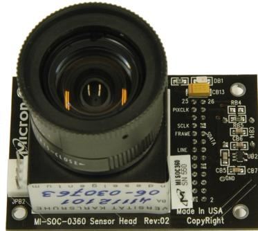
Figure 8.2: Sensor Exploration Module: a Micron MISOC-360 module. It has a CMOS image sensor (MT9V111) with a resolution of 640x480 pixels. The sensor is capable of taking 30 pictures/second.
