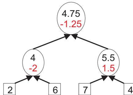
Figure 6.1: Structure graph for the Haar example
