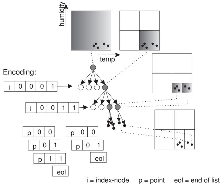
Figure B.2: Representing points with a quadtree
