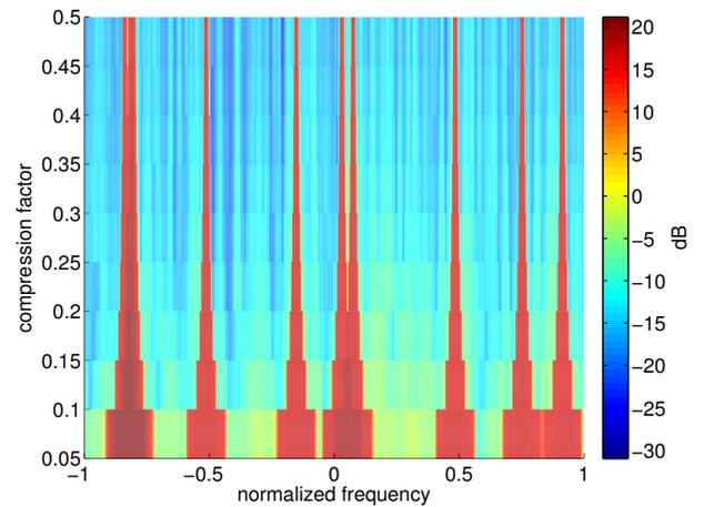
(b) Compression based on a deterministic Zadoff-Chu matrix,  $N = 2000$ . The estimated spectrum is identical to the spectrum in Figure 4(a).
