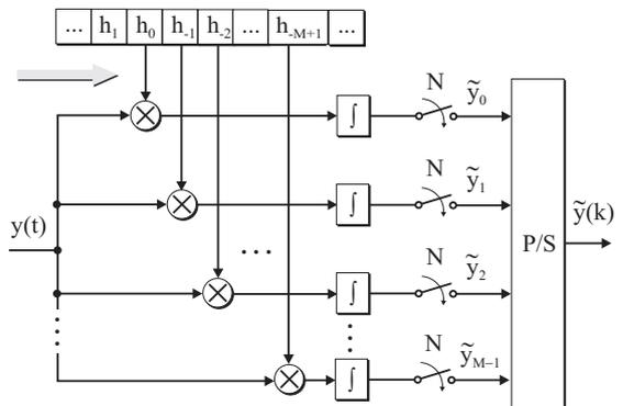
Fig. 1. Proposed time-continuous implementation of time-shifted random preintegration. Integration is reset after  $N$  samples.
