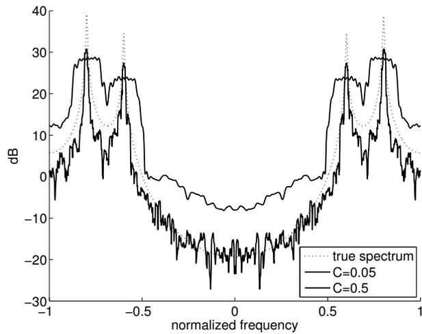
(a) Comparison of true spectrum with compressed estimates for a random Toeplitz compression matrix. The estimated spectrum stems from an autoregressive process with system function  $H(q^{-1}) = 1 - 2.2137q^{-1} + 2.9403q^{-2} - 2.1697q^{-3} + 0.9606q^{-4}$ , which exhibits two prominent peaks.
