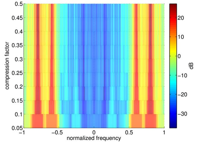
(b) Compression factor versus spectrum estimate. The estimated spectrum is identical to the spectrum in Figure 3(a).
