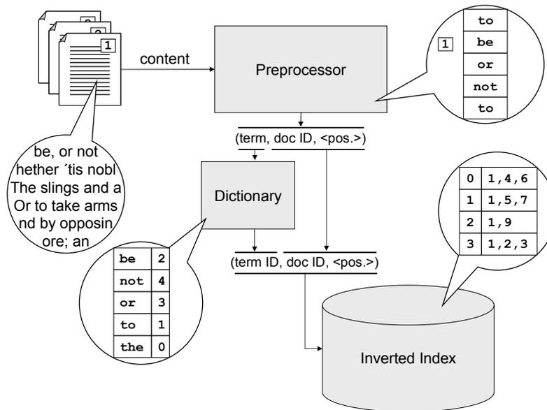
Figure 1.1: Indexing process on an inverted index based search engine
