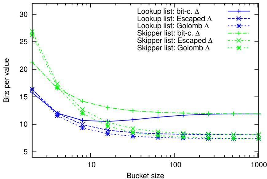
Figure 8.4: Space consumption of different representations on WT2g
