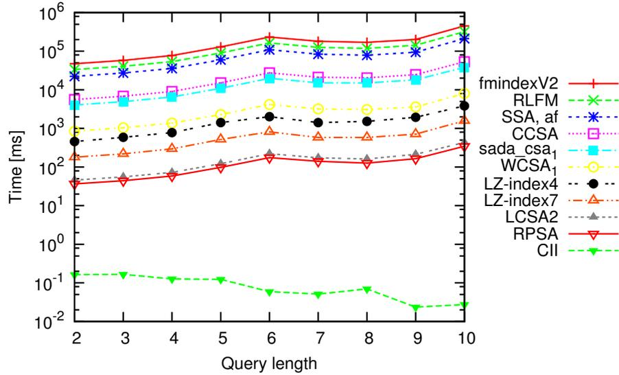
Figure 8.11: Average AND query running times on WT2g\*
