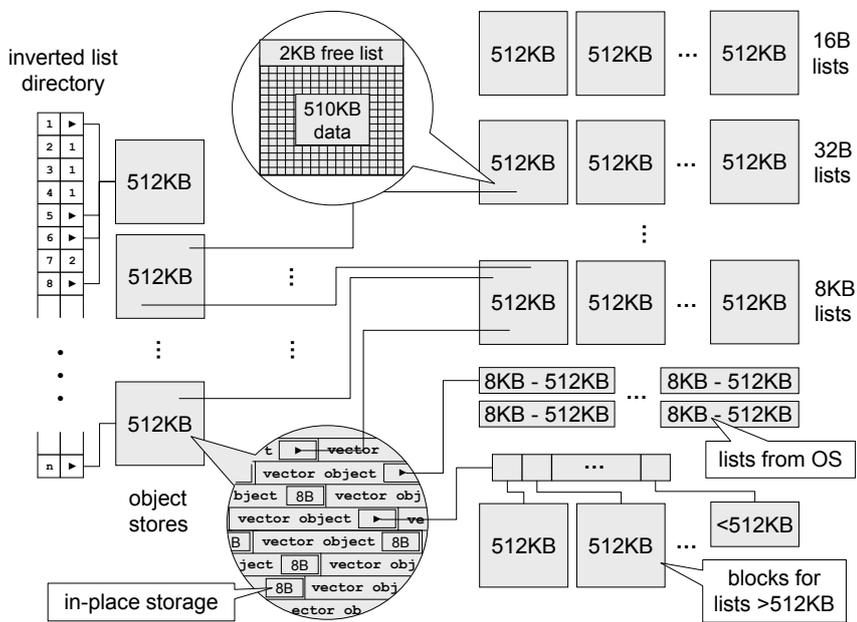
**Figure 4.2:** Organization of inverted list memory during index construction
