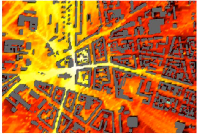
Fig. 3 Typical coverage prediction for 3G communications
