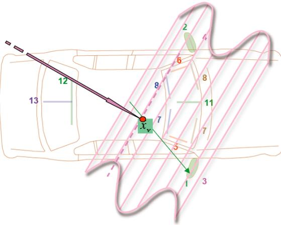
Fig. 6 Extrapolation of a wave from a reference point to one antenna
