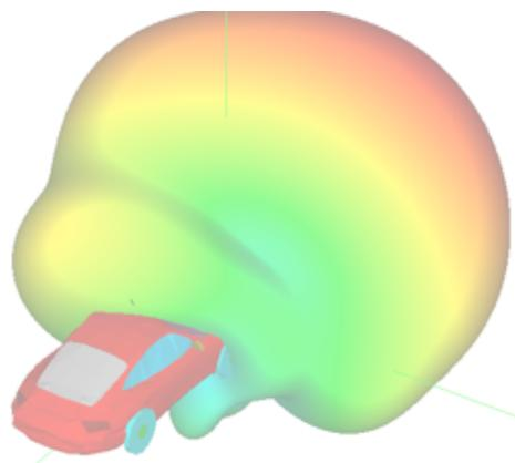
Fig. 1 Example of a car integrated 3D antenna characteristic
