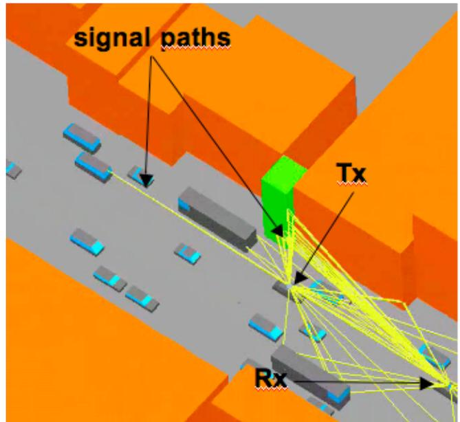
Fig. 4 Ray-tracing in a virtual scenario, here C2C communications
