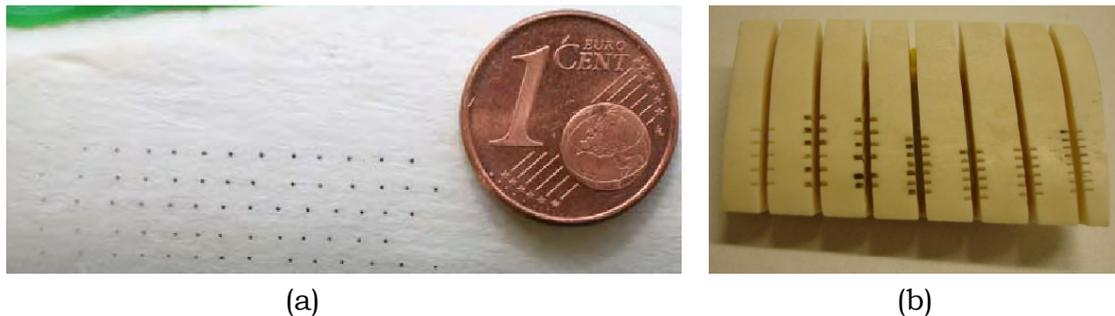
Figure 4.18: Bony specimen for determining the depth development in dependency of the applied number of laser pulses. (a) Ablation craters produced by single laser pulses. (b) Precutted bone for evaluation under a digital microscope.
