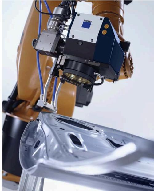
Figure 2.9: Remote laser welding with a robot positioning a three-dimensional scanning device relative to a workpiece. (Picture: TRUMPF GmbH + Co. KG.)
