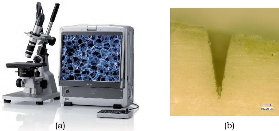
Figure 4.4: Digital microscope (VHX-600, Keyence Corp., Osaka, Japan) and an exemplary microscopic view on a cutting profile of bony specimen.
