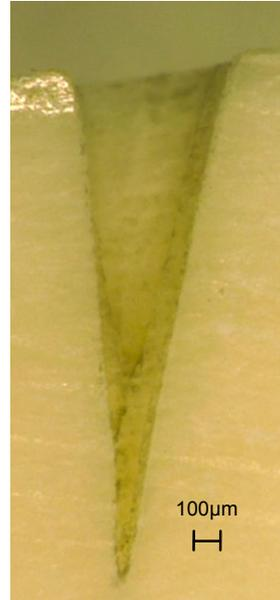
Figure 4.27: Microscopic image of an exemplary wobble cut profile after 80 consecutive lines with focal position at the surface at  $40\ \mu\text{s}$  pulse duration,  $r_{wobble} = 200\ \mu\text{m}$ ,  $v_l = 40\ \text{mm/sec}$ ,  $f_{laser} = 200\ \text{Hz}$  and  $f_{wobble} = 135\ \text{Hz}$ . The cutting depth is  $1896.73\ \mu\text{m}$  and width  $609.54\ \mu\text{m}$ .
