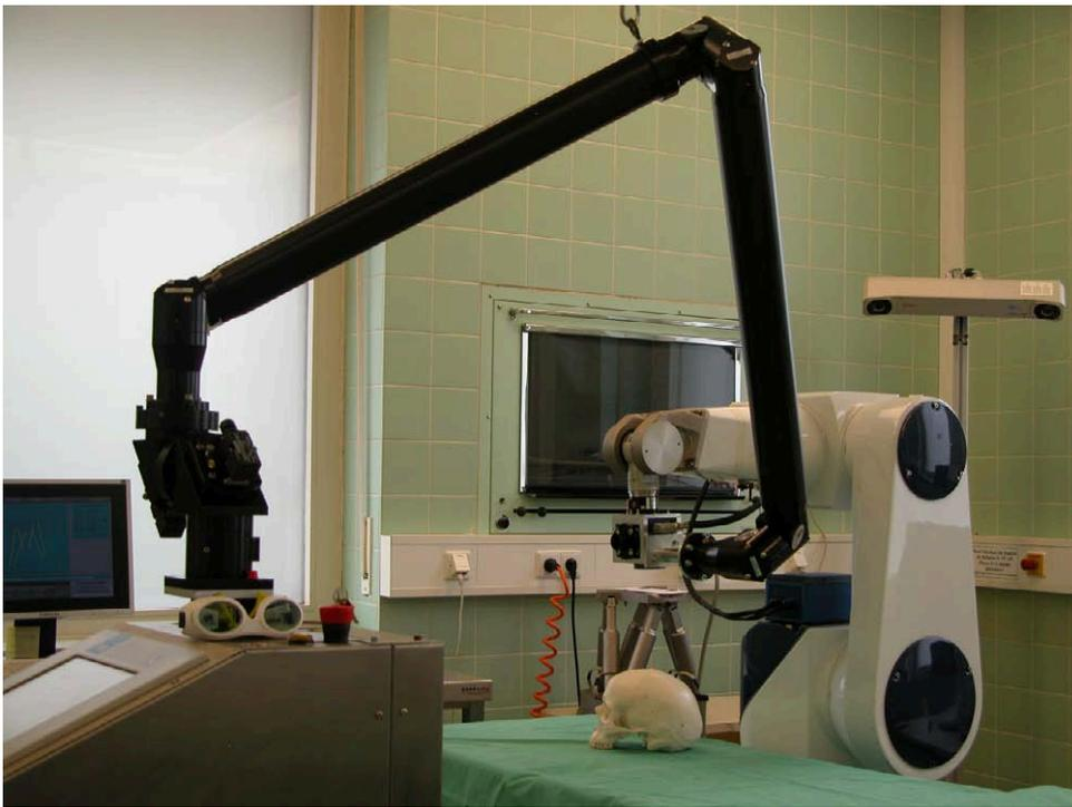
Figure 6.6: The experimental setup for robot assisted laser osteotomy.
