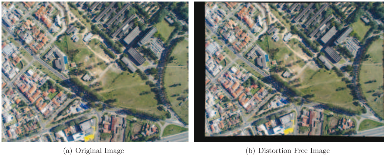
Figure 1.12: Example of the Geometric Image Correction
