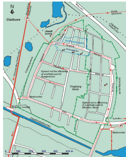
Fig.8: Design proposal with storm water elements. The wadi along the path infiltrate with a great variety, which could have been improved by a second turn in the iterative design process. [Markussen et al. 2004]
