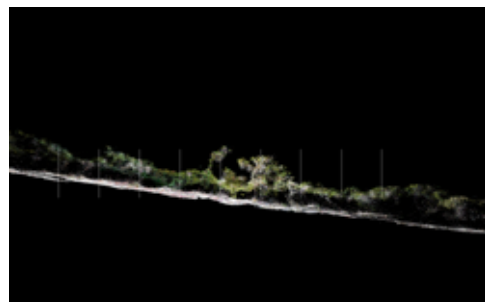
Fig. 9: Before and after the fire. Merged terrestrial laser scans taken before and after a fire on Point Henry. [Ian Weir 2004]
