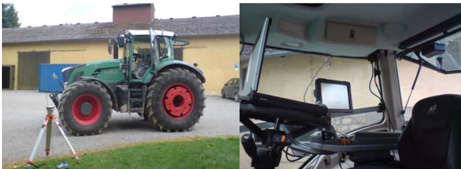
**Figure 1: Fendt 936 Vario tractor and its cabin with Trimble navigation monitor**
