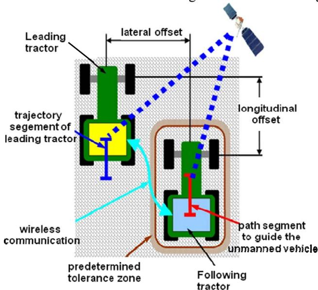
Figure 2: Schematic diagram of the towing bar system for two tractors using GPS navigation and wireless data exchange.
