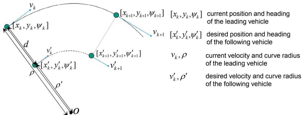
Figure 3: Trajectory of the leading tractor (solid curve) and desired reference course for the following tractor (dashed curve)
