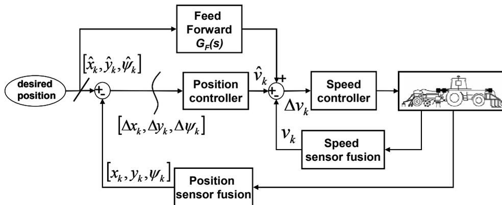
Figure 4: Structure of the cascade controller with feed-forward control for the following vehicle speed.
