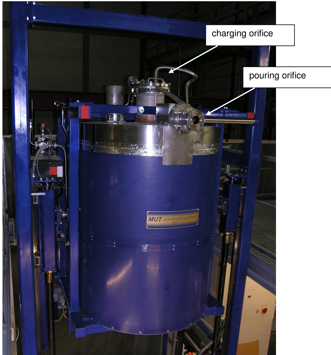
Figure 4: Heating furnace for melt generation.
