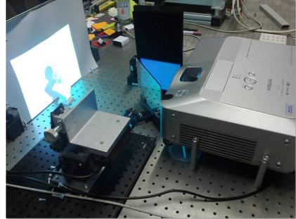
(a) Schematic of a coaxial projector-camera system
