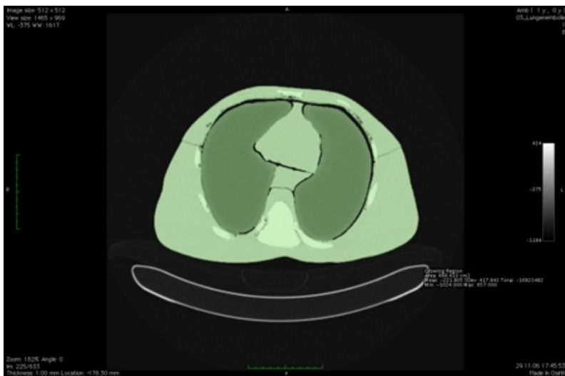
Figure 4.14: A ROI (green coloration) marks all non-air voxel of the phantom slice #225. Figure 4.15 represents the histogram of this ROI.
