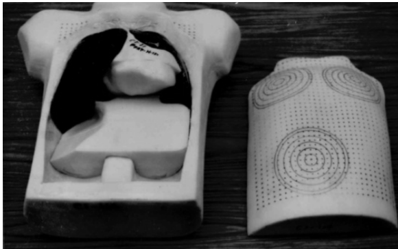
Figure 4.9: Partly disassembled LLNL Torso Phantom (Hickman, 2005).
