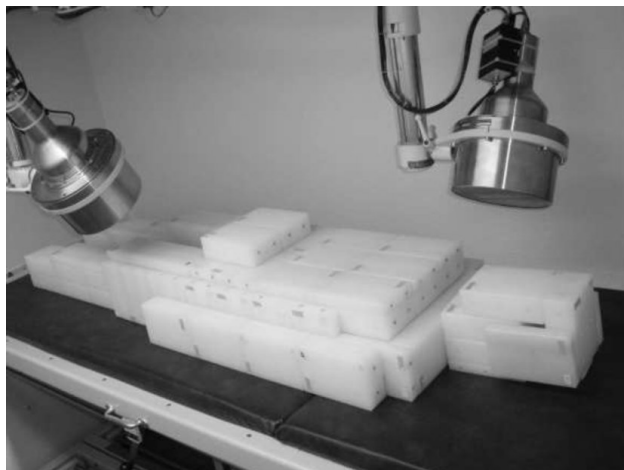
Figure 5.1: The IGOR P 4 phantom in the WBC. VRML representation of the model of IGOR P 4 in the WBC with particles tracks computed from PTRAC data extracted by Voxel2MCNP.
