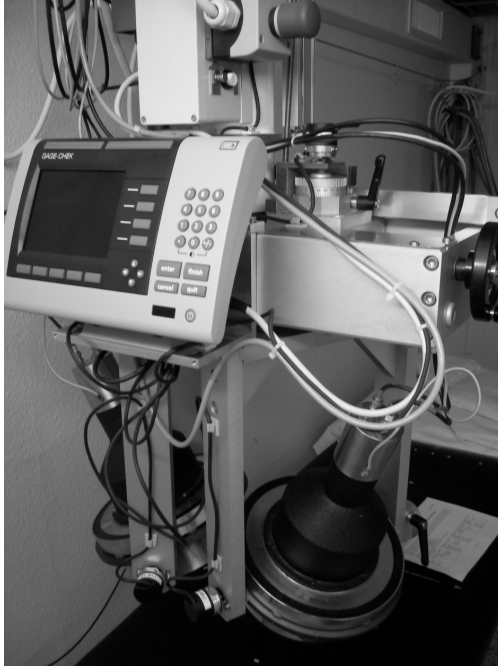
Figure 6.24: Gage Chek display mounted on the phoswich rack in the partial body counter chamber.
