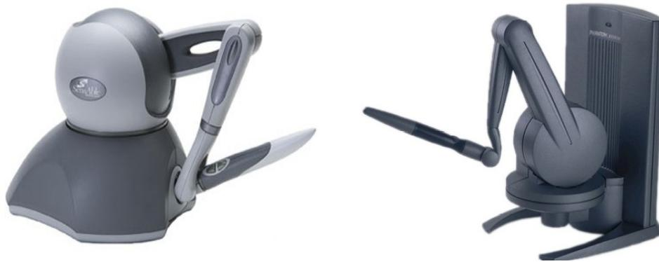
FIGURE 38: TWO TYPES OF HAPTIC INTERFACES: OMNI (LEFT) AND PHANTOM<sup>™</sup> DESKTOP (RIGHT). COURTESY SENSABLE TECHNOLOGIES
