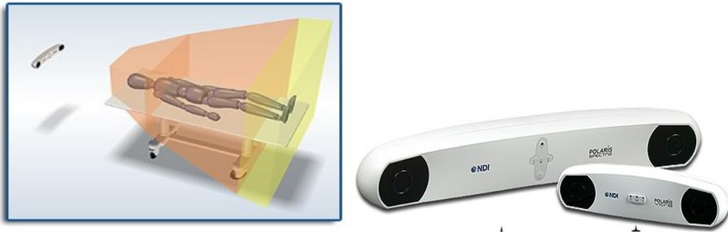
FIGURE 29: TRACKING VOLUME (LEFT) AND NDI VICRA AND SPECTRA SYSTEMS FOR MEDICAL TRACKING (RIGHT).
