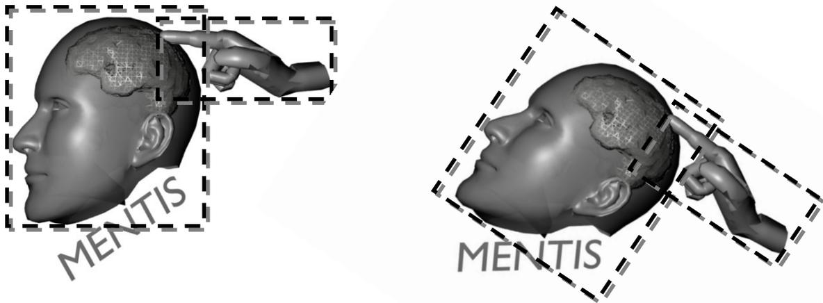
FIGURE 53: OOB STRATEGY. THE INITIAL BOUNDING BOX IS TIGHT FIT AROUND THE MODEL IN LOCAL COORDINATE SPACE AND THEN TRANSLATED AND ROTATED WITH THE MODEL.
