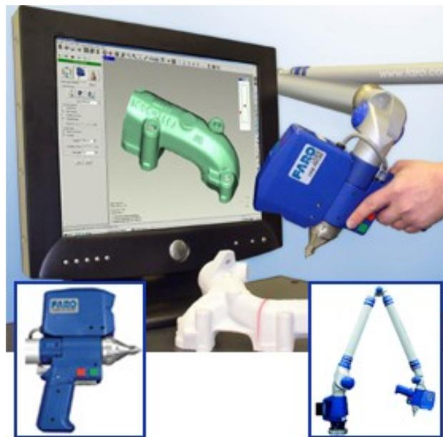
FIGURE 34: 3D SCANNING FOR REVERSE ENGINEERING (FARO ARM)
