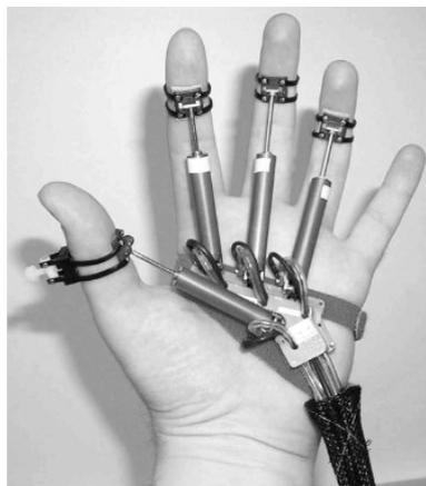
**FIGURE 37: EXAMPLE OF FORCE-FEEDBACK GLOVE WITH PNEUMATIC PISTONS TO SIMULATE GRASPING (HUMAN-MACHINE INTERFACE LABORATORY OF RUTGERS UNIVERSITY)**
