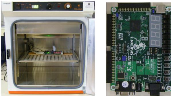
(a) Experimental setup in the thermal chamber (b) Spartan 3 board
