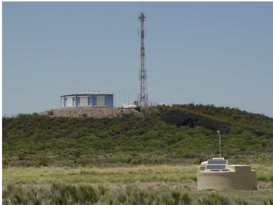
Figure 2.2: One unit of each of the two detector components of the Pierre Auger Observatory: A water Cherenkov detector station of the surface detector in the foreground and a Fluorescence Detector building containing six telescopes behind. Communication of the surface detectors with the central data acquisition works wireless and with the Fluorescence Detector buildings as relay stations, using the communications tower next to the building.
