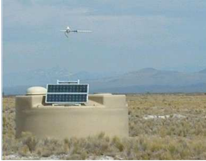
Figure 2.4: A Surface Detector station of the Pierre Auger observatory consisting of water tank, liner, PMTs, electronics, communications and power supply through solar panel and battery. Detailed description of the components is given in the text.
