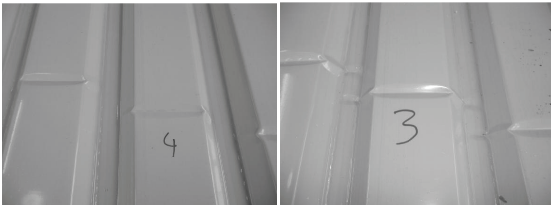
Figure 7: Upper and lower flange of the specimens after failure: trapezoidal sheeting with elastic foundation (left) and sandwich panel (right)
