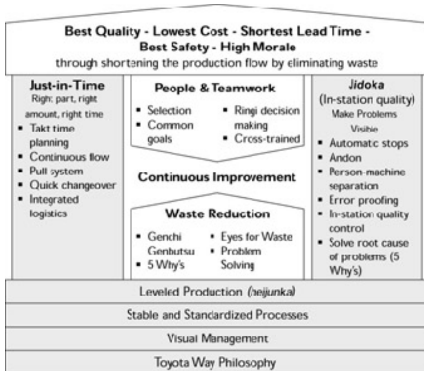
Figure 2-2 House Diagram of The Toyota Production System [LICKER '04]
