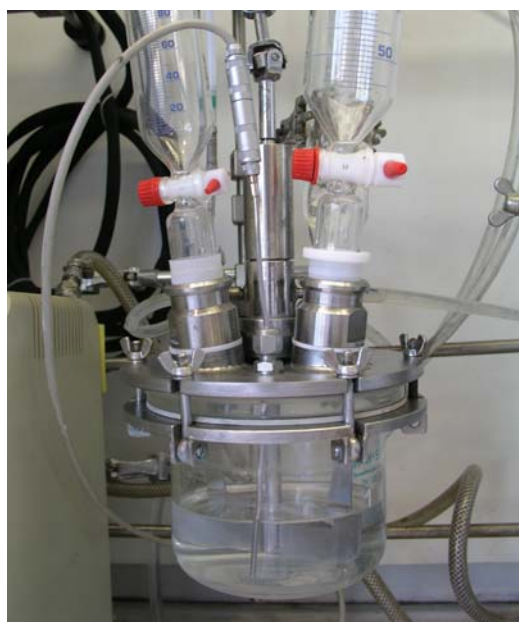
Figure 7-1: reactor used for the synthesis of polyanions, polycations and IPEC
