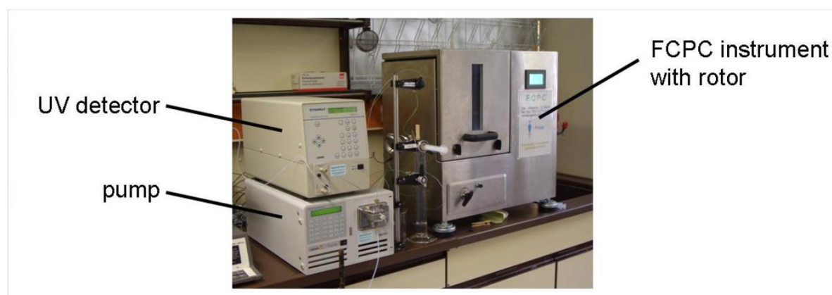
Figure 13: FCPC setup with pump and detector (left-hand side) and FCPC device (right-hand side)
