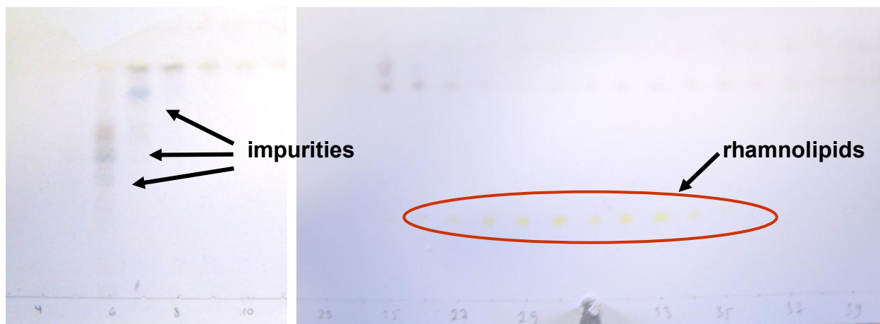
Figure 29: Result of second FCPC purification run, left: elution of impurities, right: elution of rhamnolipid
