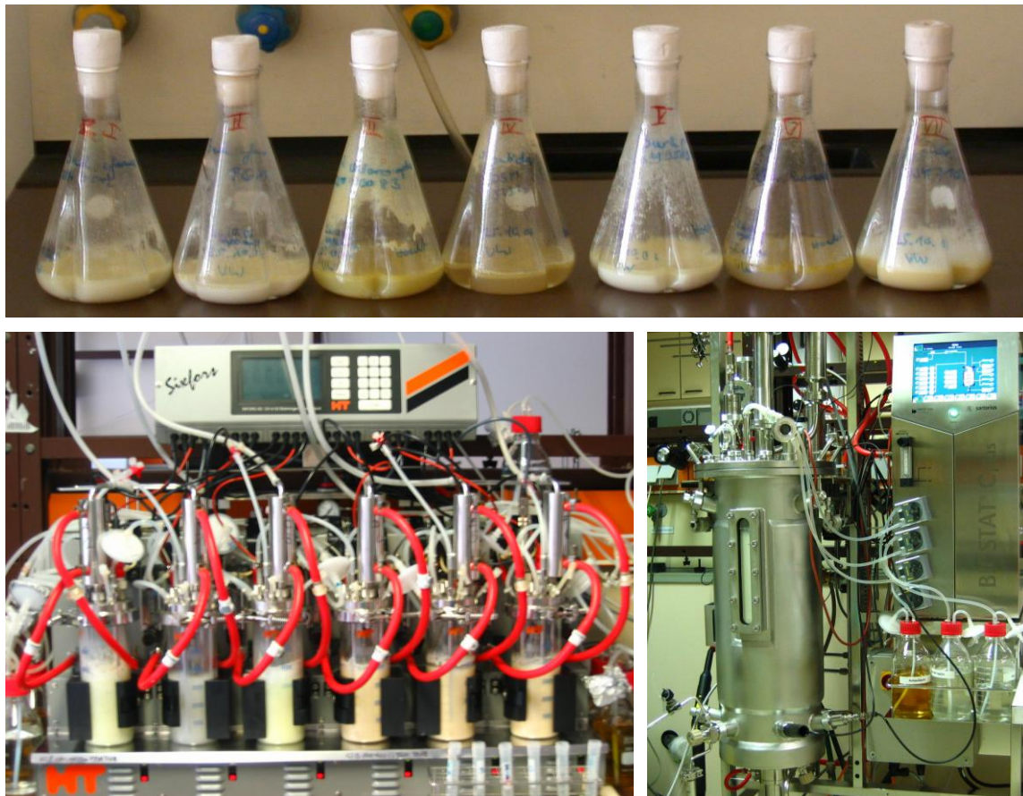
Figure 9: Applied cultivation systems, top: 500 mL shake flasks, bottom left: 0,6 L 6-fold parallel bioreactor system, bottom right: 40 L bioreactor
