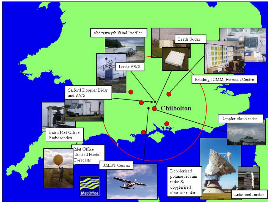
Figure 4.1: Map showing locations of instruments deployed in southern Britain during CSIP. Positions of the radiosonde stations (red circles), from left to right; Bath(B), Swanage(S), Larkhill(L), Chilbolton(C), Reading(R), and Preston Farm(P) (Adapted from Browning et al. 2007).
