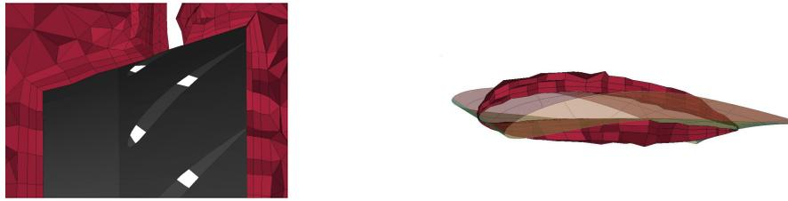
Figure 4.11: Hub and Blade Prism Layers
