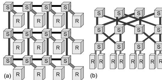
Fig. 1. Presentation of a (a) Mesh and (b) Fat-Tree topologies.  $S$  boxes are switch elements while  $R$  boxes represent a set of logical resources used to implement the tasks.
