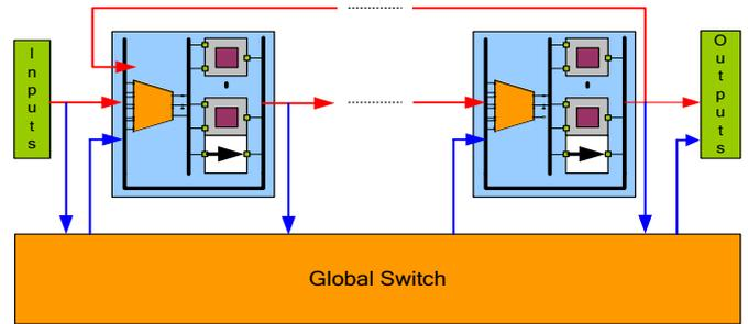
Figure 9: Architecture of the EPLA
