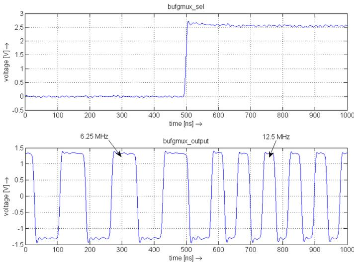
**Fig. 6 BUGMUX clock switching**
