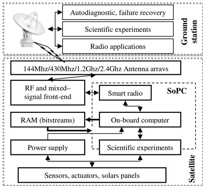
Figure 1. Hardware architecture of the SYRIUS platform.
