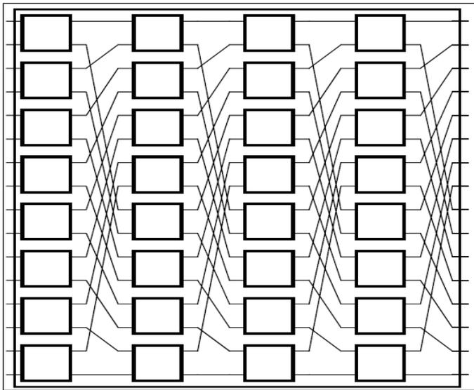
Figure 5: A 16 x 16 Reverse Omega network
