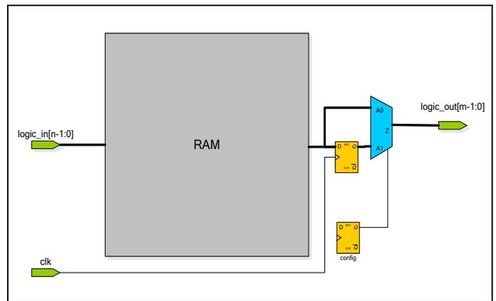
Figure 2: RAM based logic element
