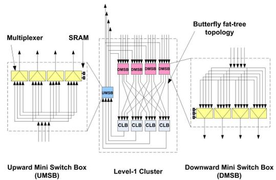
Fig. 4. Detailed Interconnect of Level-1 Cluster of Tree-based FPGA
