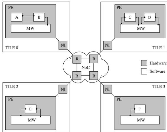
Fig. 2: KPN example mapped on 2x2 mesh NoC platform
