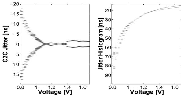
Figure 9. Cycle-to-cycle jitter (left), Jitter histogram (right).
