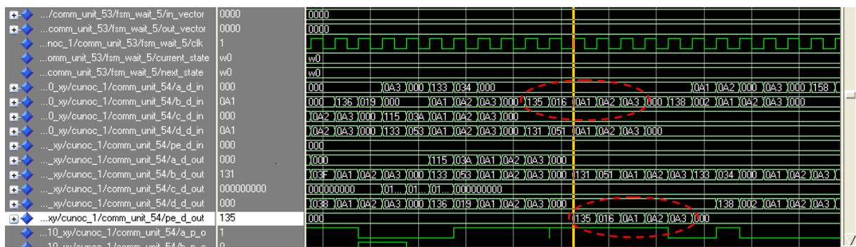
Figure 9. Simulation results of the received data packets in the *PE\_54*.
