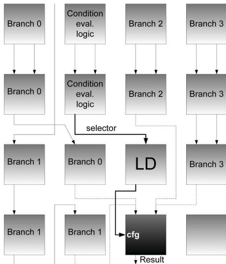
Fig. 1. Implementation of a *switch/case* with four branches.
