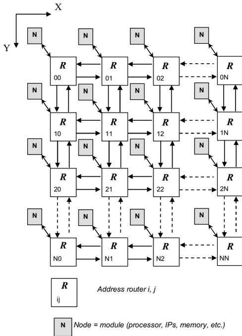
Figure 2. Illustration of the proposed  $n \times n$  Mesh *NoC* model.
