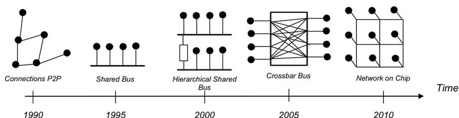
Figure 1. Interconnection evolution in *Systems on Chip*.
