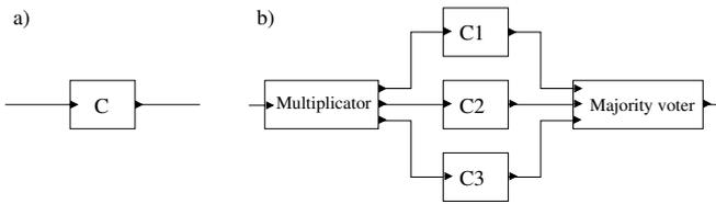
Fig. 7: Semi-concurrent error detection at application level. Component in (a) is replicated by three as shown in (b)
