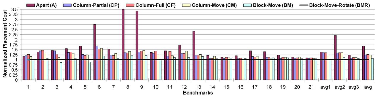
Fig. 7. Placement Cost Normalized to BMR Floor-Planning
