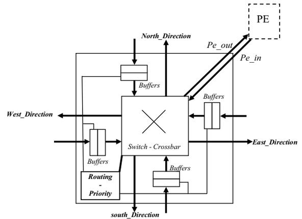
Figure 3. Illustration of the structural architecture of one *NoC* router.
