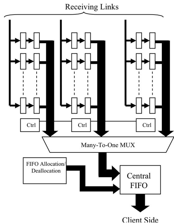
Figure 4: Block Diagram of the New Client Interface.
