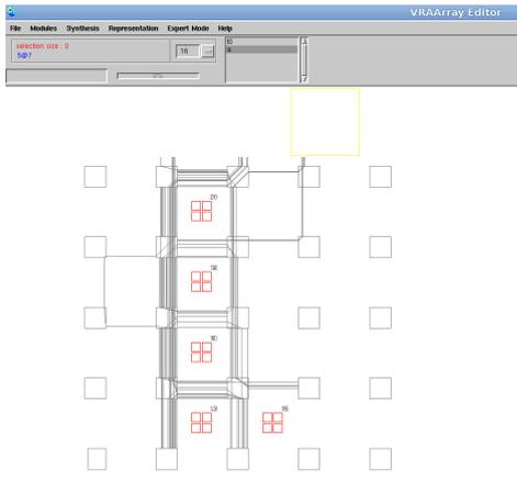
Fig. 9. An application placed and routed over the RFU.
