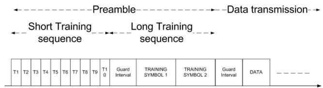
Fig. 4. Data structure of a IEEE 802.11a OFDM preamble
