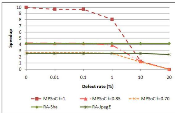
Figure 10. Graceful degradation of *sha* and *jpegE* applications
