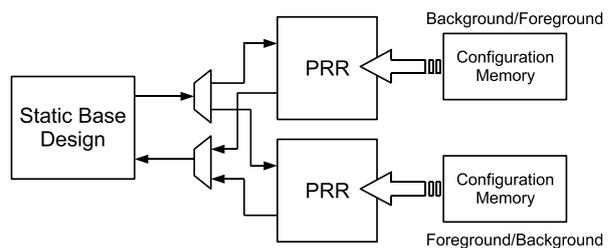
Figure 3. Virtual reconfigurations on single-context FPGAs
