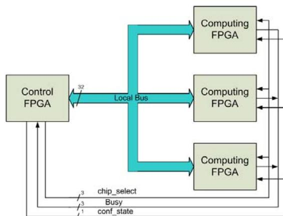
Figure 9. Communication structure during processing mode on a FLC: bidirectional data transfer is only possible via the slower Local Bus (80 MB/s). Separate point-to-point links (*chip\_select* & *busy*) are used for control and synchronization of parallel processing. A further single point-to-point link is connected to all four FPGAs and indicates the current system state, i.e. DAQ or processing mode.
