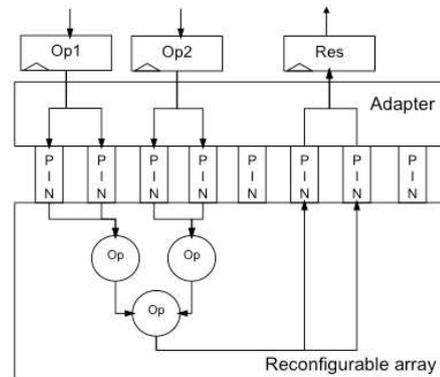
Fig. 3. RFU is interfaced with the processor registers through an adapter.
