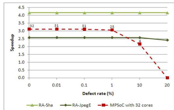
Figure 12. Graceful degradation of 32-cores MPSoC
