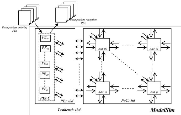
Figure 5. C-VHDL co-simulation in Modelsim environment.
