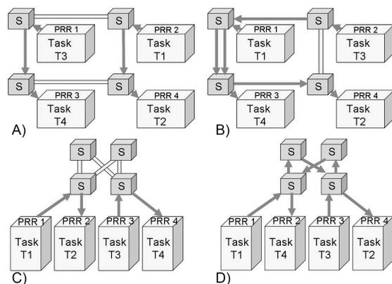
Fig. 2. Mesh (A,B) and Fat-Tree (C,D) topologies interconnecting 4 PRRs. Dynamic tasks  $T1$  and  $T3$  communicate respectively with tasks  $T2$  and  $T4$ .
