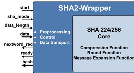
Fig. 5. Schematic overview of hashing submodule
