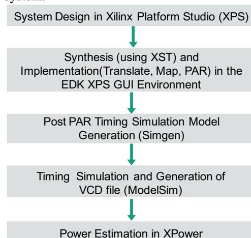
Figure 1. Flow Diagram of the EDK XPower Flow
