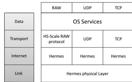
Fig. 2. HS-Scale available communication protocols
