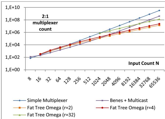
Figure 7: Gate consumption of the Fat Tree Omega network compared to other listed concepts
