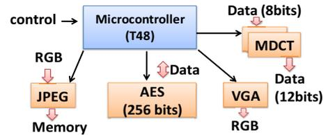
Figure 2. Hardware tasks of the application.
