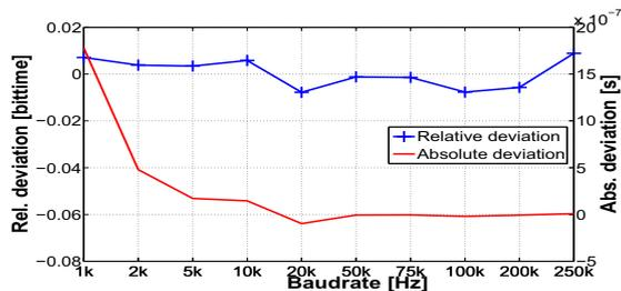
Figure 12. Mean relative/absolute deviation from optimum bit-time.
