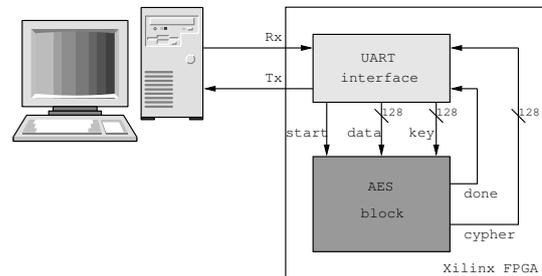
Fig. 6. AES test environment
