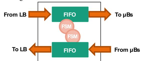
Figure 4. Virtual-IO component
