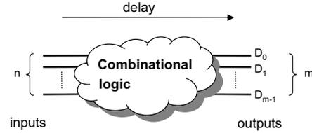
Fig. 8. Propagation delay
