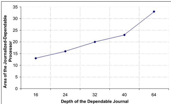
Figure 7. *Effect of Journal Depth on the overall Area*
