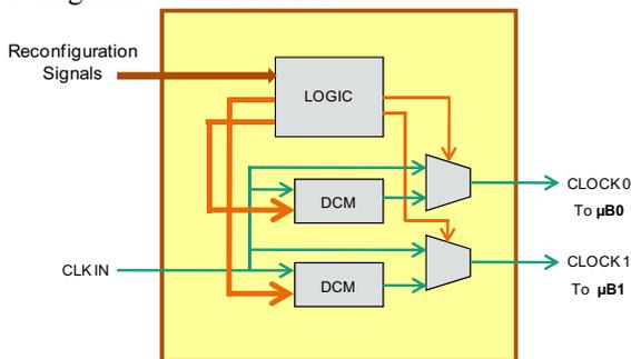
Figure 6. Internal structure of the Reconfigurable Clock Unit
