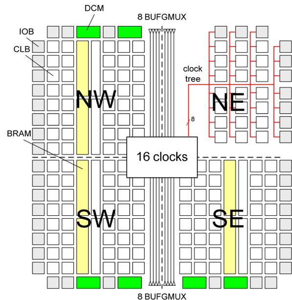
Fig. 2. Xilinx Virtex Clock distribution network
