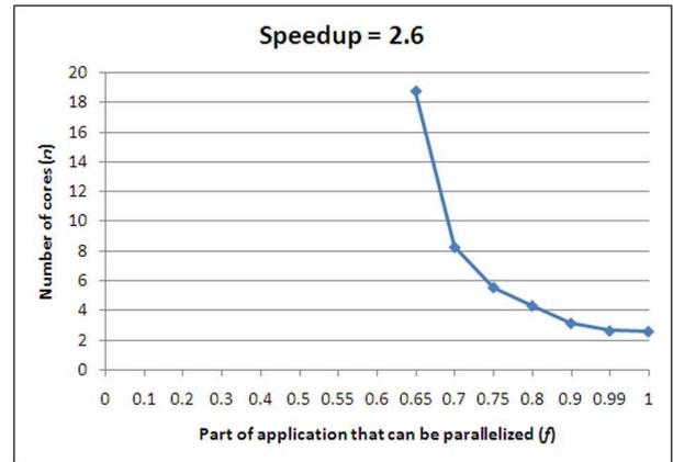
Figure 7. Number of cores as a function of  $f$
