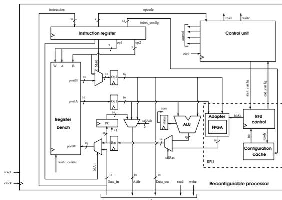
Fig. 2. Schematic of the entire reconfigurable processor.
