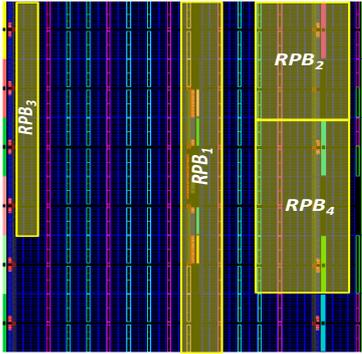
Figure 3. RZ fitting on Virtex 5 SX50.
