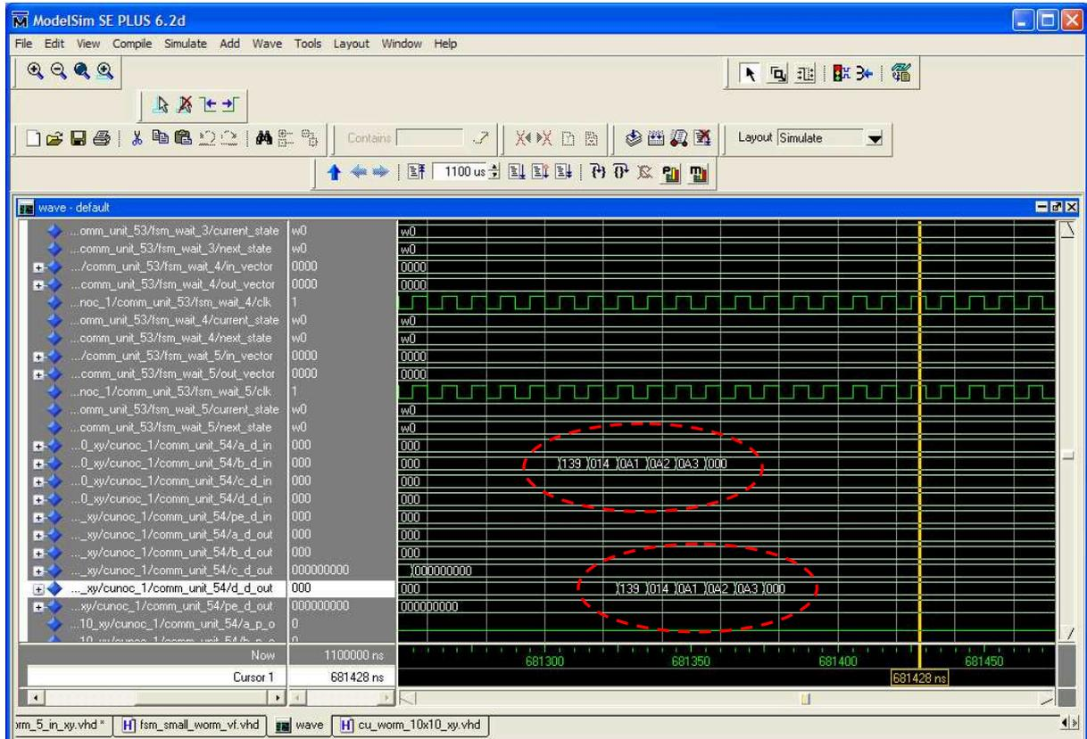
Figure 8. Simulation results of the transmit data packets in the modeled *NoC* based on the *Wormhole* switching and *XY* algorithm.
