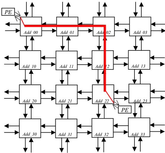
Figure 4. Illustration of the XY routing algorithm.
