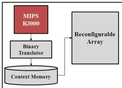
Figure 1. Reconfigurable System
