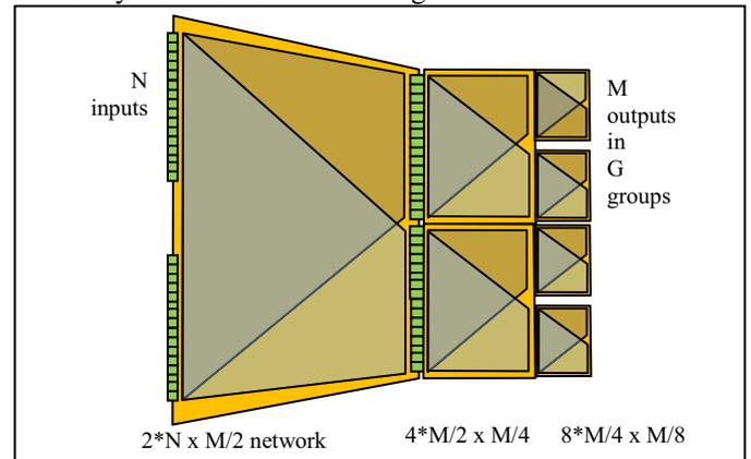
Figure 6: Fat Tree realized with Omega networks for  $r = 2$
