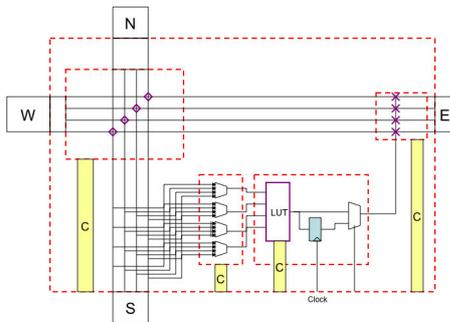
Fig. 6. Structure of a basic cell within the RFU matrix.
