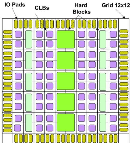
Fig. 1. Mesh-based Heterogeneous FPGA
