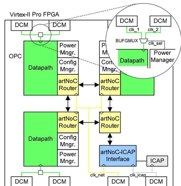
Fig. 4. DodOrg FPGA Floorplan / Clock Architecture
