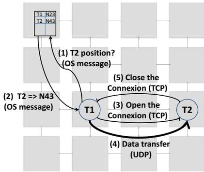
Fig. 3. *Inter-node* task communication protocol
