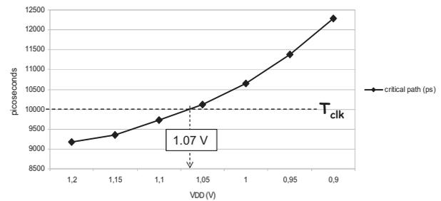
Fig. 14. Fault injection based on power supply decrease
