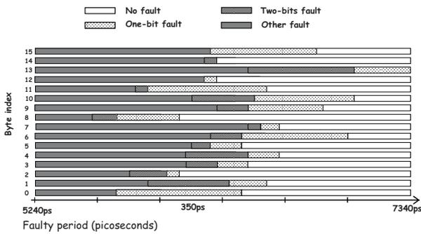
Fig. 12. Fault injection as a function of faulty period duration
