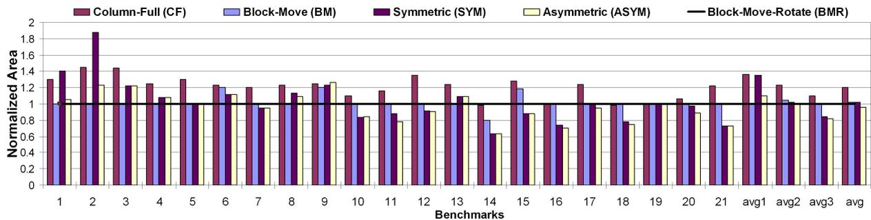
Fig. 9. Area Results Normalized to BMR Floor-Planning
