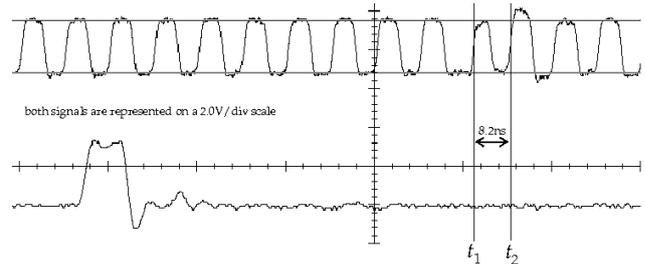
Fig. 10. Faulty clock (uppermost) and trigger signal(lowermost)
