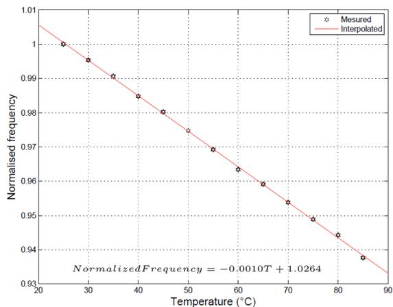
Fig. 8. Normalized Output frequency versus external temperature
