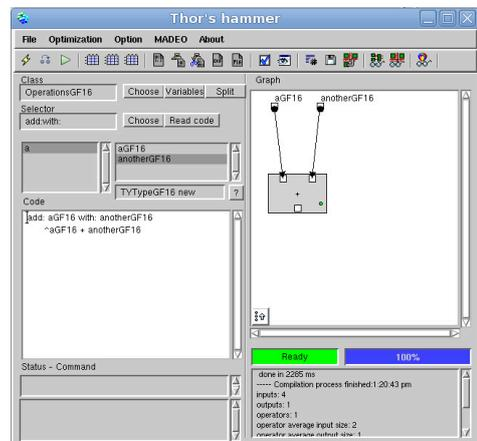
Fig. 8. Specification of a  $GF^{16}$  adder.
