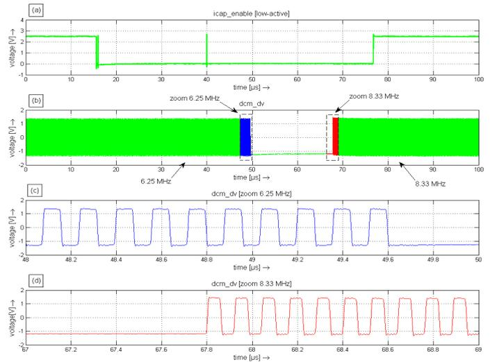
Fig. 5 DCM reconfiguration performance
