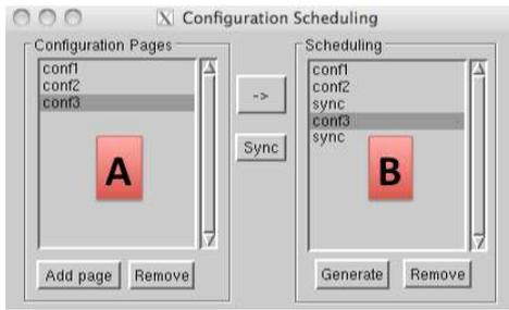
Fig. 4. User interface of the configuration scheduler. Configuration pages (part A) are scheduled (part B) for producing the configuration controller program initialized by a generated testbench.
