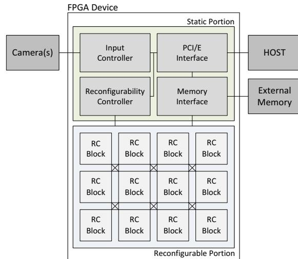
Fig. 1. FPGA Architecture
