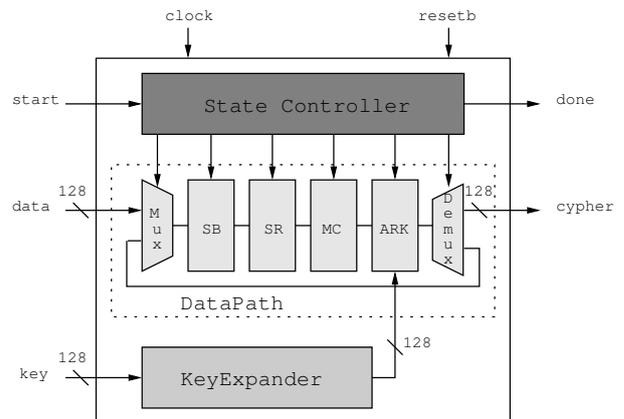
Fig. 5. AES block diagram
