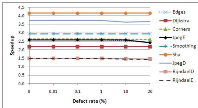
Figure 6. Acceleration degradation of the reconfigurable system
