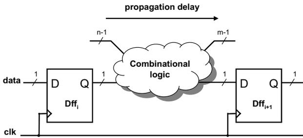
Fig. 7. Internal architecture of Digital ICs
