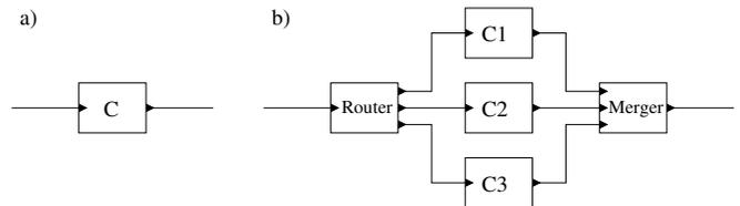
Fig. 8: Adaptation pattern for parallelization. Component in (a) is parallelized by three as shown in (b)
