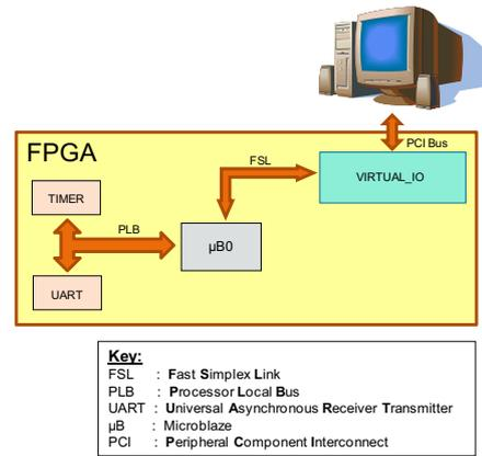
Figure 3. Uni-processor system
