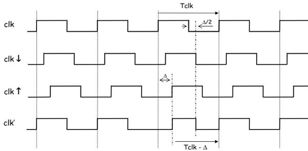
Fig. 9. Faulty clock signal generation
