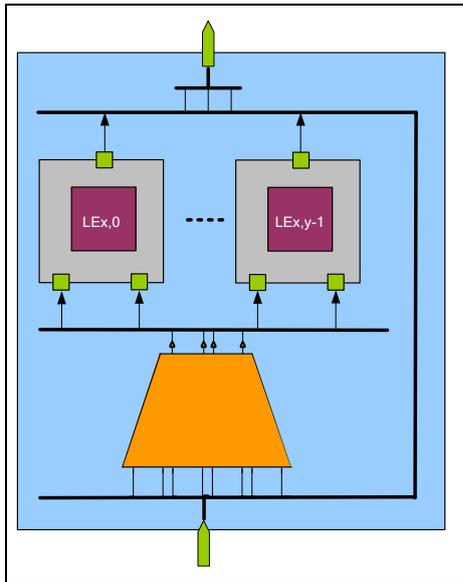
Figure 4: Structure of a LE cluster
