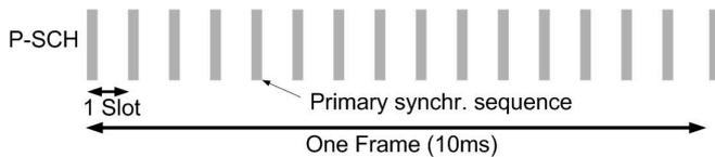
Fig. 3. Data structure of the P-SCH over 1 frame period
