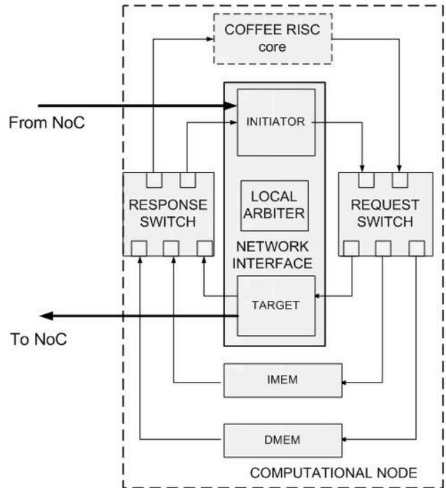
Fig. 2. Detailed view of a Ninesilica node
