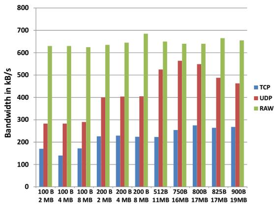
Fig. 5. TCP, UDP and RAW Bandwidth versus packet size and amount of data transferred
