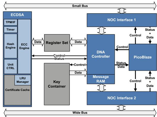
Fig. 6. Wrapping of the signature system for V2X-integration
