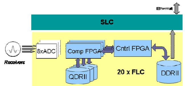
Figure 6. Detailed data-flow on one FLC during the newly created processing mode: As the data sets were previously stored in DDRII memory, they are transferred back to QDRII memory and processed in the computing FPGAs. Finally, the resulting data is stored again in DDRII memory.
