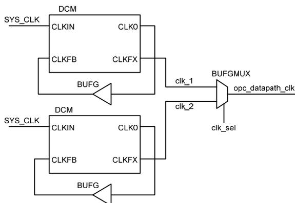
Fig. 3. Example BUFGMUX /DCM configuration
