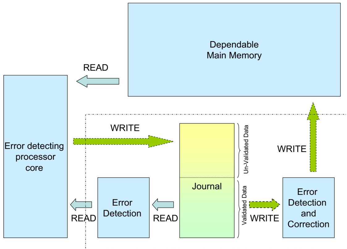
Figure 2. Block Diagram of overall architecture
