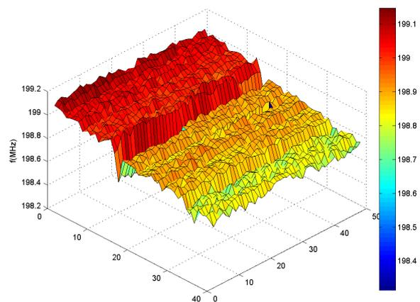
Fig. 9. Oscillator frequency cartography at  $T = 40^{\circ}C$  for Board 3
