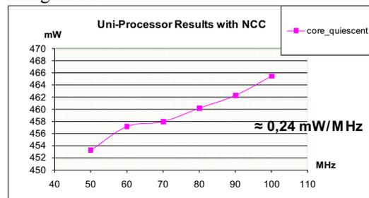
Figure 8. Impact of the clock frequency onto the static power consumption of a uni-processor design.
