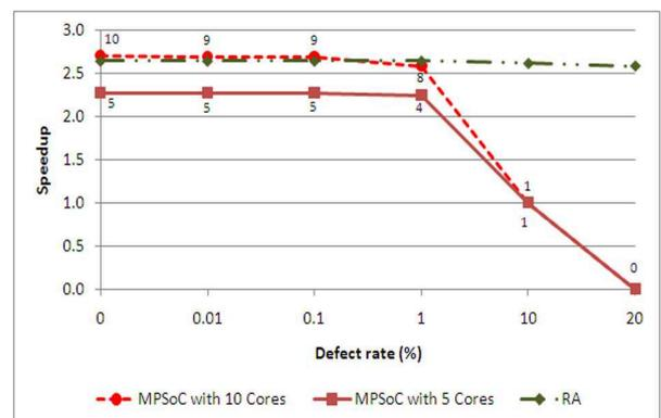
Figure 9. Performance degradation of the MPSoC
