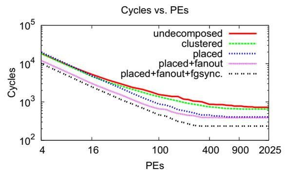
Fig. 12: *Clustering, Placement, Fanout-Routing and Fine-Grained Synchronization*
