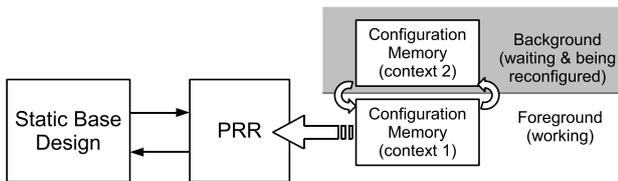
Figure 1. Virtual reconfigurations on multi-context FPGAs
