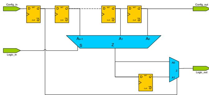
Figure 1: Logic structure of a logic element (LE)
