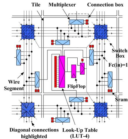
Fig. 2. Detailed Interconnect of a CLB with its Neighboring Channels
