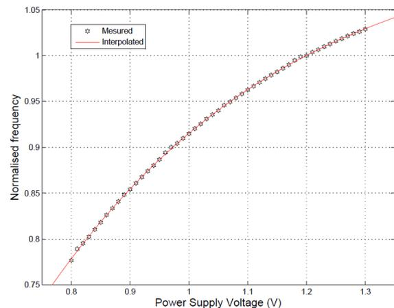
Fig. 7. Normalized Output frequency versus Power Supply Voltage
