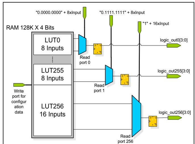
Figure 3: Using multiple read ports to share one RAM between LEs
