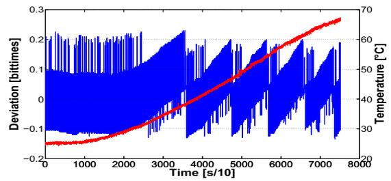
Figure 10. Relative deviation from optimal sending slot and operating temperature.
