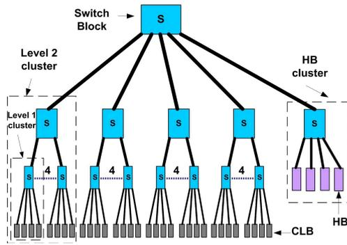
Fig. 3. Tree-based Heterogeneous FPGA
