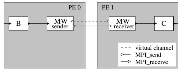
Fig. 3: Middleware details for the connector between B and C
