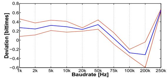
Figure 11. Mean relative deviation from optimal sending point vs. baudrate.
