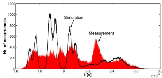
Figure 4. Jitter histogram simulated/measured, 4-bit counter.
