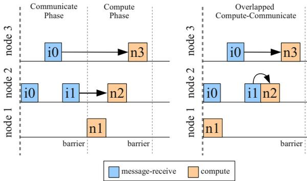
Fig. 6: Fine-Grained Synchronization
