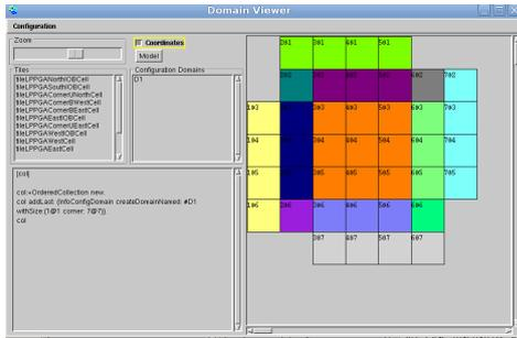
Fig. 5. On the right, view of the different cell types composing the matrix (border cells, middle cells, IO cells). On the left, configuration domains are defined as a set of rectangular boxes. They can be reconfigured independently from each other.
