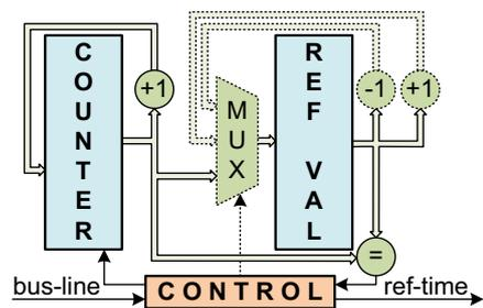
Figure 6. Basic structure of the timer-reference generation circuit.
