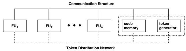
Fig. 1. Abstract Model of an AMIDAR Processor
