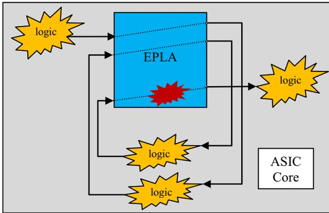
Figure 11: Architecture for variable test and modification point insertion
