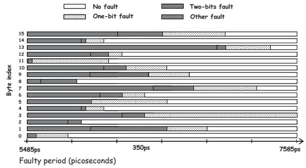
Fig. 13. Fault injection for a different plaintext
