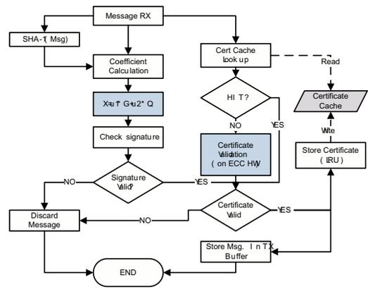
Fig. 4. Procedure for signature verification
