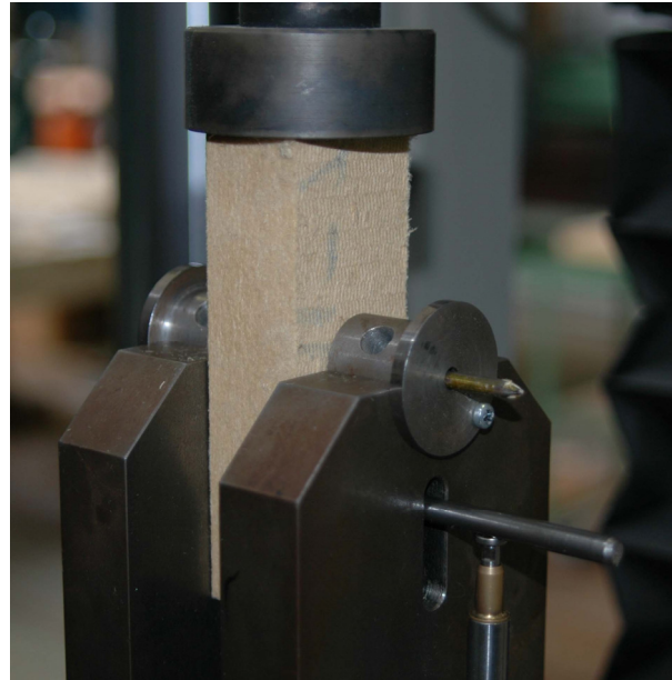
Figure 4: Test - embedding strength of nails in WFIB
