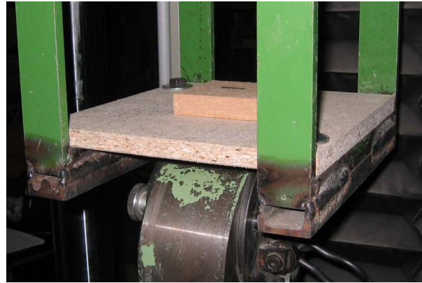
Figure 7: Test – Crown pull-through resistance of wide-crown staples in WFIB
