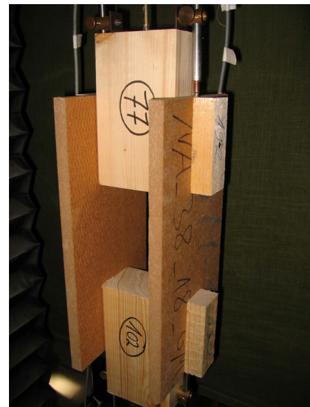
Figure 14: Test specimen for test of timber-WFIB-joints
