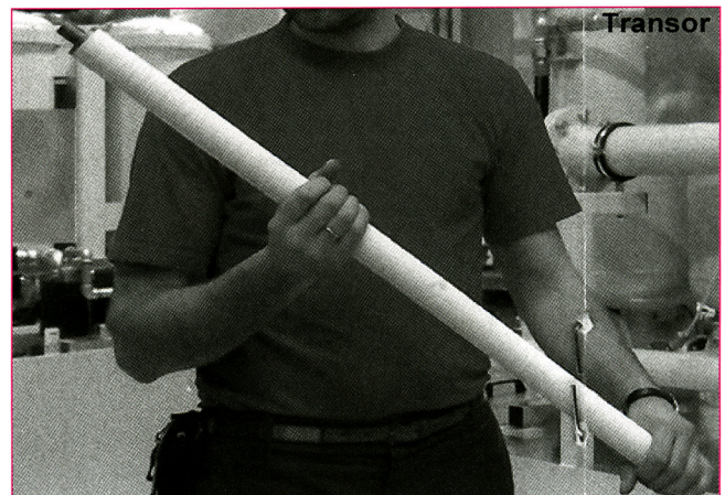
Abb. 2: Papier-Spaltfilterkerze (Transor GmbH)
