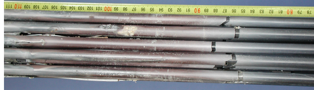
Fig. 38: QUENCH-14; Posttest view of the test bundle at elevations 800-1000 mm (cladding breaches caused by disassembly of test bundle and shroud).
