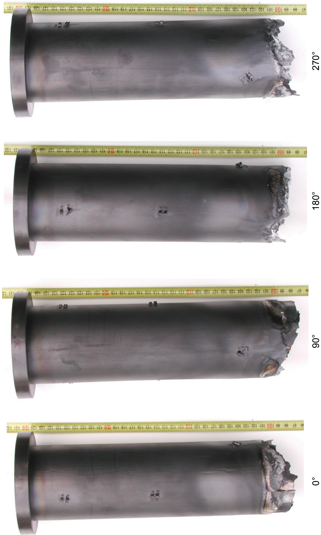
Fig. 42: QUENCH-14; Posttest view of the upper part of the shroud at elevations 1000-1300 mm.
