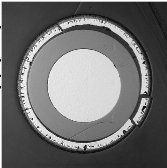
heated rod 19: 5 through going cladding cracks
