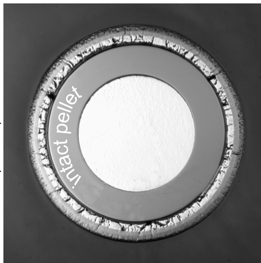
heated rod 3: pre-and post-reflood cracks
