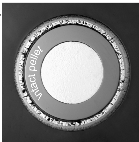
unh. rod 1: steam starvation at necking
