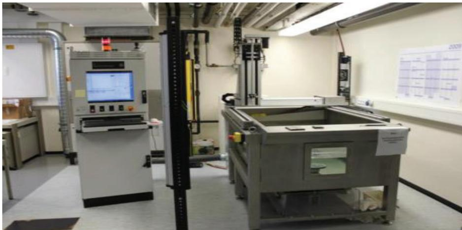
Fig. 15: Immersion testing facility KC-200
