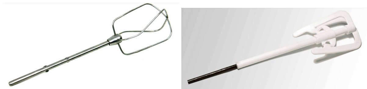
Figure 3-6: Agitator F 520 75 used for dispersing (left) and modified horseshoe mixer used for agglomeration (right).
