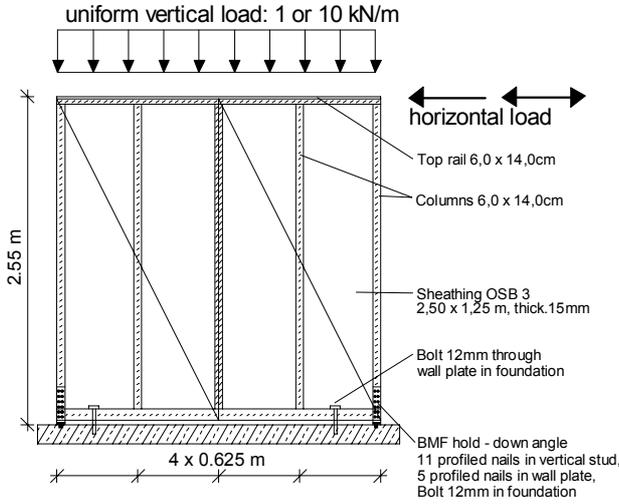
**Figure 10:** Timber Framed Wall Test Specimen
