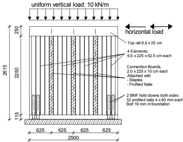
Figure 5: X-lam massive panel Test Wall Specimen
