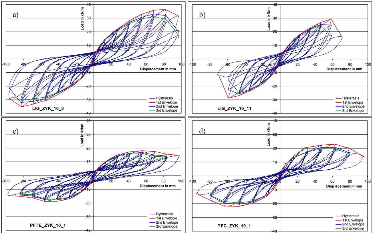
**Figure 11:** Hysteresis for a) X-lam massive panel system connected with staples, b) X-lam massive panel system connected with nails, c) prefabricated timber wall elements, d) timber frame construction
