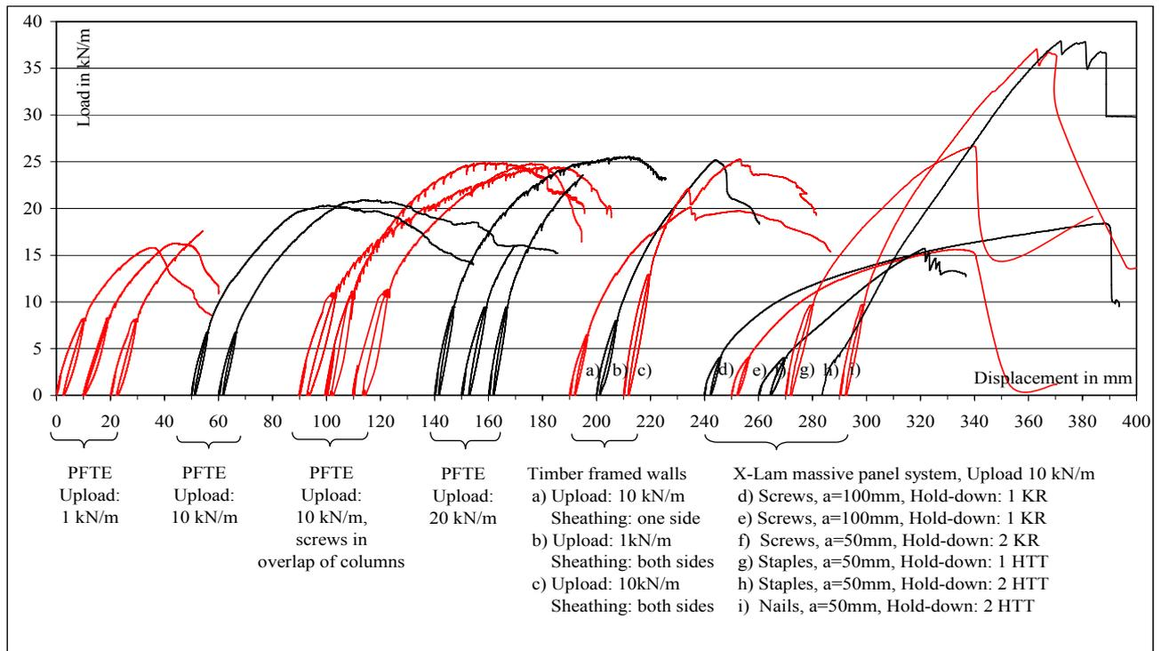
Figure 8: Comparison of the monotonic tests of the different systems
