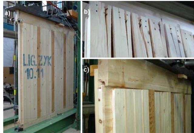
Figure 6: a) X-lam massive panel Test Wall Specimen b) failure due cracking of boards when using nails c) deformed wall (top rail perspective)
