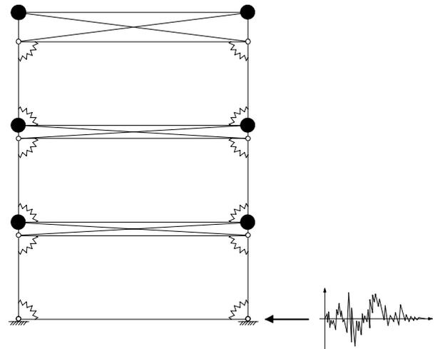
**Figure 12:** Model chosen for the evaluation of behaviour factors
