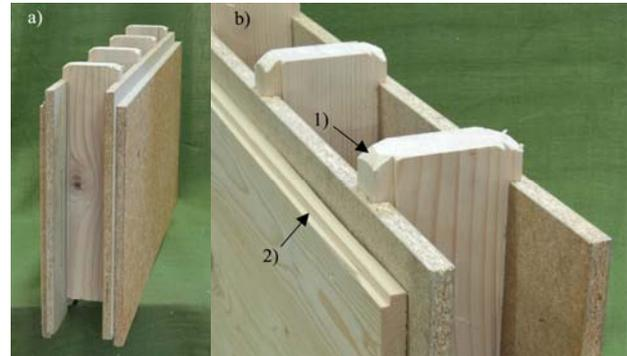
**Figure 3:** a) Prefabricated timber wall element b) Offset of columns (1) and offset of layers (2)
