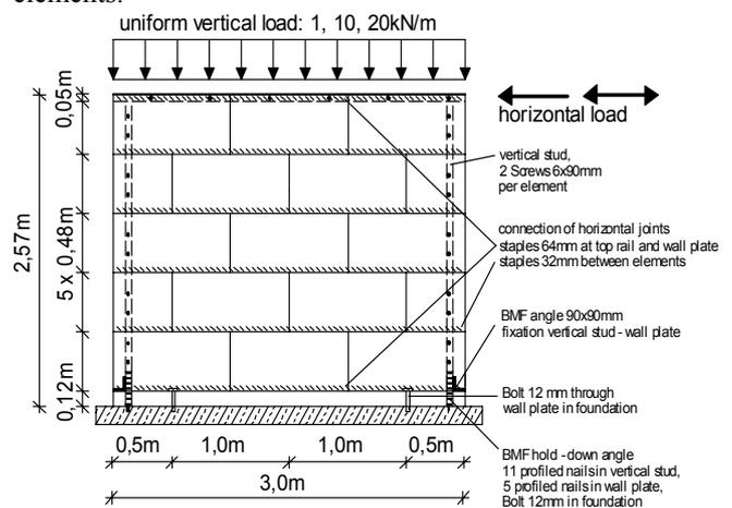
Figure 7: PFTE Test Wall Specimen
