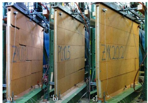
Figure 9: Typical Failures in PFTE Tests
