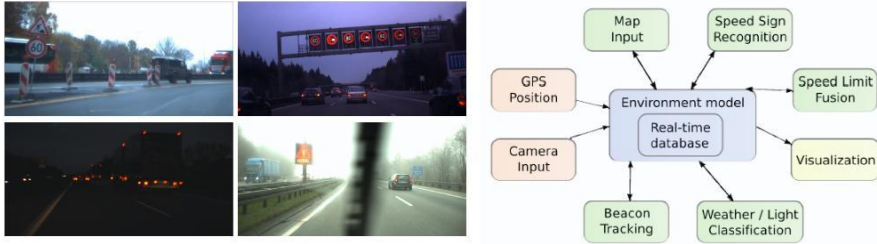
Fig. 1. Vision based system are beneficial in the presence of construction sites and dynamic traffic signs, while digital maps are preferable in bad weather and adverse lighting scenarios. Adapting sensor input reliability in such situations improves fusion results.
