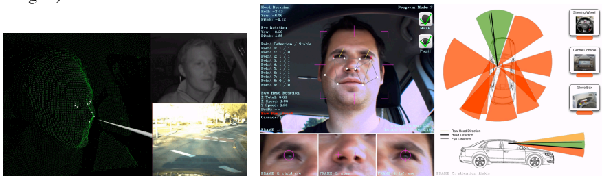
Fig. 4. Headpose estimation based on 3D tof data (left) and appearance based gaze tracking and focus of attention detection (right).
