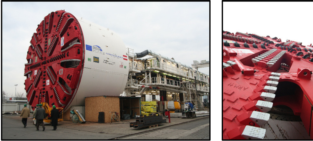
Figure 1.5.: Hard rock tunnel boring machine (TBM) at the Herrenknecht AG headquarter, Schwanau, Germany: 13.3 m diameter TBM build for tunneling the Brenner railroad track Munich - Verona (left picture), detailed view on the TBM cutting wheel (right picture).
