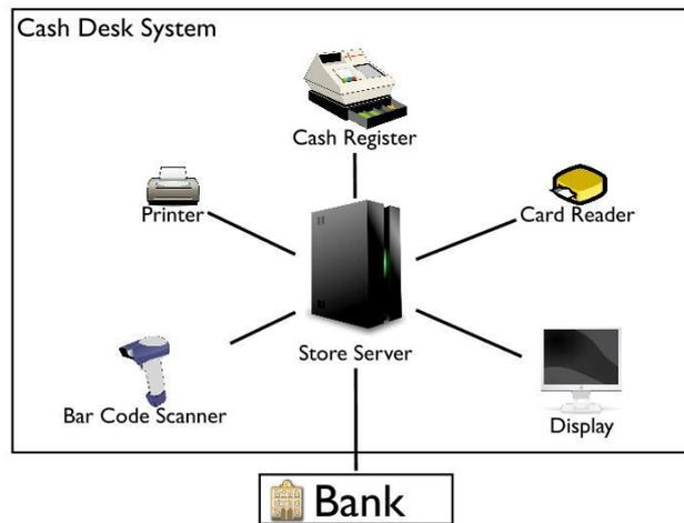
**Fig. 2.** The hardware components of a single cash desk. Image adapted from [3].
