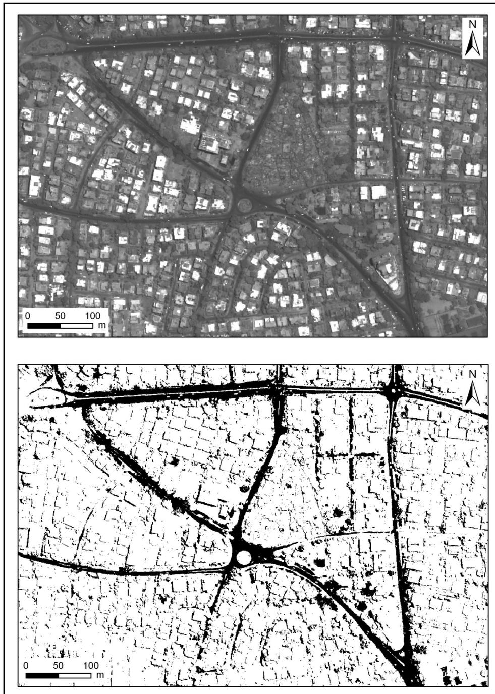
Figure 30: Linear stretch on panchromatic subset. The upper figure shows the original panchromatic image. The lower figure displays the linear stretched image with the data range set to 369 to 414.
