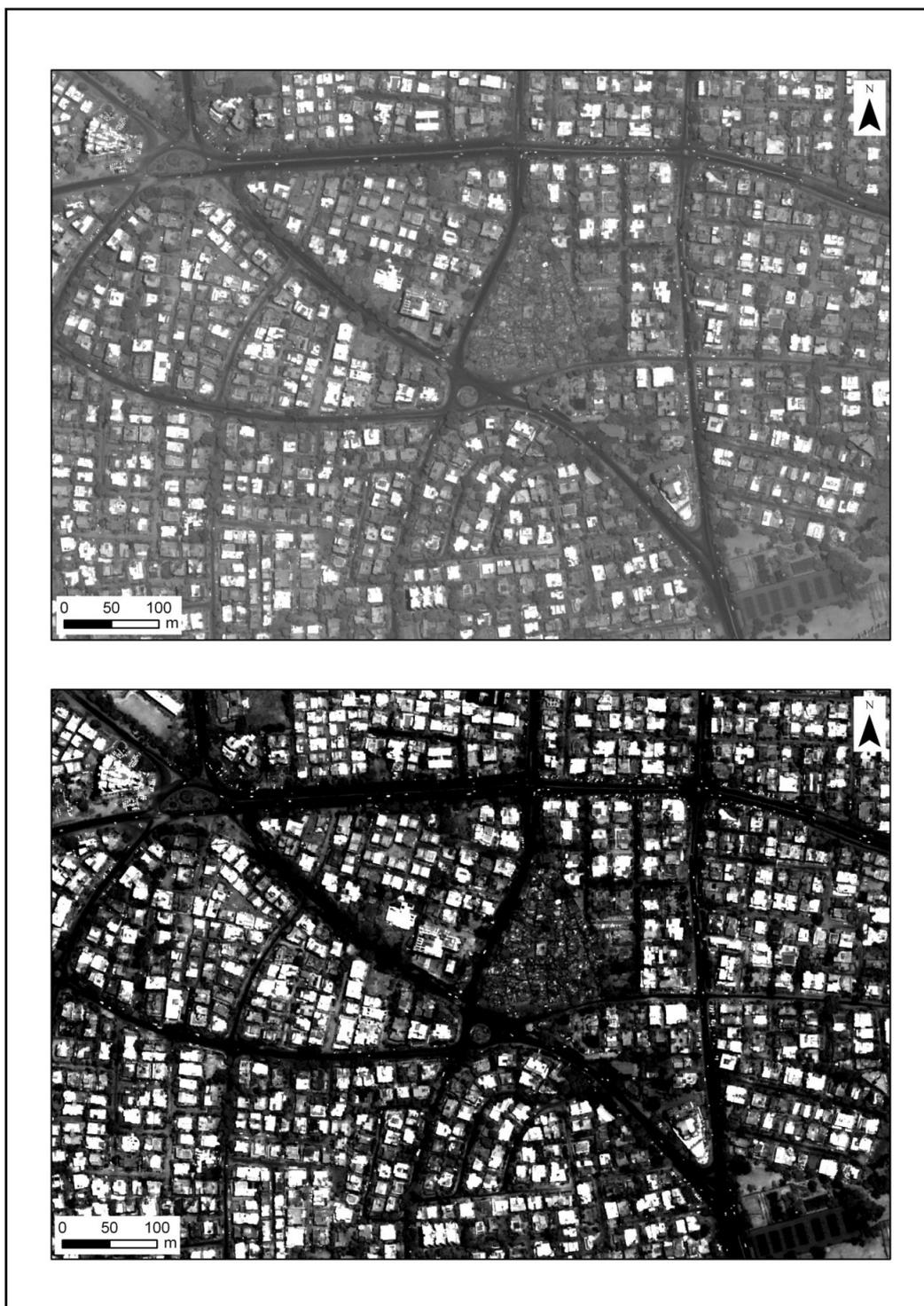
Figure 29: Linear stretch on panchromatic subset. The upper figure shows the original panchromatic image. The lower figure displays the linear stretched image in which the brightness of the moderate reflection objects is increased. From the image, it becomes obvious that less bright roofs can be observed in low income areas than in middle to high income areas.
