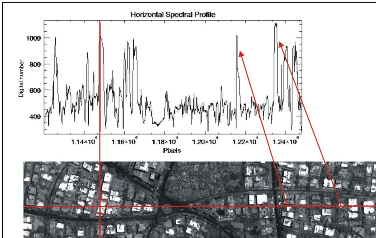
Figure 27: Panchromatic subset from Quickbird image and horizontal spectral profile. The bright roofs correspond well with the peak in the spectral profile.
