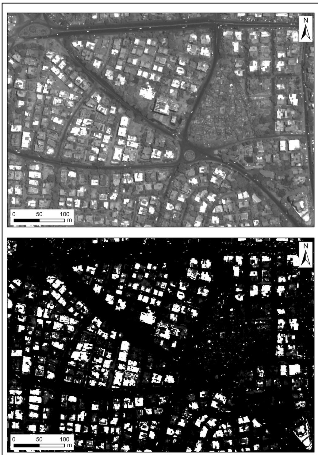
Figure 33: Square root stretch on panchromatic subset. The upper figure shows the original panchromatic image. The lower figure displays the linear stretched image with the data range set to 520 and 616.
