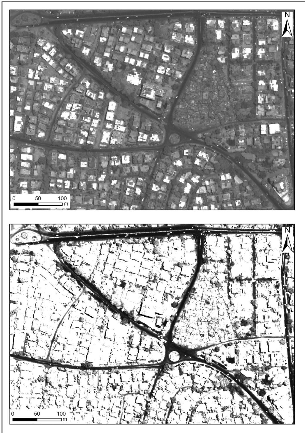
Figure 32: Histogram equalization stretch on panchromatic subset. The upper figure shows the original panchromatic image. The lower figure displays the linear stretched image with the data range set to 192 and 440.
