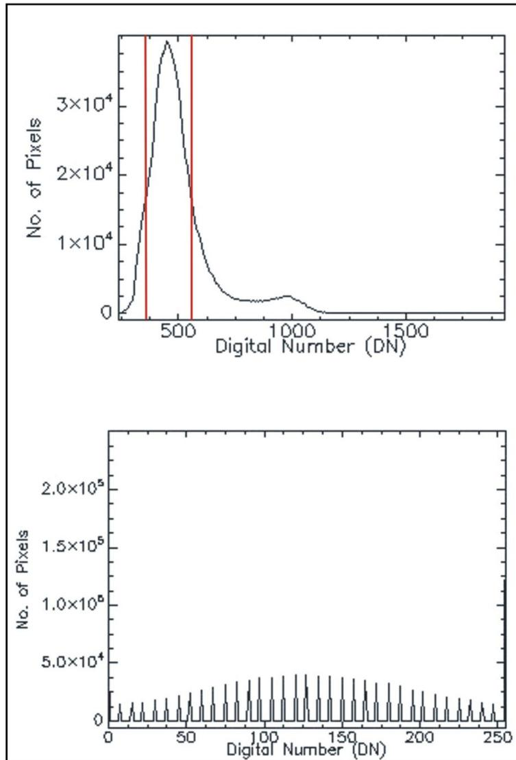
Figure 28: Linear stretch histograms. Upper histogram: The right peak between 900 and 1000 DN represents the high reflectance objects whereas the large peak represents the large portion of moderate reflectance objects. Lower histogram: Linear stretch for DN from 335 to 579 to increase the reflectance of the bright roofs which serve as an indicator for middle and high income areas.
