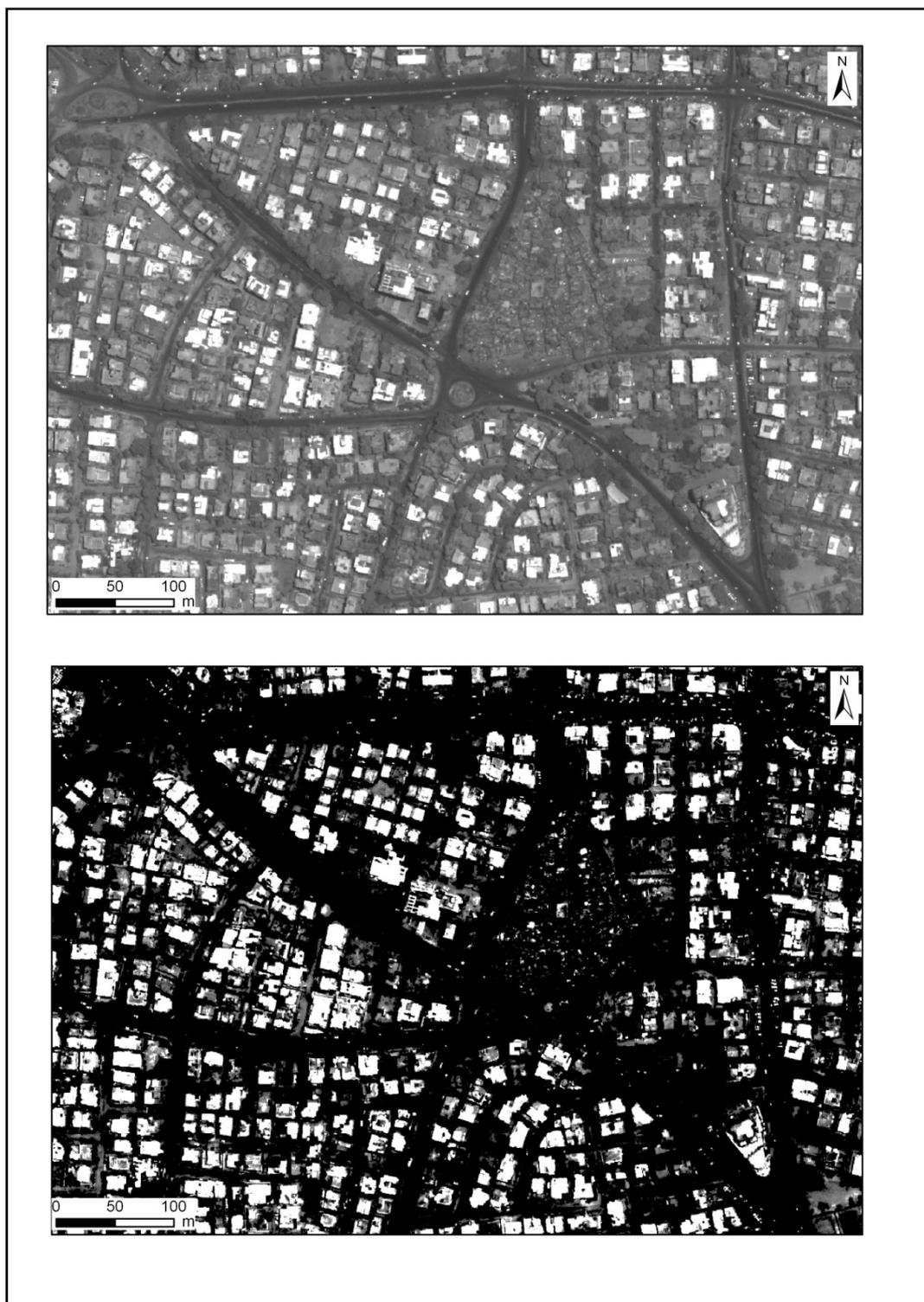
Figure 31: Gaussian stretch on panchromatic subset. The upper figure shows the original panchromatic image. The lower figure displays the linear stretched image with the data range set to 512 to 608.
