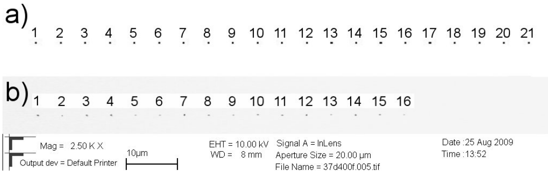
Figure 3.4: Dose study to get the base dose D_0 and \beta for our special resist system (470 nm MAA plus 220 nm PMMA 950 K) and substrate material (p-doped Si covered by 400 nm of oxide). a) shows the reference structure designed for this purpose: A series of directly adjacent bars of 1 \times 30 \mu\text{m}^2 written with from left (50% D ) to right (150% D ) in 10% steps increasing dose. b) is a camera picture of the structure taken after development. c) is the corresponding simulation. Red to green represents increasing dose, while blue on the right end corresponds to completely developed resist and on the left end to some very low exposure. d) illustrates the parameter fitting: simulation pictures with varying D_0 were laid across the photo until the left edges of the developed regions corresponded. The resulting base dose was D_0 = 141 \mu\text{A}\cdot\text{s}/\text{cm}^2 . \beta could only be found after the determination of \eta (see 3.5) by adjusting the form of the borders of the developed area. We got \beta = 4.0 \mu\text{m} .
