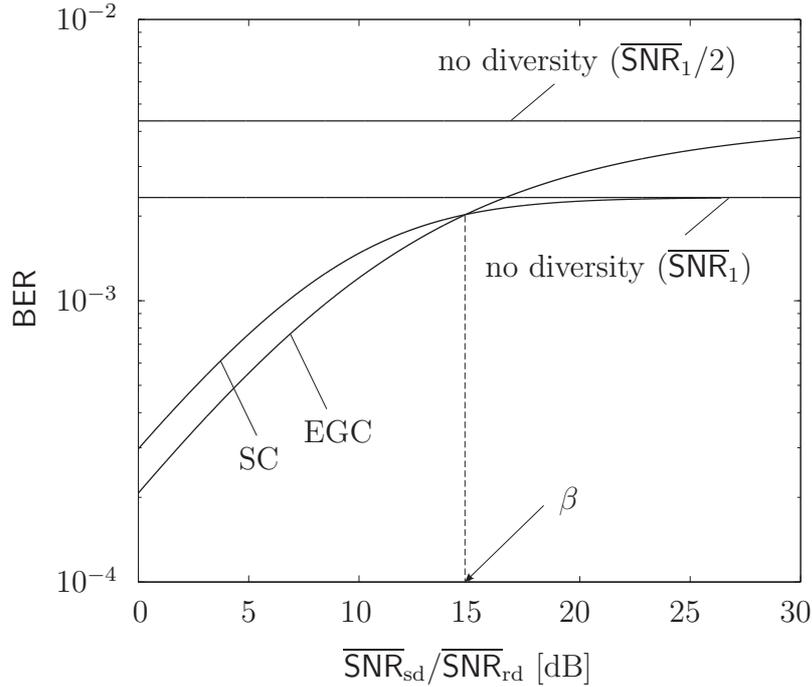
Figure 5.5: Bit error rate (BER) of selection combining (SC) and equal gain combining (EGC) for BPSK with respect to branch unbalance  $\overline{\text{SNR}}_{\text{sd}}/\overline{\text{SNR}}_{\text{rd}}$  [dB]. Parameter  $\overline{\text{SNR}}_{\text{sd}}$  was set to 10 dB.
