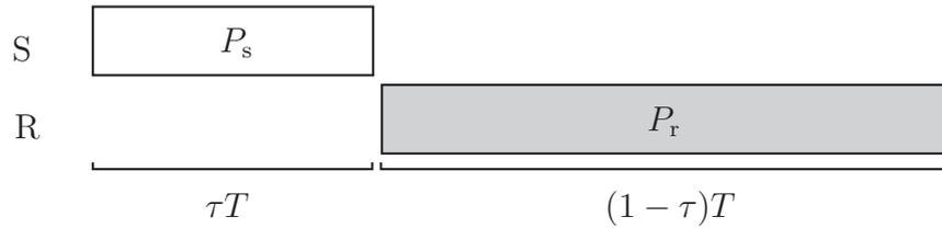
Figure 4.2: Basic transmission scheme. The first phase of duration  $\tau T$  is reserved for source transmission with power  $P_s$  and the second phase of duration  $(1 - \tau)T$  is reserved for relay transmission with power  $P_r$ .
