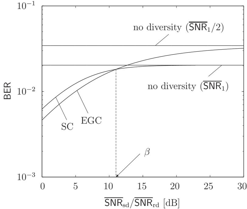
Figure 5.4: Bit error rate (BER) of selection combining (SC) and equal gain combining (EGC) for BPSK with respect to branch unbalance  $\overline{\text{SNR}}_{\text{sd}}/\overline{\text{SNR}}_{\text{rd}}$  [dB]. Parameter  $\overline{\text{SNR}}_{\text{sd}}$  was set to 5 dB.
