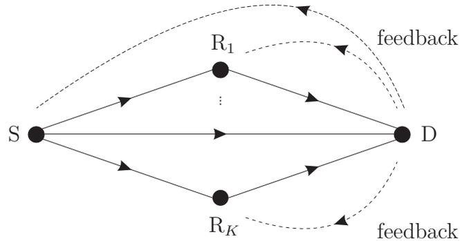
Figure 2.6: Principle of an incremental relaying network with one source  $S$ ,  $K$  relays  $R_k$ ,  $k = 1, \dots, K$ , and one destination  $D$ .
