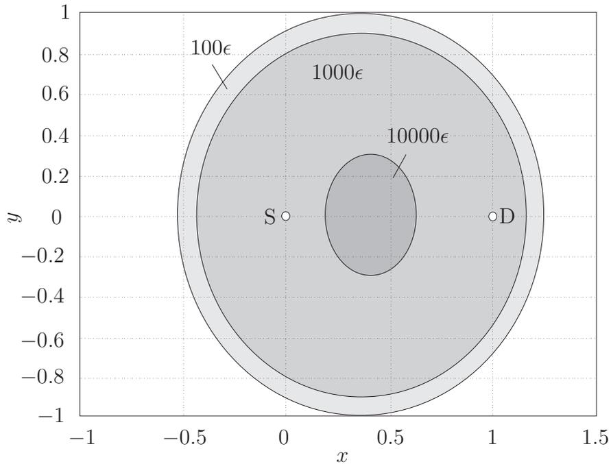
Figure 6.7: Regions where  $\epsilon$ -outage capacity of incremental relaying with decode-and-forward outperforms  $\epsilon$ -outage capacity of transmit diversity for different values of  $\Pr(\text{“source transmission fails”})$  as a function of  $\epsilon$ . Parameters are  $\epsilon = 10^{-4}$ ,  $\text{SNR} = 20$  dB, and  $\alpha = 3$ .
