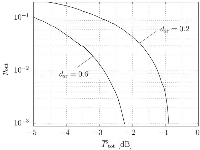
Figure 4.13: Outage probability vs. averaged total transmit power for  $d_{\text{sr}} = 0.2$  and  $d_{\text{sr}} = 0.6$ .
