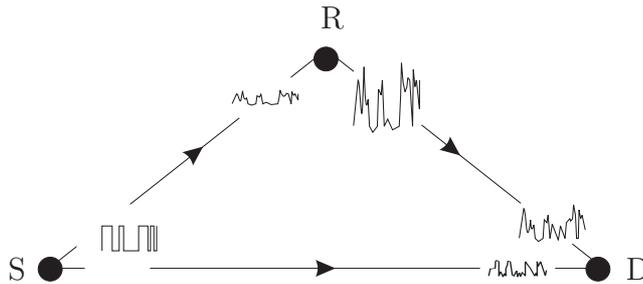
Figure 2.7: The functionality of amplify-and-forward (AF).
