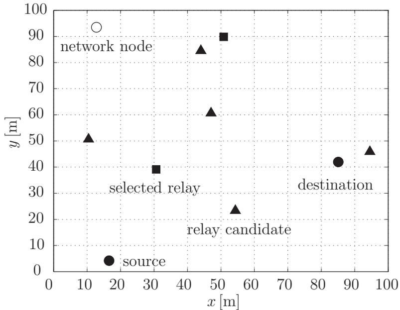
Figure 3.6: Network constellation of example 1 with  $\mathbf{x} = [20.5111]^T$  and BER =  $10^{-3}$ .
