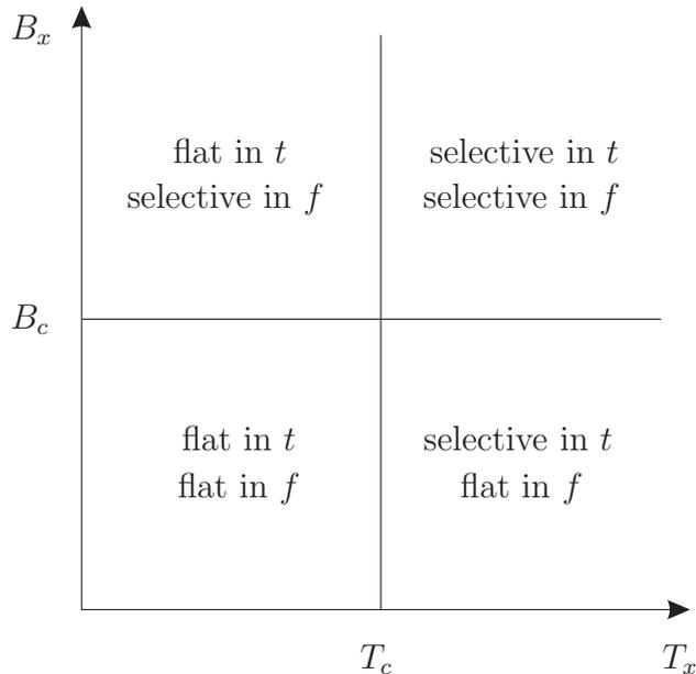
Figure 2.1: Classification of wireless channels (cf. [69]).
