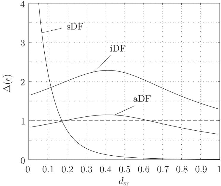
Figure 6.5: Ratio between  $\epsilon$ -outage capacity of relaying protocols and transmit diversity vs. source-relay distance  $d_{\text{sr}}$  for  $\epsilon = 10^{-4}$ ,  $\text{SNR} = 20$  dB, and  $\alpha = 3$ . Curve sections that are above the dashed line indicate regions in which the cooperative protocols outperform transmit diversity.
