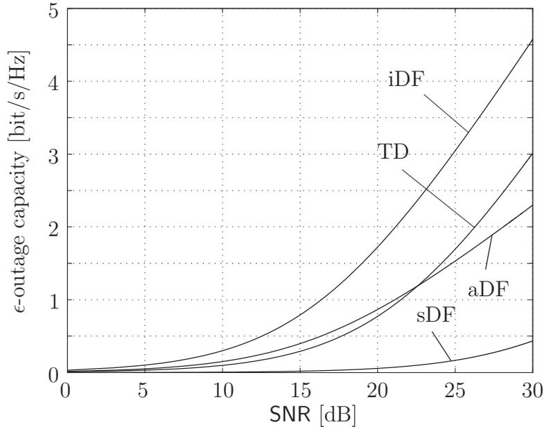
Figure 6.4:  $\epsilon$ -outage capacity in bit/s/Hz vs. SNR in dB for an outage probability of  $\epsilon = 10^{-4}$  and  $\alpha = 3$ . The relay has been placed at  $d_{\text{sr}} = 0.5$ .
