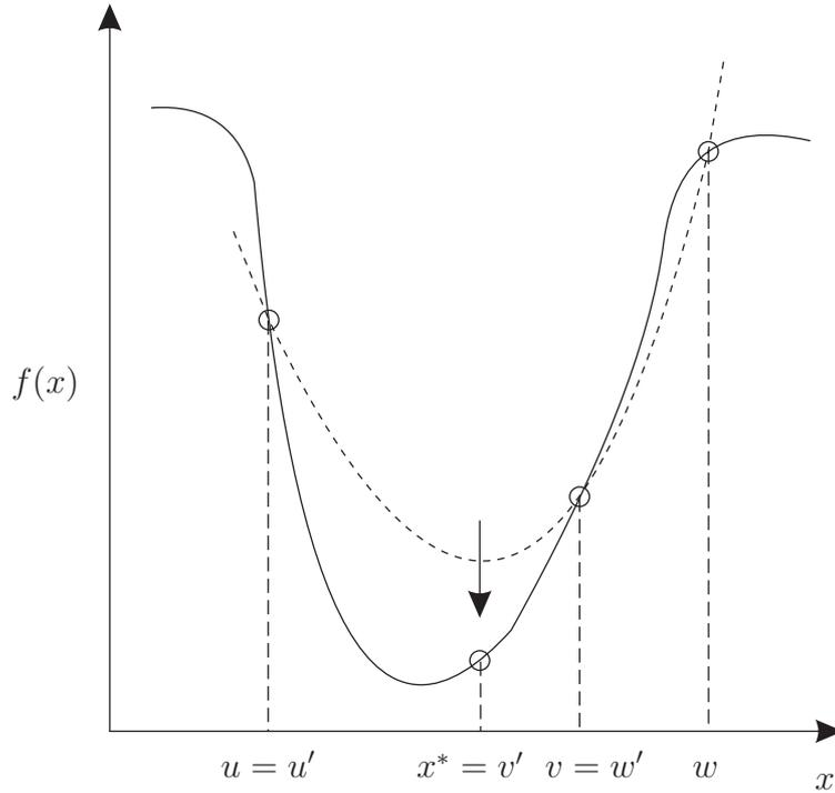
Figure 4.4: Parabolic interpolation.
