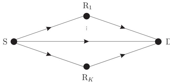
Figure 2.4: Principle of a multi-route network with one source  $S$ ,  $K$  relays  $R_k$ ,  $k = 1, \dots, K$ , and one destination  $D$ .
