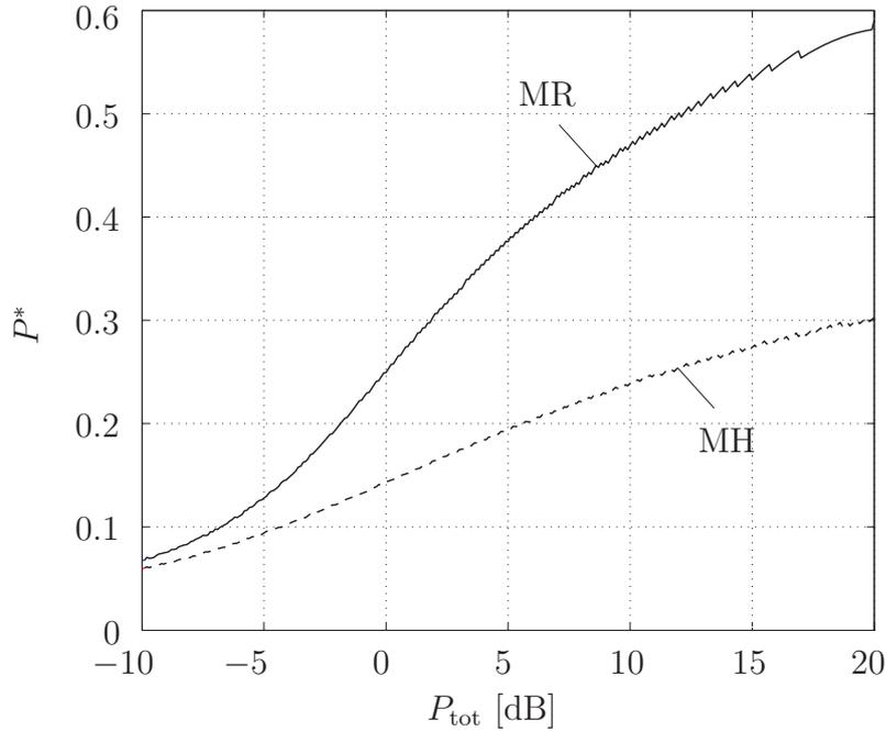
Figure 4.7: Optimal power allocation  $P^* = \tau^* P_s / P_{\text{tot}}$  for the source. The distance source-relay has been set to  $d_{\text{sr}} = 0.3$ .
