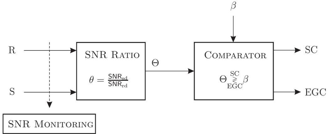
Figure 5.3: Structure of a dual-diversity combining receiver that selects between selection combining (SC) and equal gain combining (EGC) on the basis of an SNR criterion.
