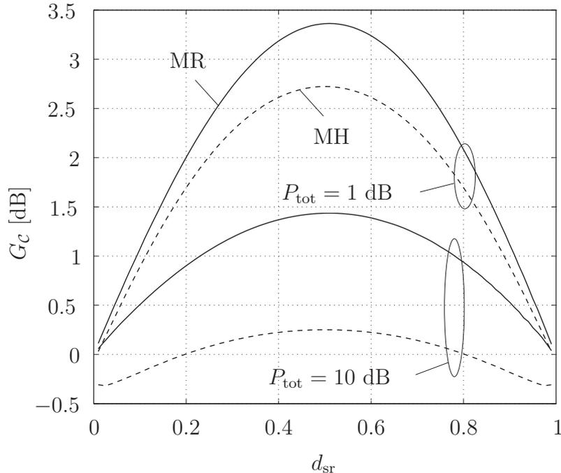
Figure 4.9: Capacity gain  $G_c$  of multi-route and multi-hop over direct transmission when optimized power allocation  $P^*$  and optimized time allocation  $\tau^*$  are used.
