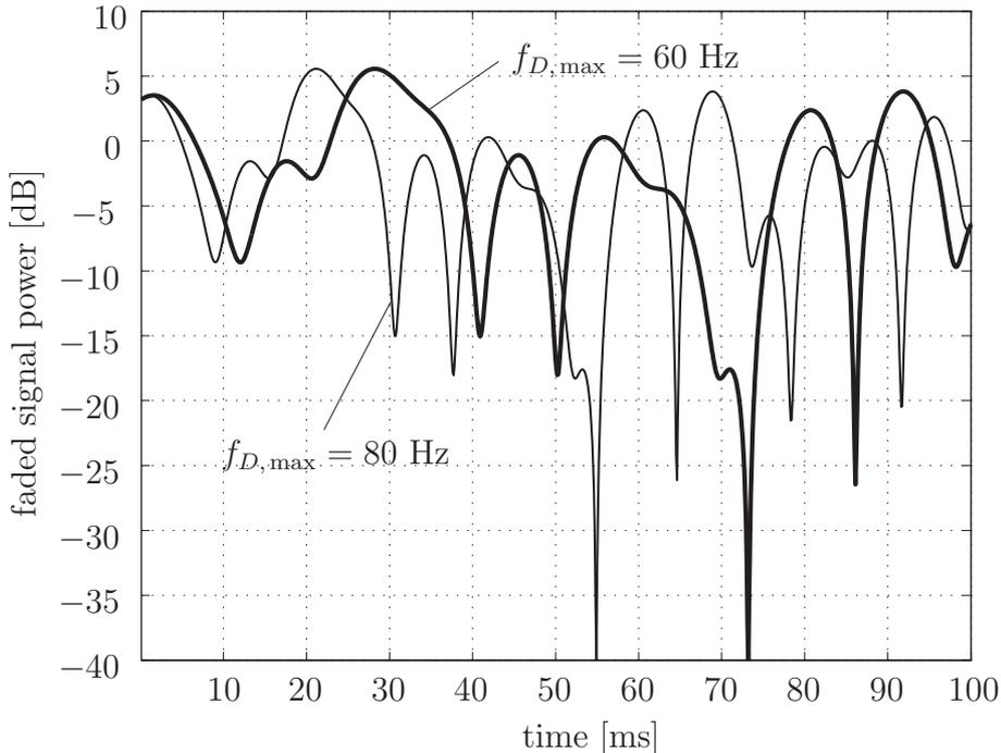
Figure 1.1: Faded signal power [dB] of a signal that is transmitted over two different Rayleigh fading channels with a maximum Doppler shift of  $f_{D,\max} = 80$  Hz (thin line) and  $f_{D,\max} = 60$  Hz (thick line), respectively. Sampling time equals  $100 \mu\text{s}$ .
