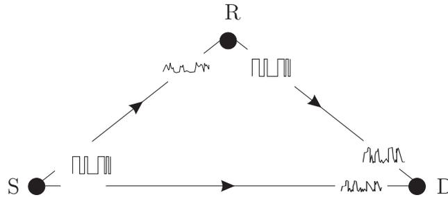
Figure 2.8: The functionality of decode-and-forward (DF).
