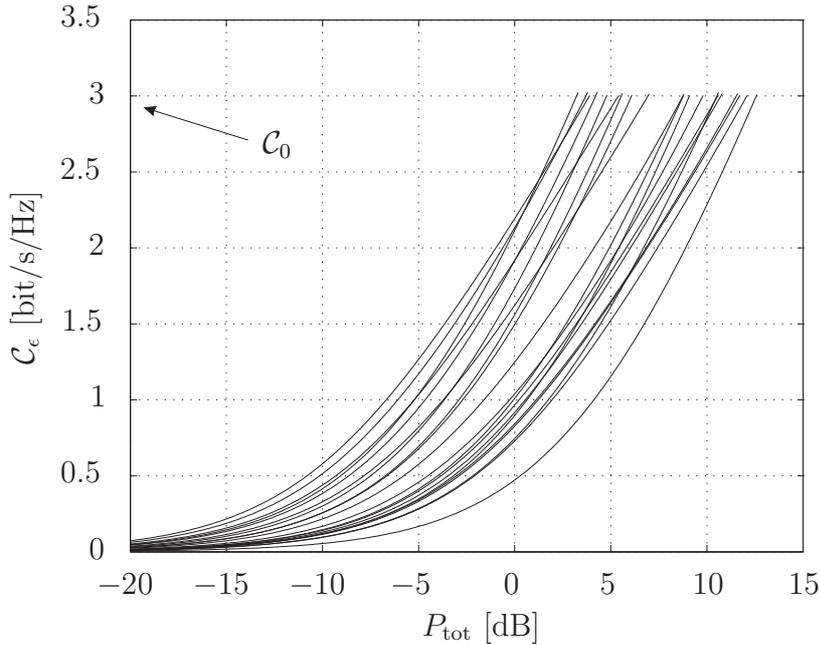
Figure 4.10: Delay-limited capacity vs. total transmit power for selective multi-route and the parameters  $d_{\text{sr}} = 0.2$  and  $\alpha = 4$ .
