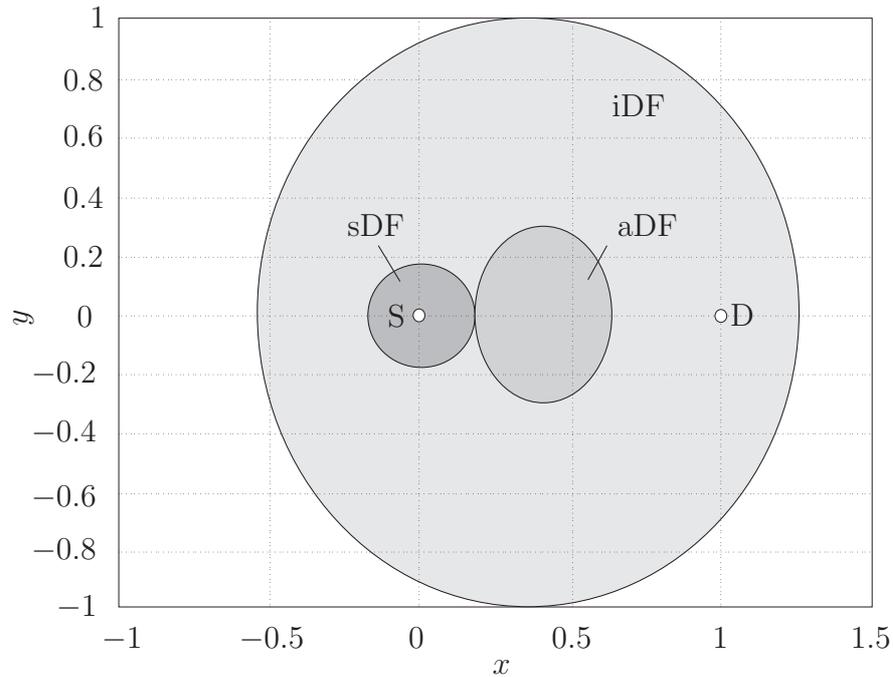
Figure 6.6: Regions in which  $\epsilon$ -outage capacity of the cooperative relaying protocols outperforms  $\epsilon$ -outage capacity of transmit diversity for  $\epsilon = 10^{-4}$ , SNR = 20 dB, and  $\alpha = 3$ .
