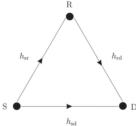
*Figure 5.1:* Statistically symmetric relay network with source S, relay R, and destination D. Statistically symmetric means that in average all channel coefficients are equal.
