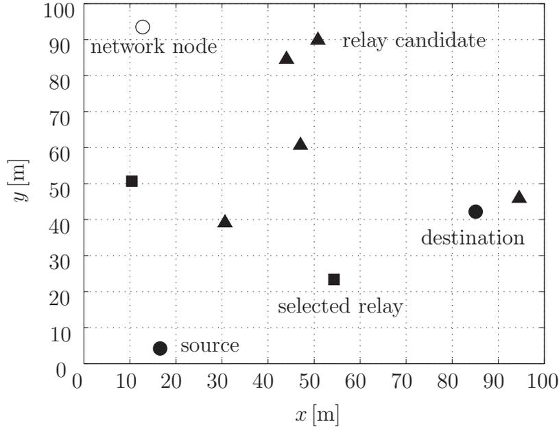
Figure 3.7: Network constellation of example 2 with  $\mathbf{x} = [1 \ 2 \ 1 \ 1 \ 1]^T$  and  $\text{BER} = 10^{-3}$ .
