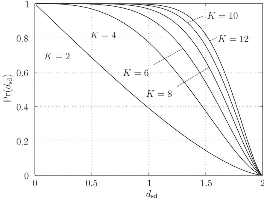
Figure 3.2: Probability of finding at least one relay candidate.
