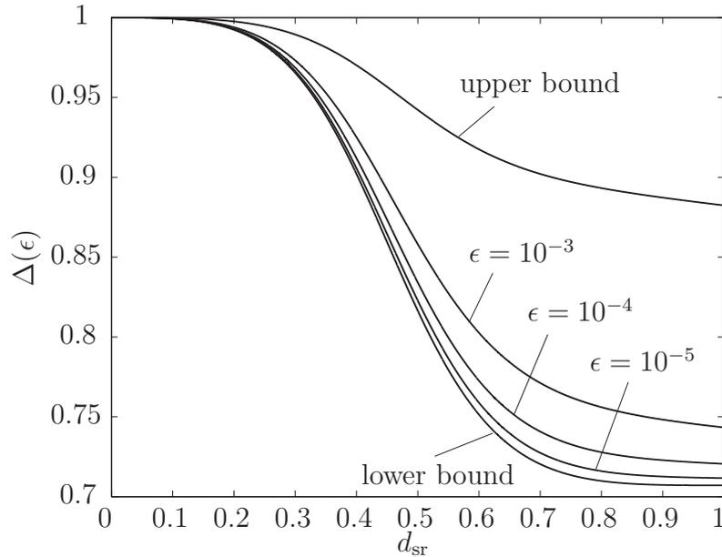
Figure 6.9: Ratio  $\Delta(\epsilon)$  of the  $\epsilon$ -outage capacity of incremental relaying with decode-and-forward to the cut-set bound for  $g \rightarrow 0$  and  $\alpha = 3$ .
