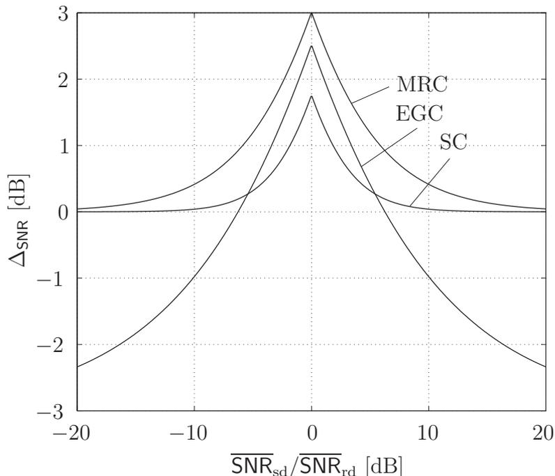
Figure 5.2: Comparison of the SNR gain  $\Delta_{\text{SNR}}$  of selection combining (SC), equal gain combining (EGC), and maximal ratio combining (MRC) with respect to branch unbalance  $\overline{\text{SNR}}_{\text{sd}}/\overline{\text{SNR}}_{\text{rd}}$  [dB].
