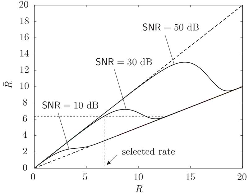
Figure 6.1: Mapping of  $R$  to  $\bar{R}$ . Dashed lines illustrate upper and lower bounds. The upper bound is given by  $\bar{R} = R$  and the lower bound is given by  $\bar{R} = R/2$ . In [37] the smallest  $R$  out of those is selected that determine the same  $\bar{R}$ .
