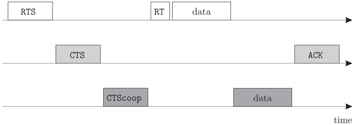
Figure 3.3: General functionality of the adaptive relay selection protocol (ARSP), where one relay has been selected.
