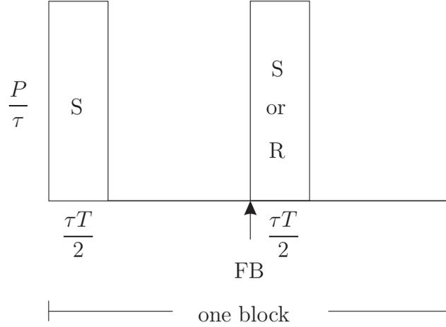
Figure 6.8: Transmission model for incremental relaying with AF and BAF. If the source transmission succeeded (feedback  $\text{FB} = 1$ ), the source transmits during the second sub-block, too. If the source transmission failed (feedback  $\text{FB} = 0$ ), the relay aids communication during the second sub-block.
