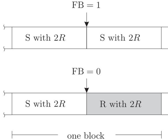
*Figure 6.2:* Transmission model for incremental relaying. If the source-destination link is not in outage (feedback  $\text{FB} = 1$ ), the source transmits during the second sub-block, too. If the source-destination link is in outage (feedback  $\text{FB} = 0$ ), the relay aids communication during the second sub-block.
