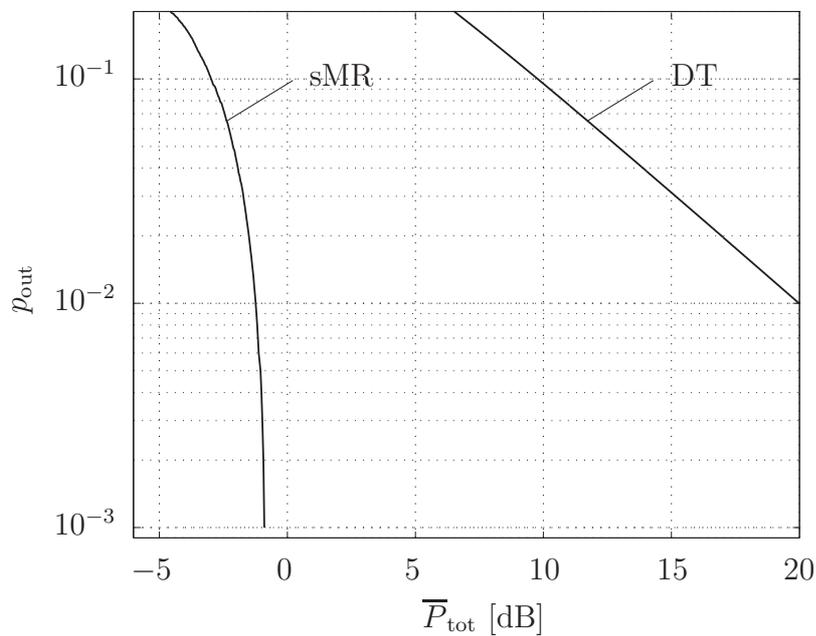
Figure 4.14: Outage probability of selective multi-route and direct transmission vs. averaged total transmit power for  $C_0 = 1$  bit/s/Hz,  $d_{\text{sr}} = 0.2$ , and  $\alpha = 4$ .
