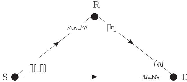
Figure 2.9: The functionality of compress-and-forward (CF).
