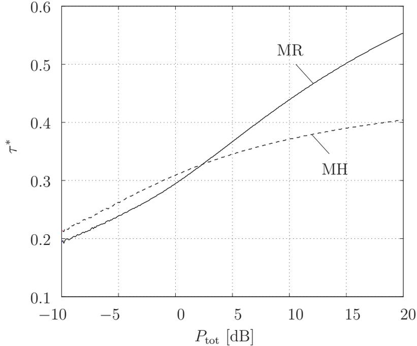
Figure 4.8: Optimal time allocation  $\tau^*$  for the source. The distance source-relay has been set to  $d_{\text{sr}} = 0.3$ .
