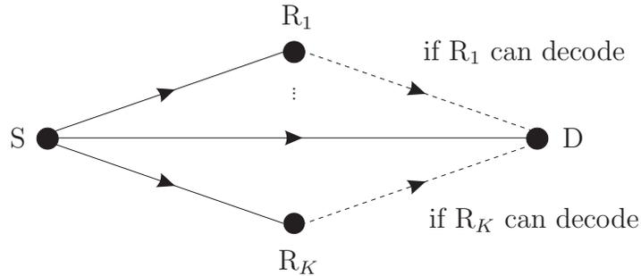
Figure 2.5: Principle of an adaptive multi-route network with one source S,  $K$  relays  $R_k$ ,  $k = 1, \dots, K$ , and one destination D.
