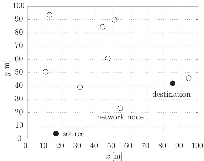
Figure 3.9: Network constellation of example 4 with  $\mathbf{x} = [1 \ 2 \ 1 \ 1 \ 1]^T$  and  $\text{BER} = 10^{-2}$ .
