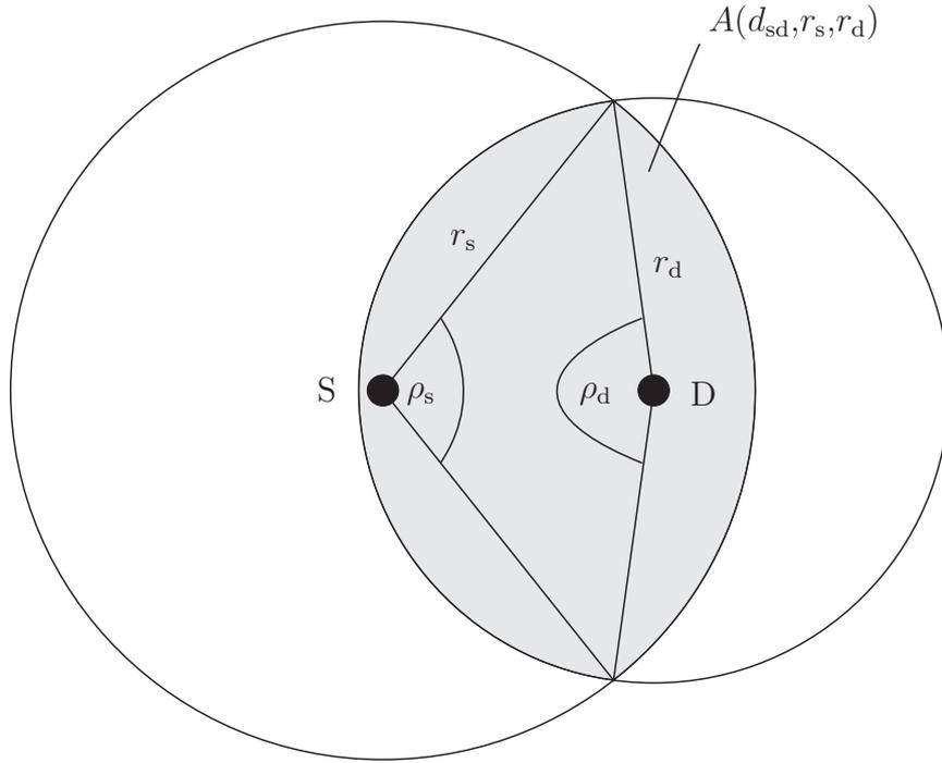
Figure 3.1: Relay area  $A(d_{sd}, r_s, r_d)$ .
