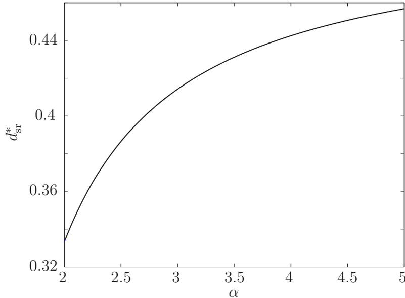
Figure 6.3: Optimal source-relay distance  $d_{sr}^*$  vs. path-loss factor  $\alpha$ . For  $\alpha \rightarrow \infty$   $d_{sr}^*$  tends asymptotically to  $d_{sr}^* = 0.5$ .  $d_{sr}^*(\alpha = 2) = 1/3$ .
