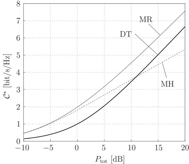
Figure 4.6: Instantaneous channel capacities with optimal resource allocation for multi-hop (MH) and multi-route (MR) in bit/s/Hz. The distance source-relay has been set to  $d_{\text{sr}} = 0.3$ . Capacity of direct transmission (DT) is illustrated as reference.
