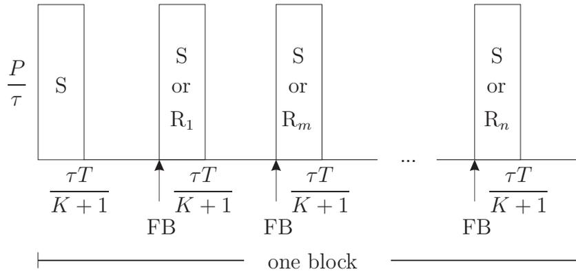
Figure 6.11: Transmission model for BAF with incremental relaying and an arbitrary number of relay nodes.  $R_m$ ,  $m \in \{1, 2\}$ , and  $R_n$ ,  $n \in \{1, 2, \dots, K\}$ , describe the transmitting relay depending on prior transmissions.
