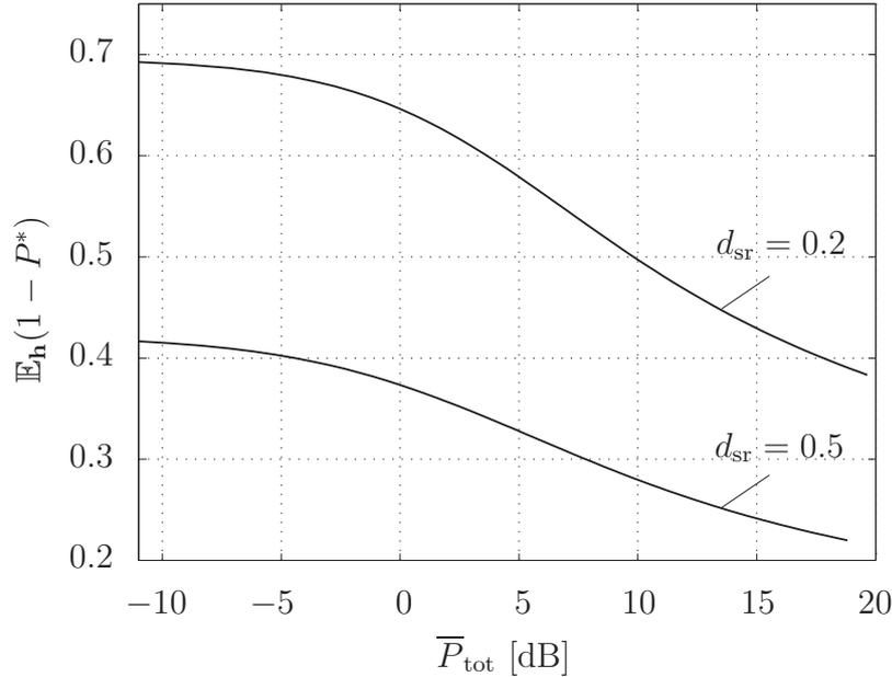
Figure 4.12: Averaged optimal power allocation for the relay vs. averaged total transmit power for  $d_{\text{sr}} = 0.2$  and  $d_{\text{sr}} = 0.5$ .
