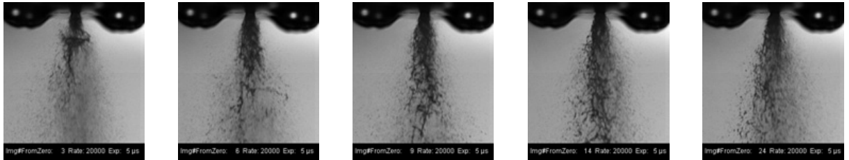
Figure 4. High speed video images of the spray structure: CS 4,5 wt.%, ALR 0,228
