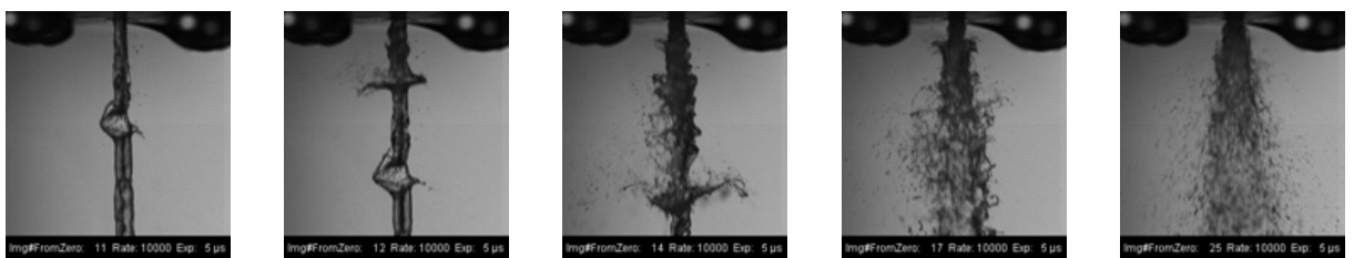
Figure 8. High speed video images of the spray structure: CS 5,5 wt.%, ALR 0,293
