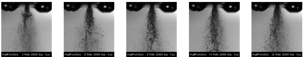
Figure 7. High speed video images of the spray structure: CS 4,5 wt.%, ALR 0,228
