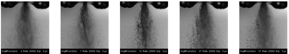
Figure 6. High speed video images of the spray structure: CS 3,5 wt.%, ALR 0,281
