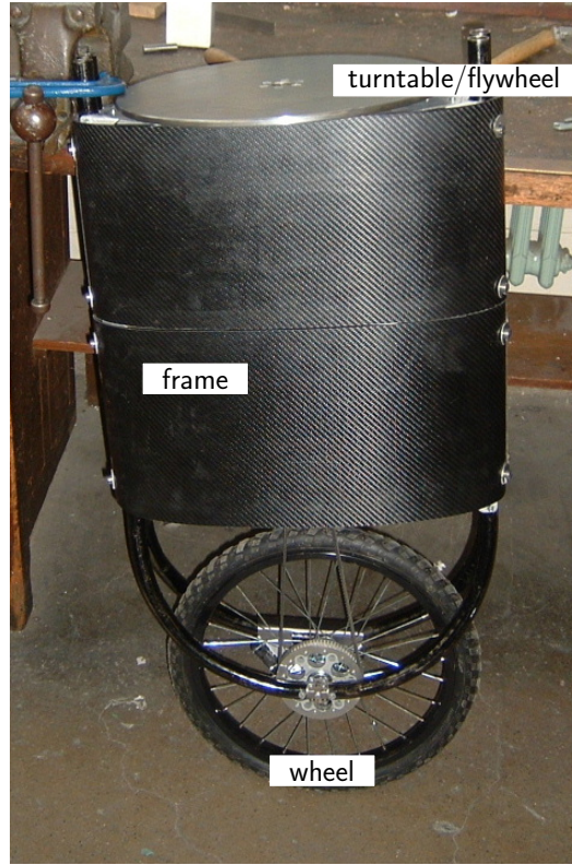
Figure 3.39: Robotic unicycle in the Department of Engineering, University of Cambridge, UK. With permission borrowed from http://www.roboticunicycle.info/ .
