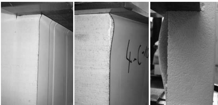
Figure 7: Failure modes at load application
