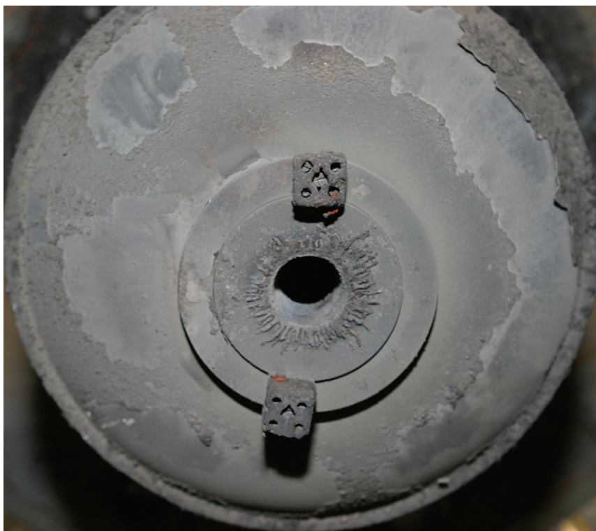
Fig. 4-92. KH03: Post test view of RPV lower head and hole
