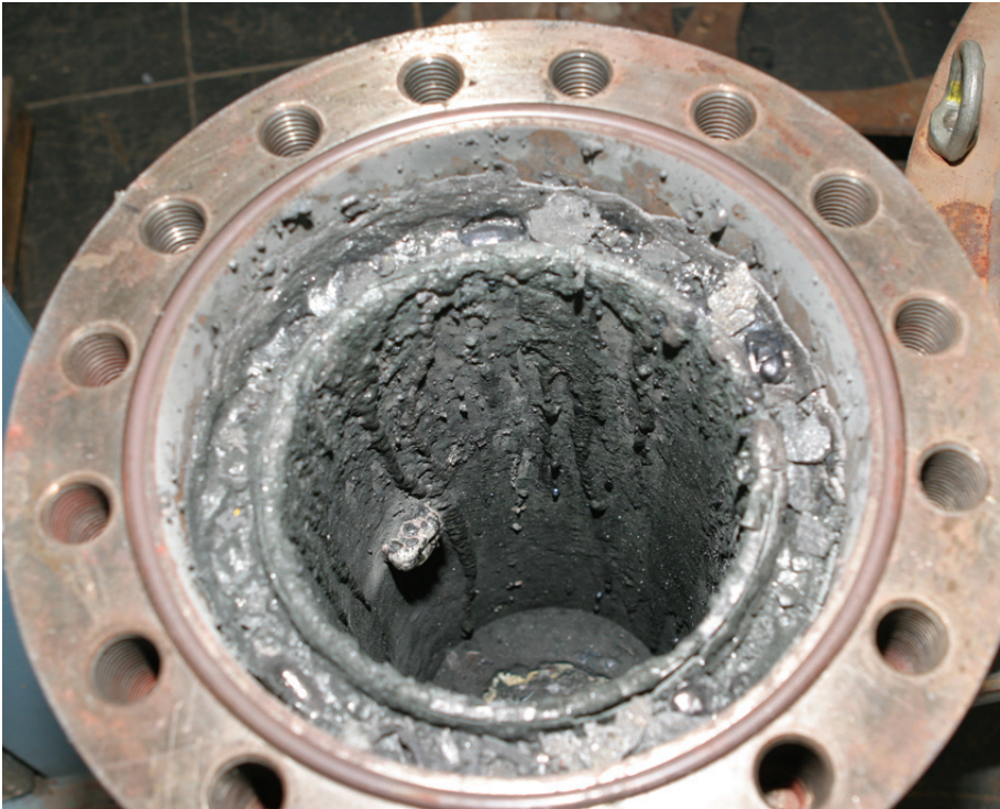
Fig. 4-130. KH05: Post test view of inside of RPV
