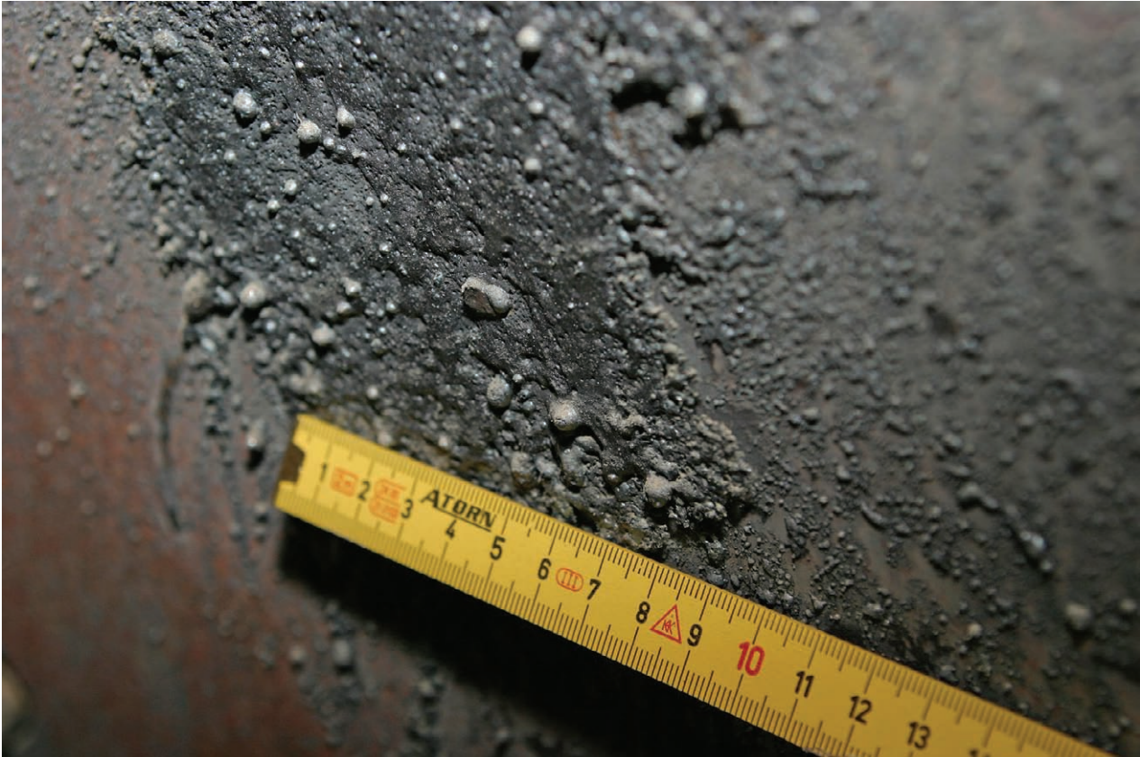
Fig. 4-21. KH01: Crust on the wall of subcompartment 1
