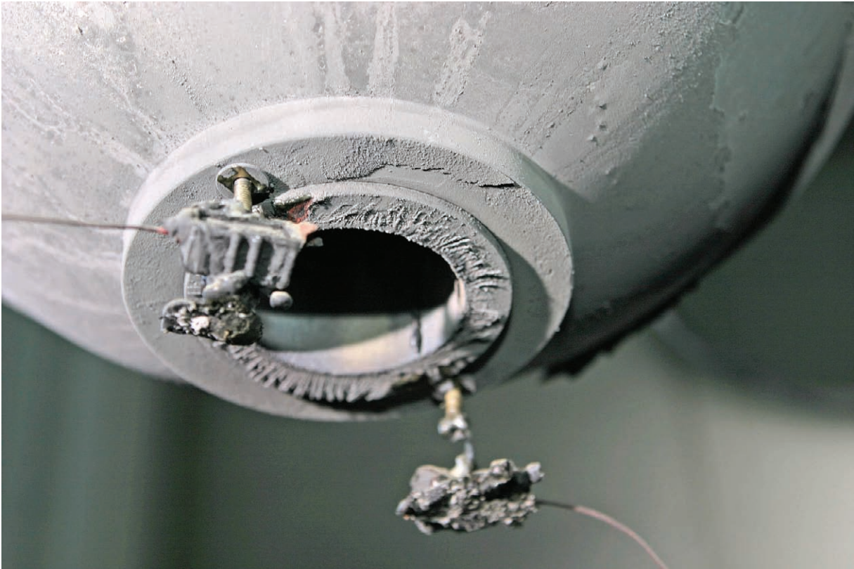
Fig. 4-18. KH01: Post test view of RPV lower head and hole
