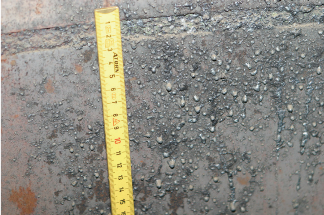
Fig. 4-112. KH04: Crust on the wall of subcompartment 1 opposite of main cooling line
