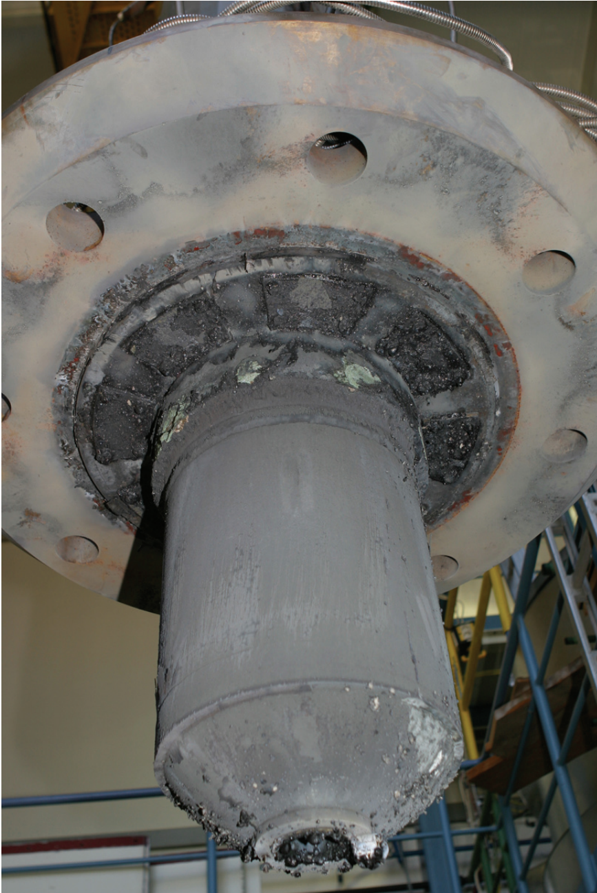
Fig. 4-128. KH05: Post test view of RPV
