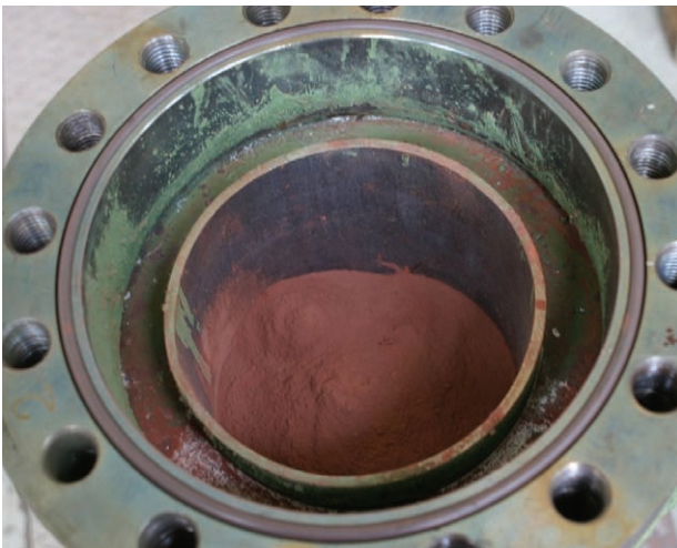
Fig. 3-24. Crucible with thermite powder, filled (left) and pressed with ignition wire (right)
