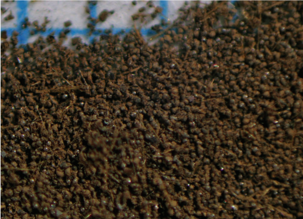
Fig. 4-33. Shape of debris particles, 0,056 – 0,08 mm
