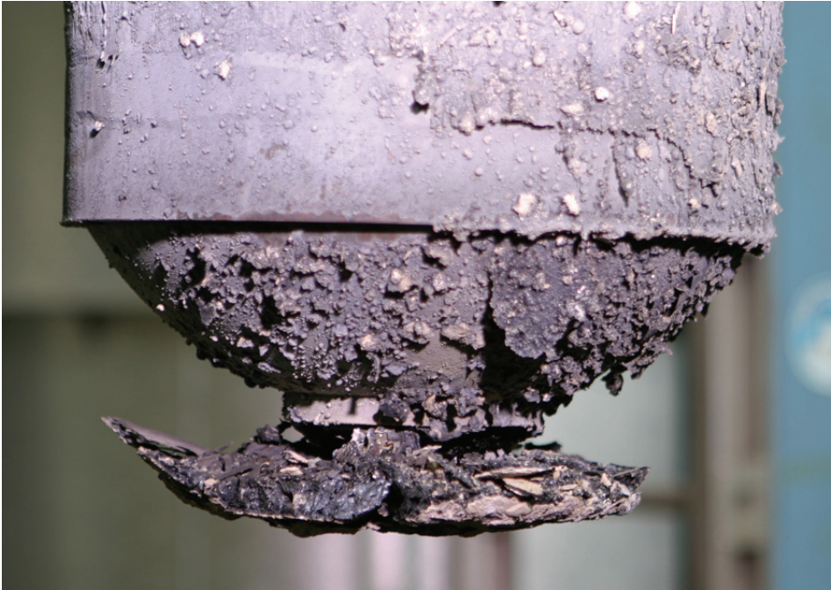
Fig. 4-144. KH06: Post test view of lower part of RPV
