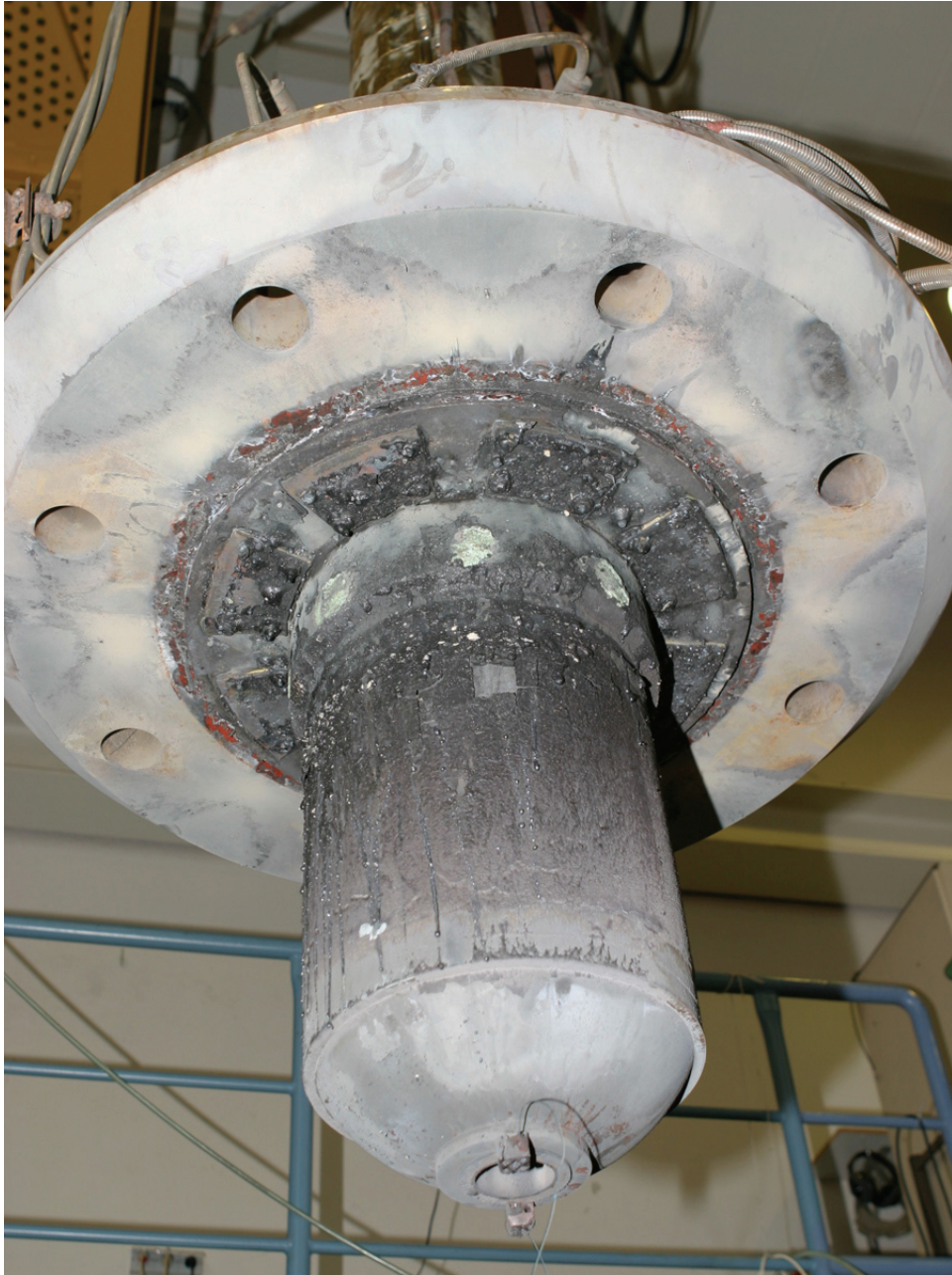
Fig. 4-75. KH02: Post test view of RPV lower head and hole
