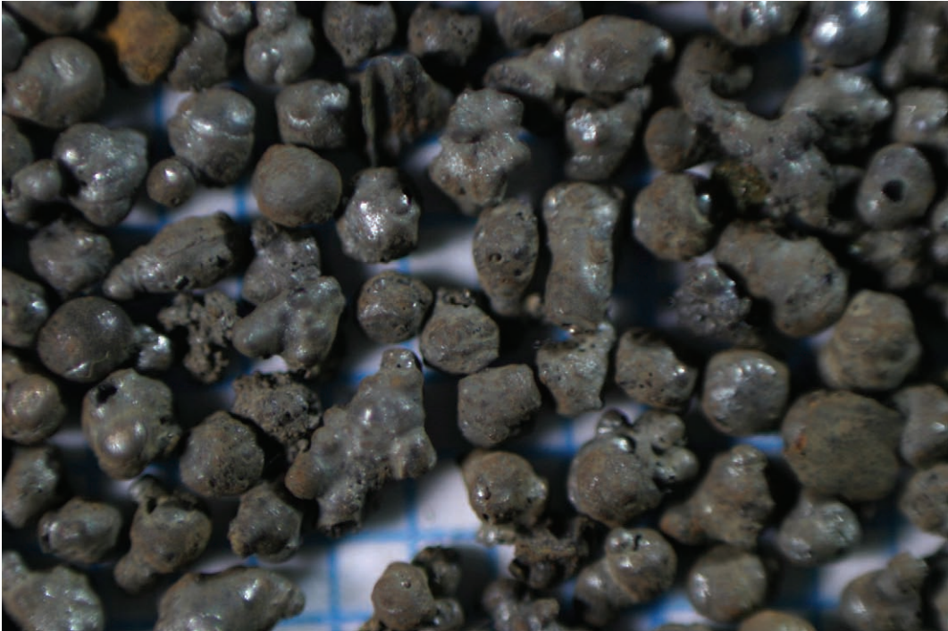
Fig. 4-29. Shape of debris particles, 0,9 – 1,25 mm
