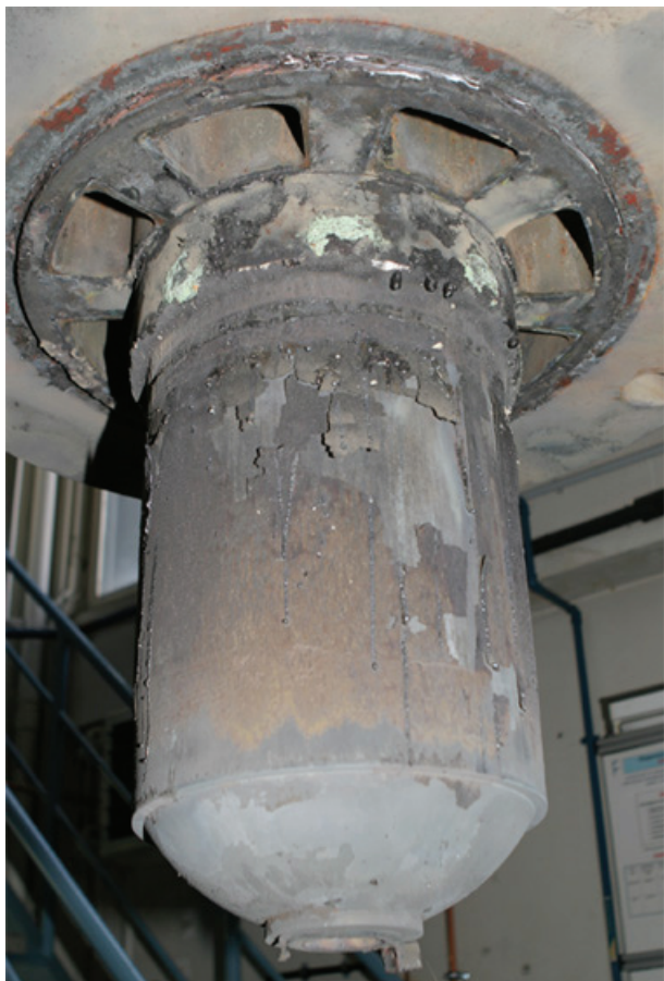
Fig. 4-110. KH04: Post test view of RPV
