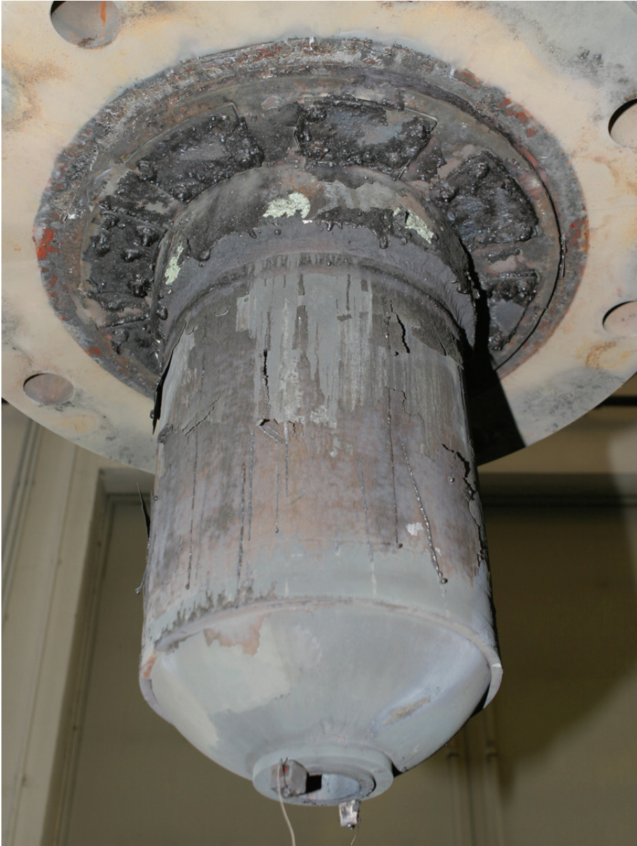
Fig. 4-157. KH07: Posttest view of RPV
