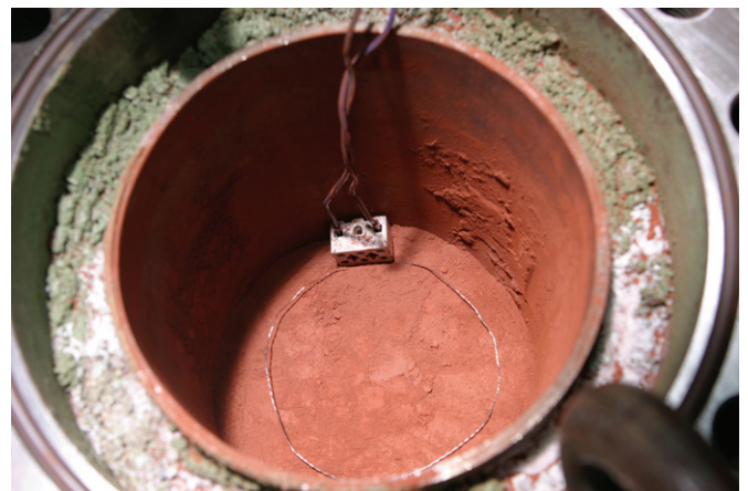
Fig. 3-24. Crucible with thermite powder, filled (left) and pressed with ignition wire (right)
