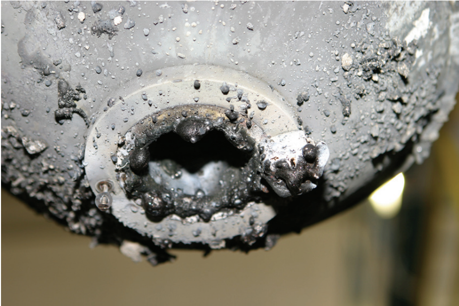
Fig. 4-129. KH05: Post test view of hole in RPV
