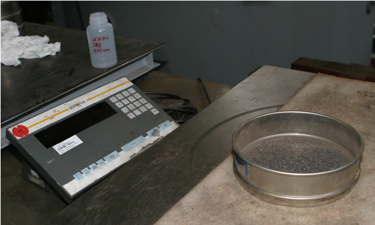
Fig. 3-26. Weighing of a sieve with particles
