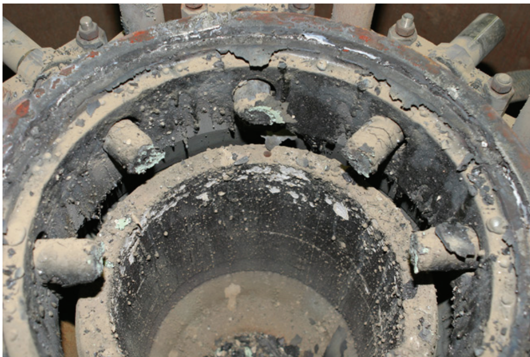
Fig. 4-110. KH04: Post test view of RPV
