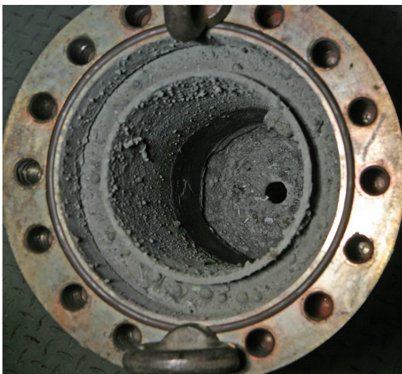
Fig. 4-93. KH03: Post test view into RPV (crucible)
