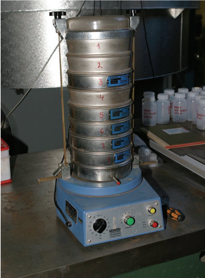
Fig. 3-25. Sieving vibrating unit with 8 of 17 sieves
