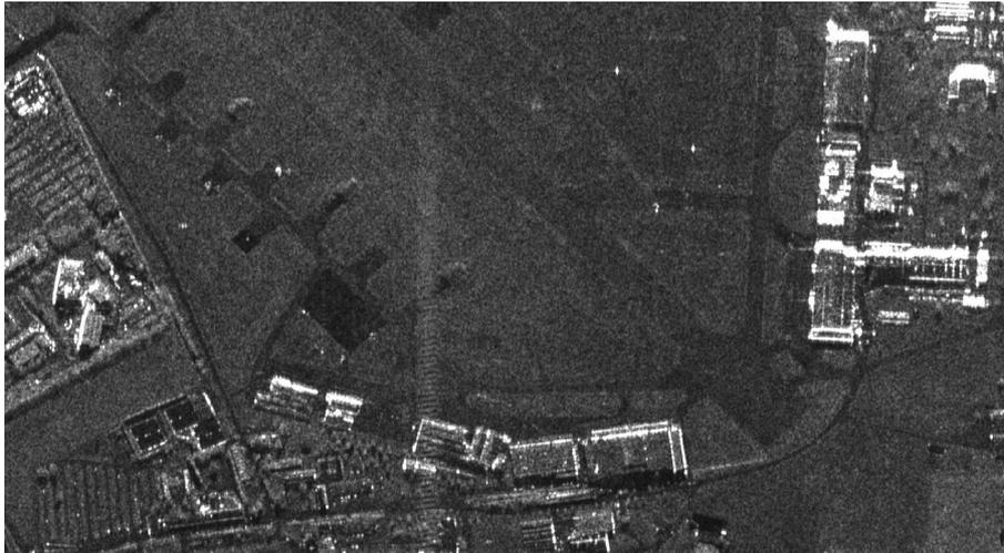
Fig. 10. Sub-image (X-band) acquired by the E-SAR sensor showing parts of the airport in Oberpfaffenhofen, close to Munich, Germany.
