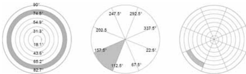
**Abbildung 21.3:** Illumination patterns. Left: Rings with polar angles. Center: Sectors with azimuth angles. Right: Combination of rings and sectors.
