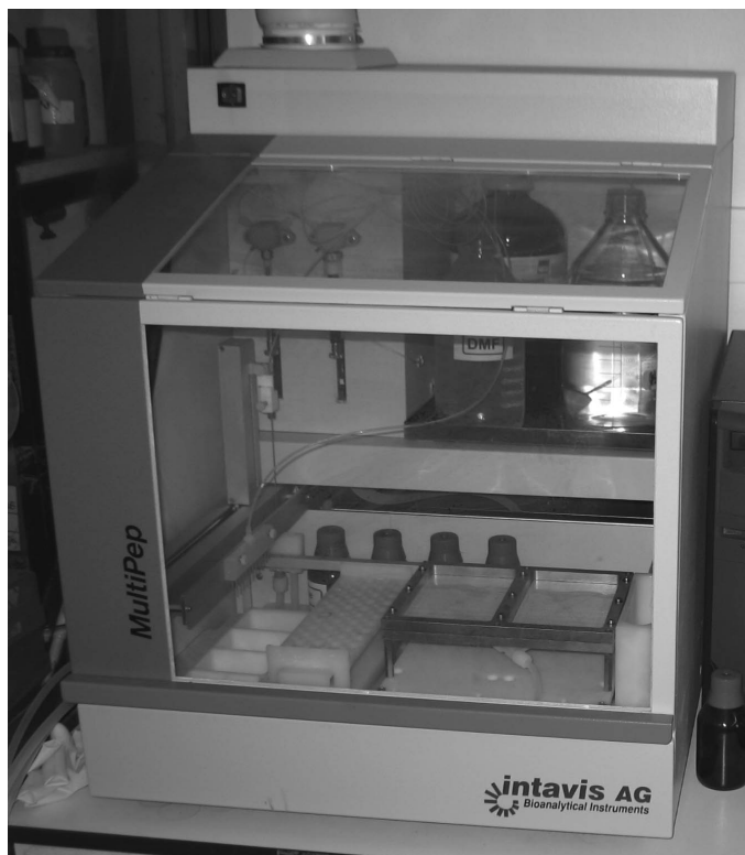
Figure 15: Fully automatic spot synthesizer. The MultiPep Spotter by Intavis AG, Köln.
