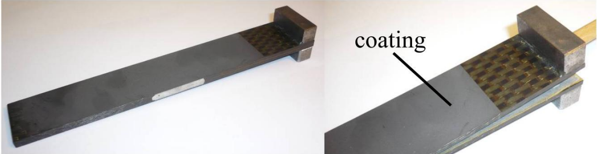
Figure 5. CFRP coupon with artificial delamination
