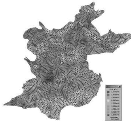
Fig. 4 Hydraulic Conductivity Map (30 – 60/120 m in depth)
