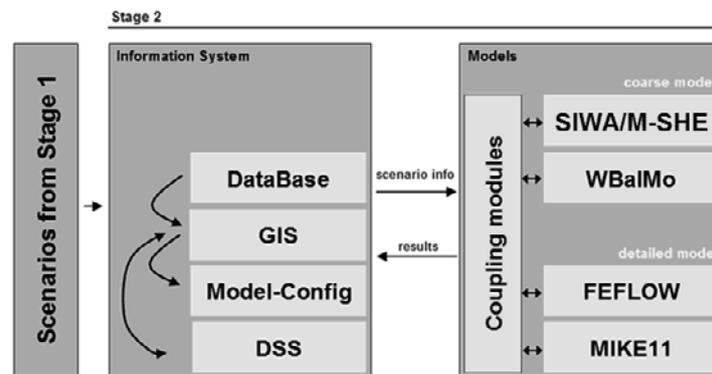
Fig. 3: Concept of the GIS-based and model supported DSS2 system
