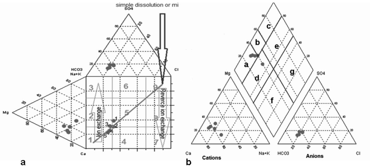
**Figure 4:** Hydrochemical data interpretation using aquachem, a: Durove diagram of ground water samples. b: Piper diagram for ground water samples.
