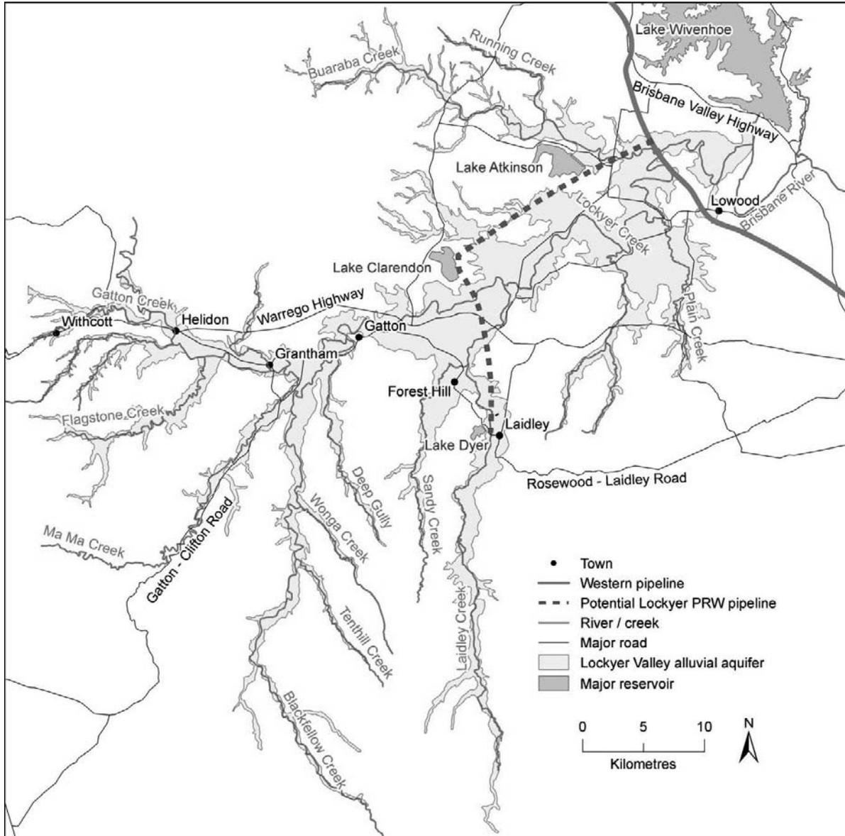
Fig.2: The Lockyer Valley alluvial aquifer and the planned diversion from the Western Pipeline
