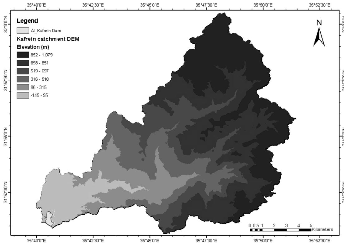
Fig. 1: High accuracy DEM extracted from Cartosat-1 imagery data with final cell size of 5m x 5m (Alkhoury, 2010).
