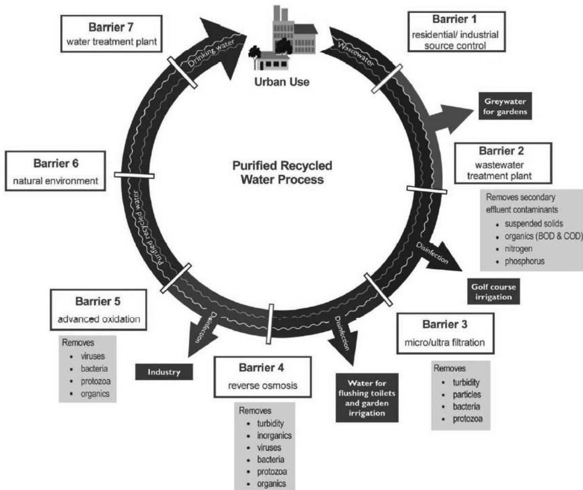
Fig.1: The multi-barrier concept for indirect potable reuse in Queensland [1]
