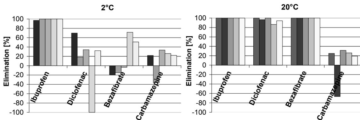
Fig.5 Elimination of selected pharmaceutical residues after trickling through soil columns operated at different temperatures
