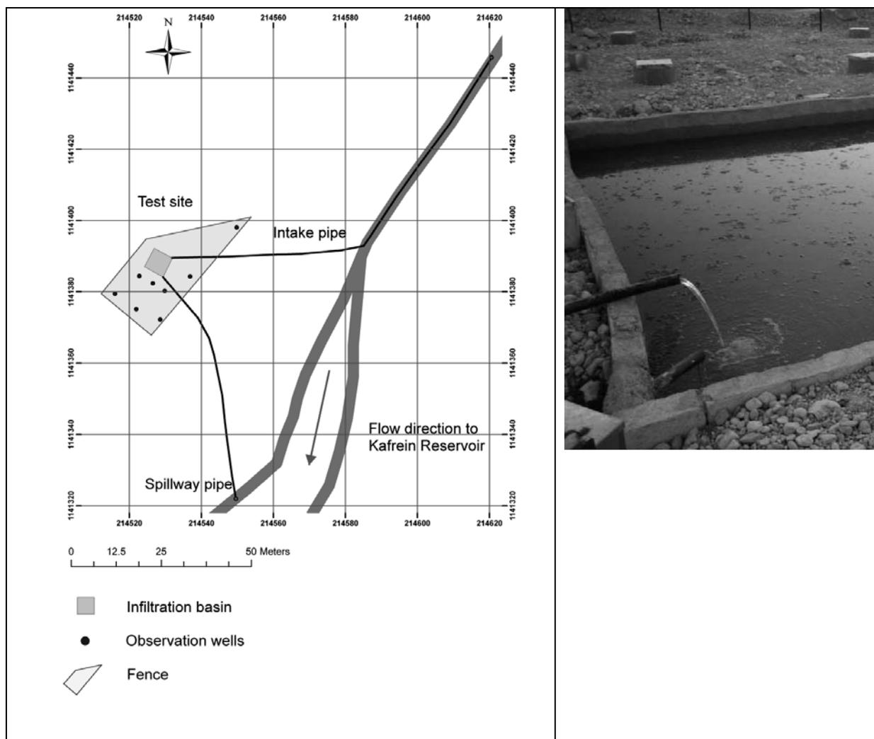
Figure 3: Artificial recharge test side at the Wadi Kafrein; left schematic map, right Foto of the infiltration basin (Wolf et al., 2009)
