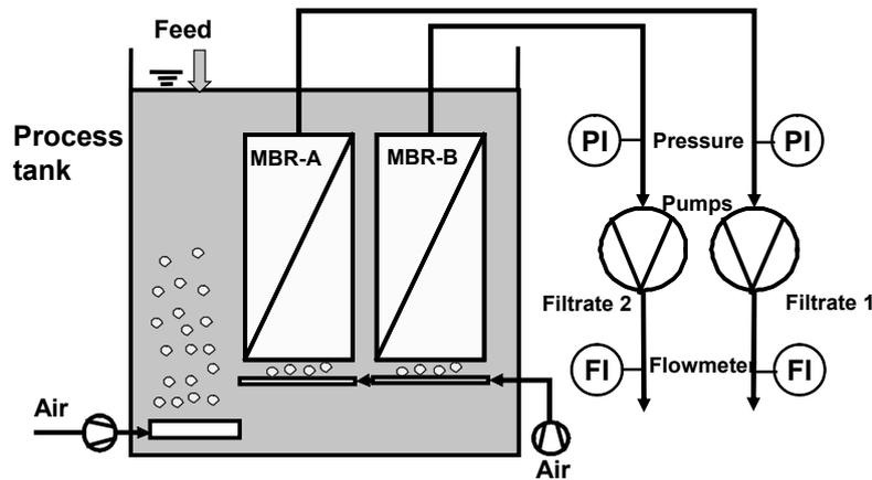
Fig. 1: Schematic illustration of the MBR pilot plant
