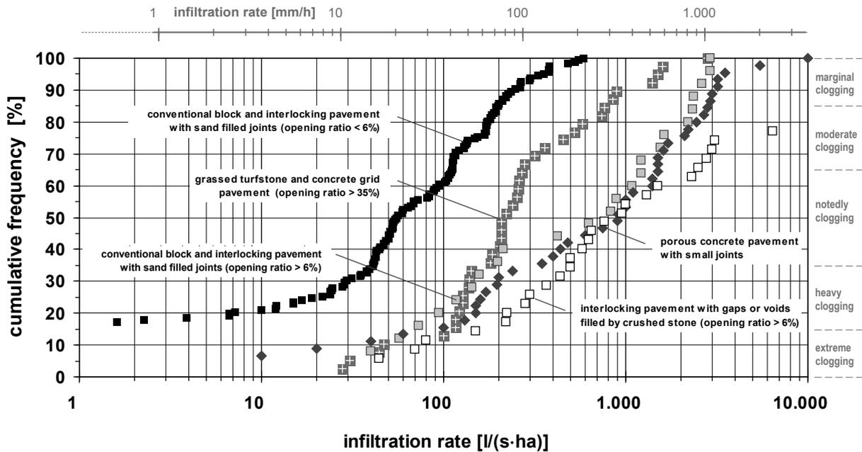
Fig 2: Cumulative frequency of final infiltration rates of common pavement types.
