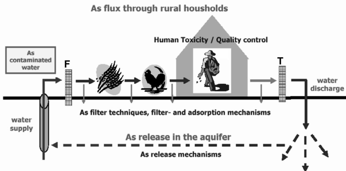
**Figure 2: Arsenic flux through rural households of the Red River Delta, Vietnam. F is representing adapted filter systems for arsenic and T is representing a treatment system for waste water. The development of F and T are aims of the presented program.**
