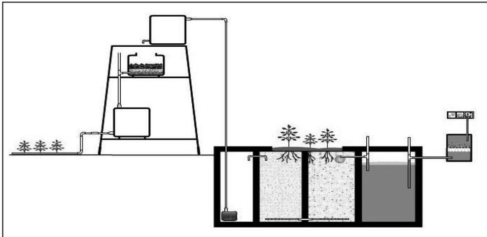
Figure (1): Grey waste water treatment plant scheme used by PHG.
