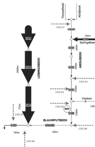
Figure 2: ratio between continuous wastewater discharge and minimum natural base flow.
