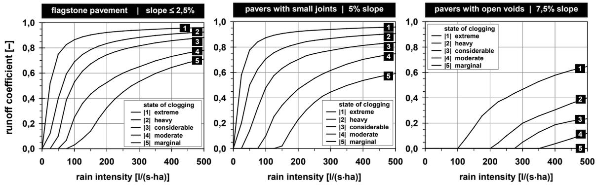
Fig. 3: Nomograms of recommended runoff coefficients for several pavement types.
