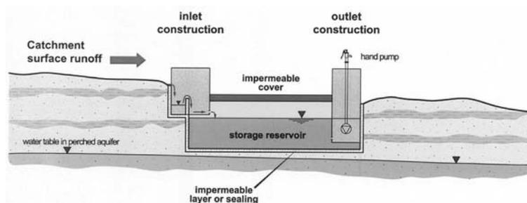
Fig. 4: General construction of a Subsurface Water Storage: Catchment surface runoff is diverted into an inlet construction and into a closed artificial subsurface reservoir.
