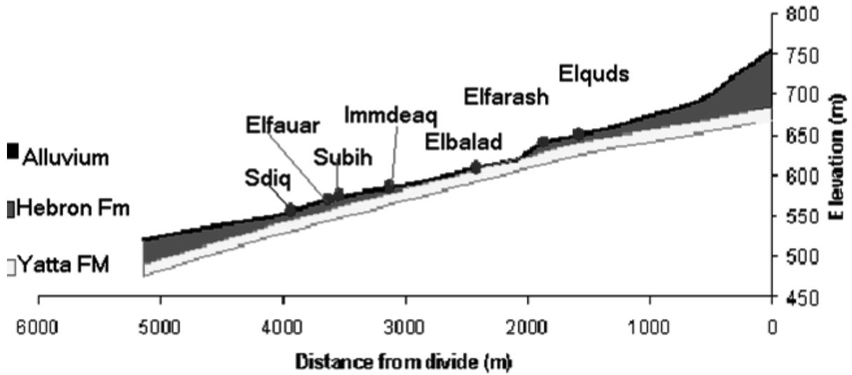
**Figure 3:** longitudinal cross section profile for the main stream in Wadi Fuqeen catchment presenting the flow direction from North to South and the perched aquifers.
