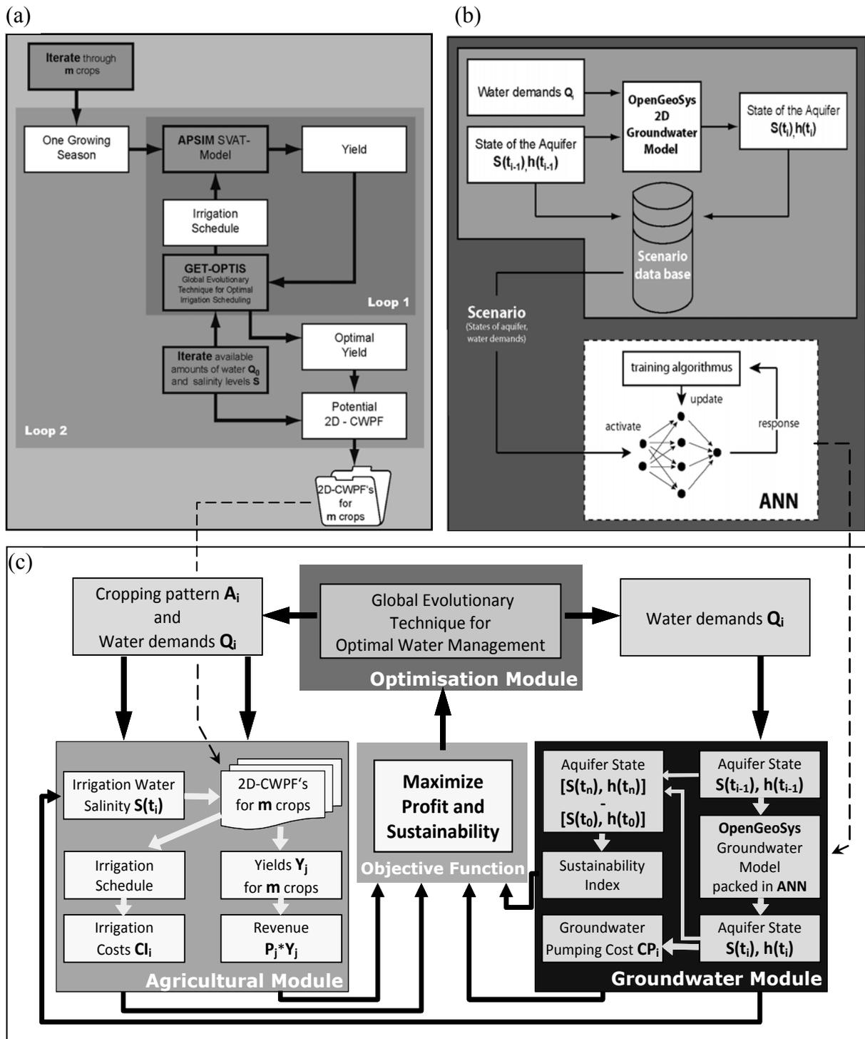
Fig. 1: Estimation procedure for the 2D crop water production functions (a) and the ANN groundwater model (b) and their linking within the optimisation framework (c)
