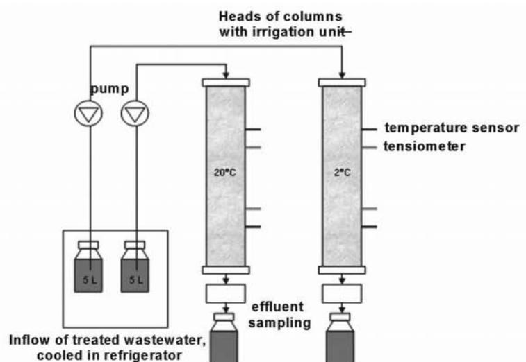
Fig. 2: Laboratory setup and scheme of the column experiment
