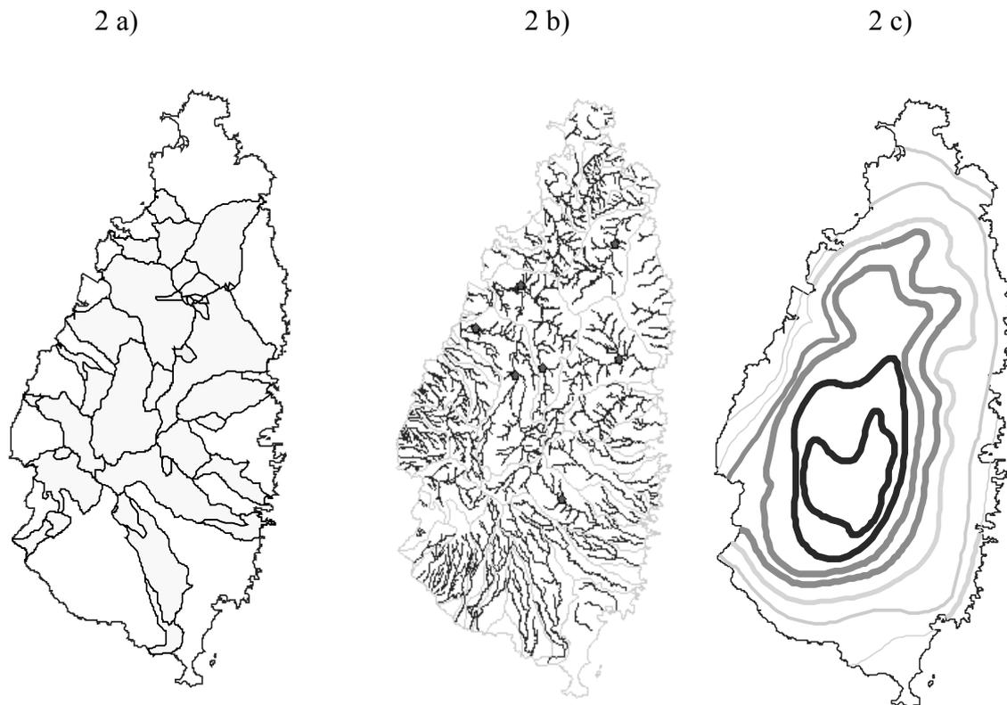
Figure 2. Examples of digitised coverages for St Lucia showing a) river catchments and water supply sub-catchments, b) streams and hydrological gauging stations, and c) annual rainfall isohyets plotted from rain gauging station data
