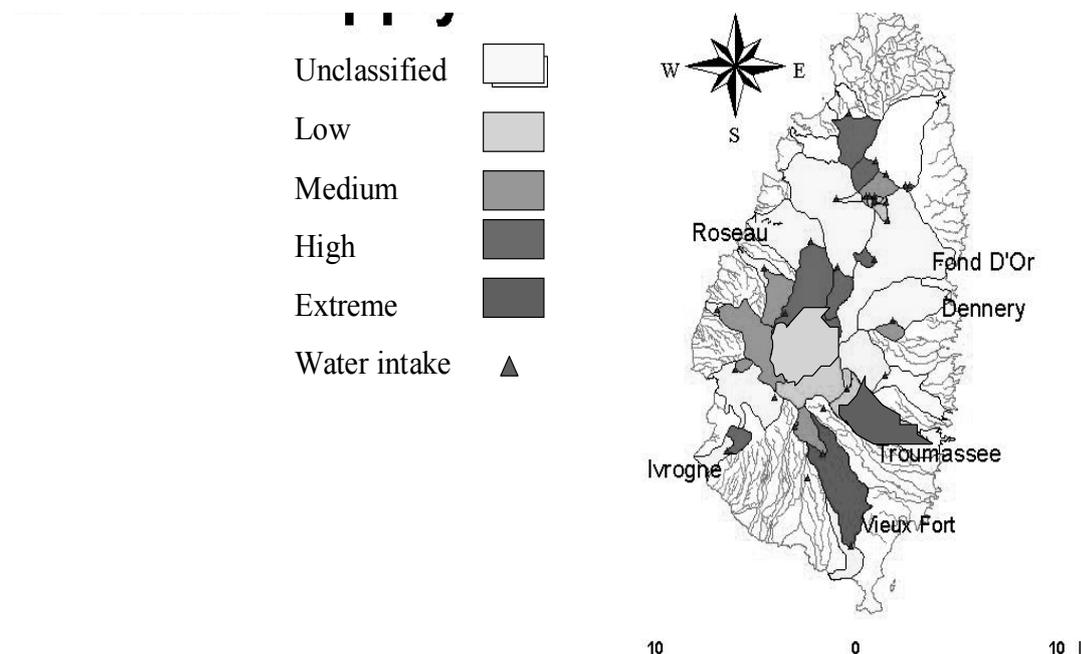
Figure 2. Preliminary classification of vulnerability of sub-catchments for water supply
