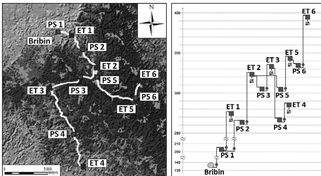
Fig. 2: Existing transmission main system (scenario A)
