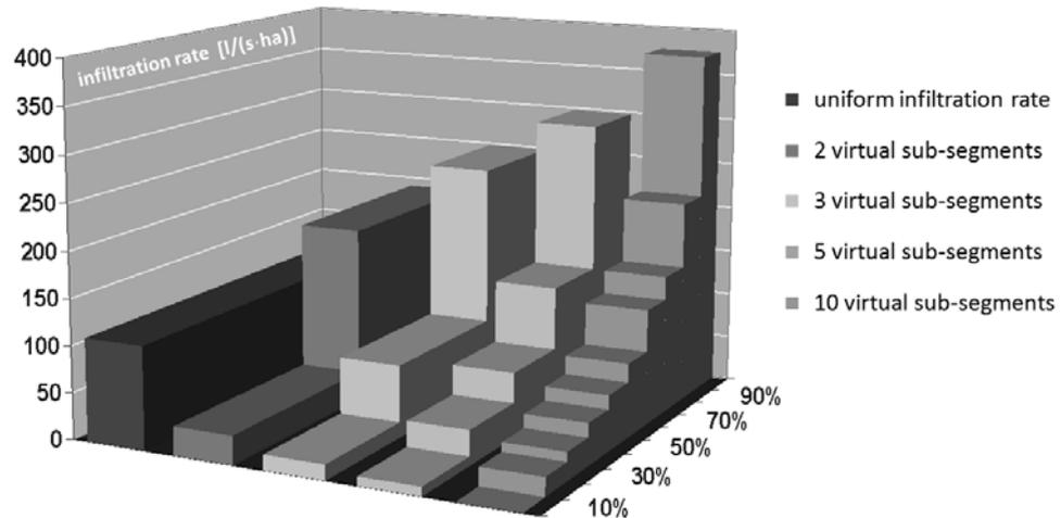
Fig. 5: Sub-division into sub-segments with varying infiltration capacity (e.g. 3 to 10 segments)
