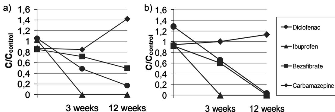
Fig. 4 Biodegradation of 4 pharmaceuticals during batch experiments with filtered raw waste water (a) and effluent from a waste water treatment plant (b)
