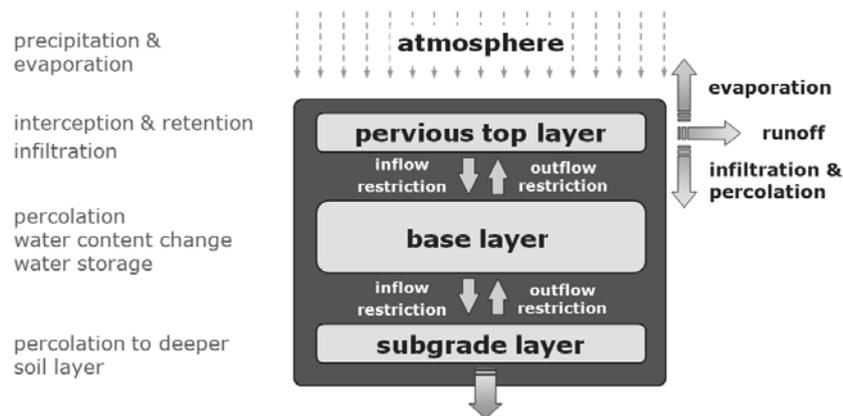
Fig. 4: Basic scheme of the bi-directional layer model and basic infiltration algorithm.
