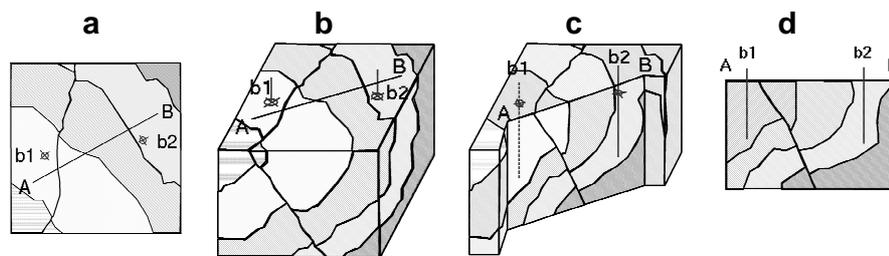
**Figure 1** Example of a 3Dto2D service: Planar profile section between endpoints A and B, with projected borehole profiles b1 and b2. (a) – location in map plane, (b) – block view of 3D model, (c) – view of profile section with part of model removed, (d) – resulting 2D profile section with the projected boreholes.
