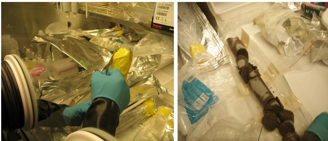
**Figure 7:** Opening of the vacuum sealed samples in  $N_2$  glovebox in the laboratory of radiochemistry, University of Helsinki.
