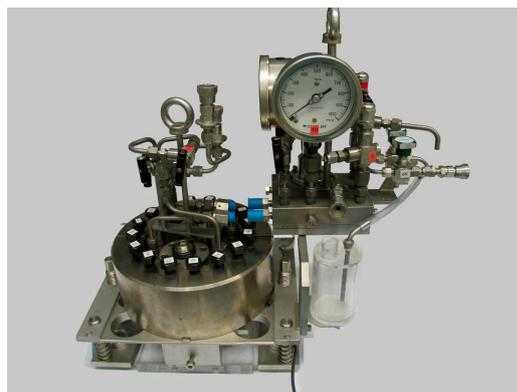
**Figure 1:** The corrosion autoclave setup (left) and a photograph of the autoclave vessel (right).
