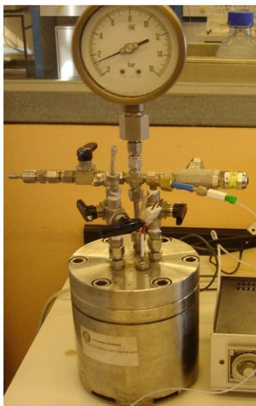
**Figure 8.** Autoclave used to perform the batch experiments.
