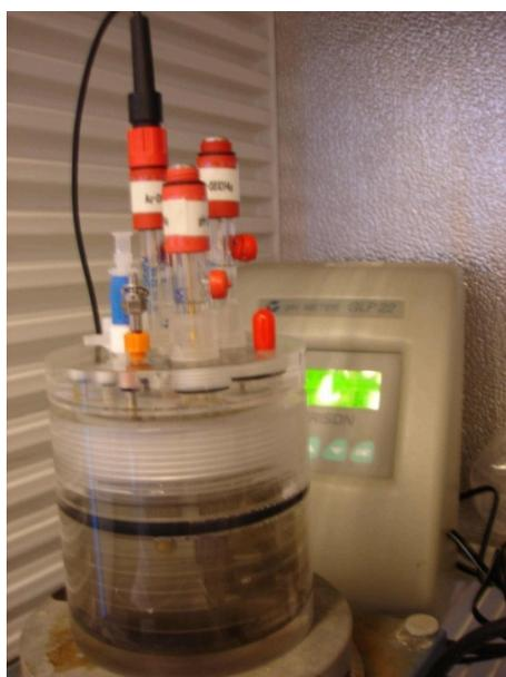
**Figure 1:** Batch reactor used for the pyrrhotite dissolution experiments.
