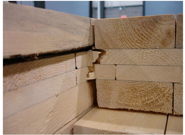
Fig. 84 Testing assembly for beams with notches (left). Failure of the reinforcing layer in short DLT beams with four plies and with notches (right)
