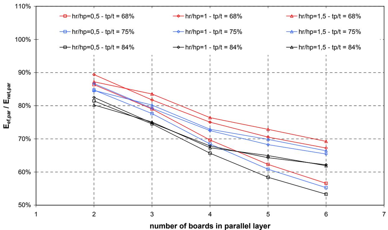
Fig. 121 Ratio between  $E_{ef}$  and  $E_{net}$  for short 5-ply DLT beams (Series 2-1)
