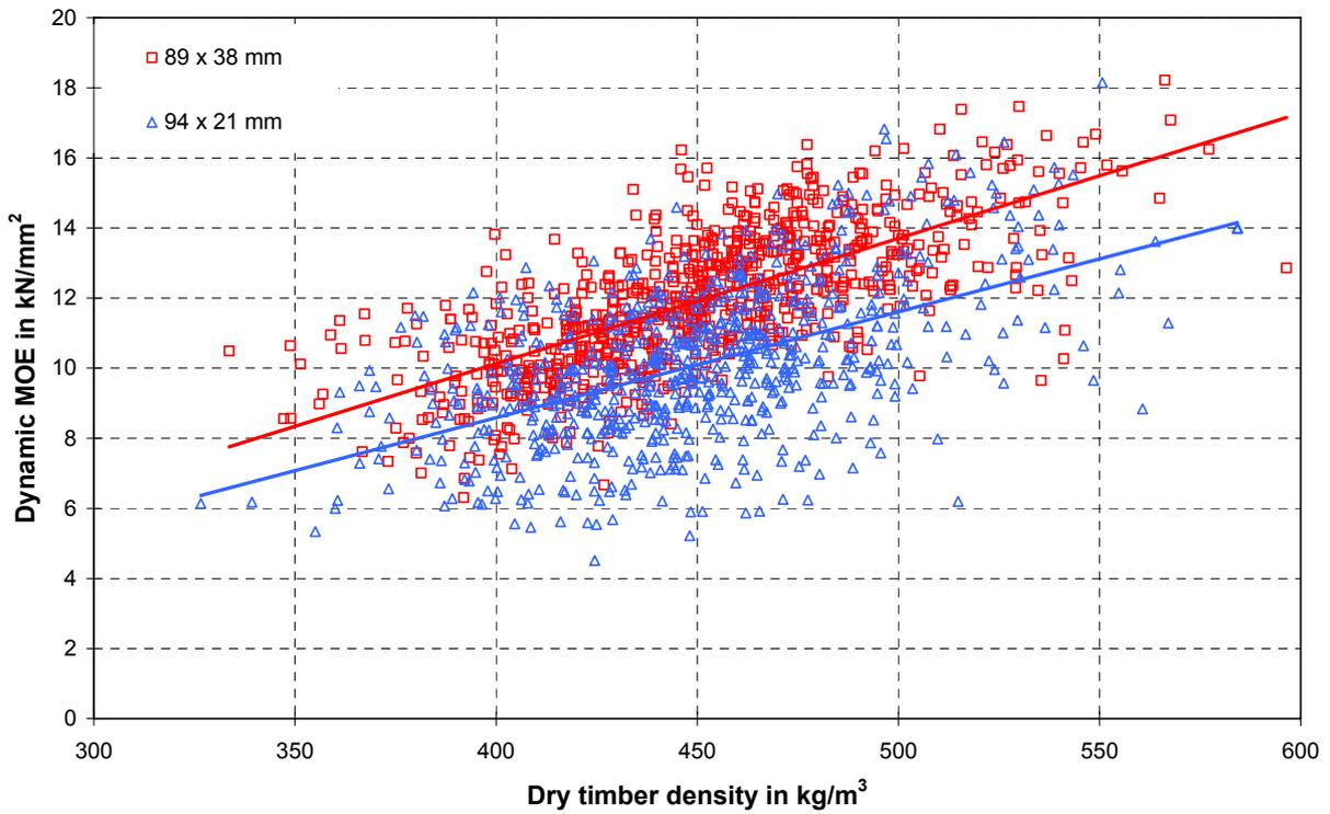
Fig. 14 Relation between the dynamic MOE and the dry timber density
