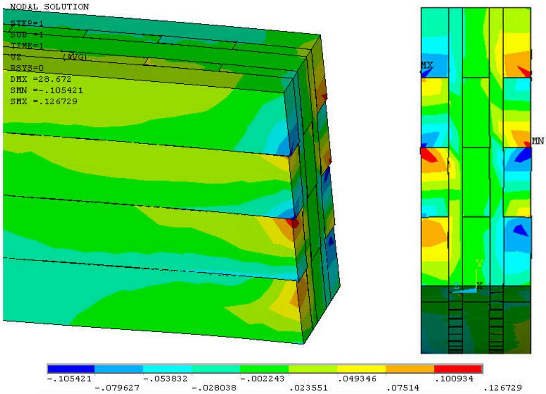
Fig. 97 Beam end with deflection in z-direction (Sp.1-1, five times distorted)
