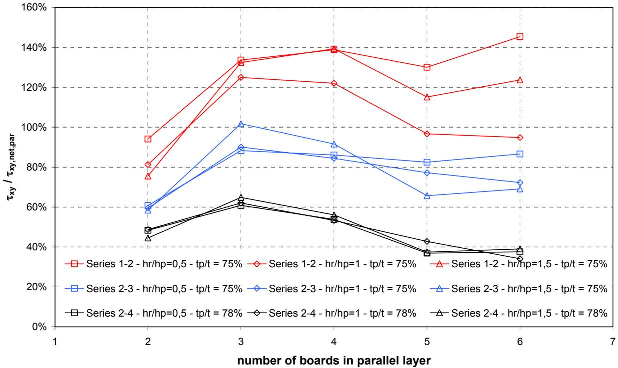
Fig. 46 Ratio between  $\tau_{xy}$  and  $\tau_{xy,net,par}$  for long beams with  $t_p/t = 75\%$  (78%)
