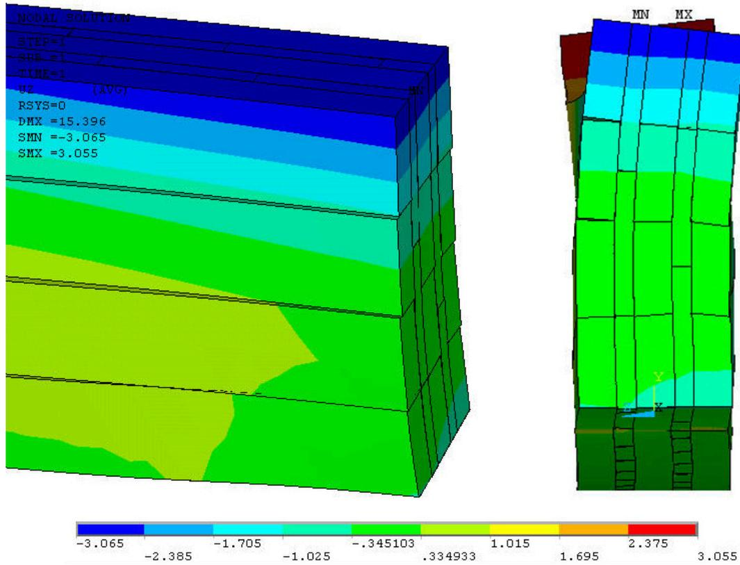
Fig. 100 Beam end with deflection in z-direction (Sp.2-1, five times distorted)
