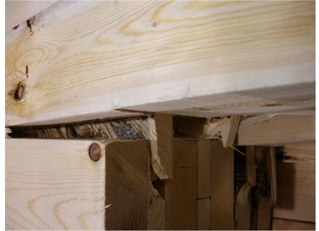
Fig. 83 Failure of the reinforcing layer in short DLT beams with five plies and with notches
