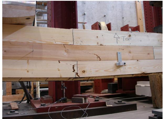
Fig. 78 DLT beam with four plies before and after bending failure
