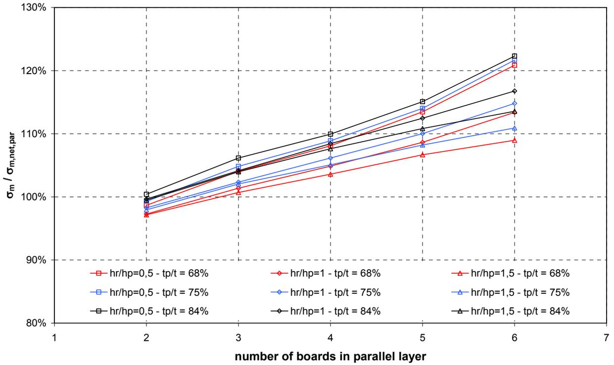
Fig. 126 Ratio between  $\sigma_m$  and  $\sigma_{m,net}$  for short 5-ply CLT beams (Series 1-1)
