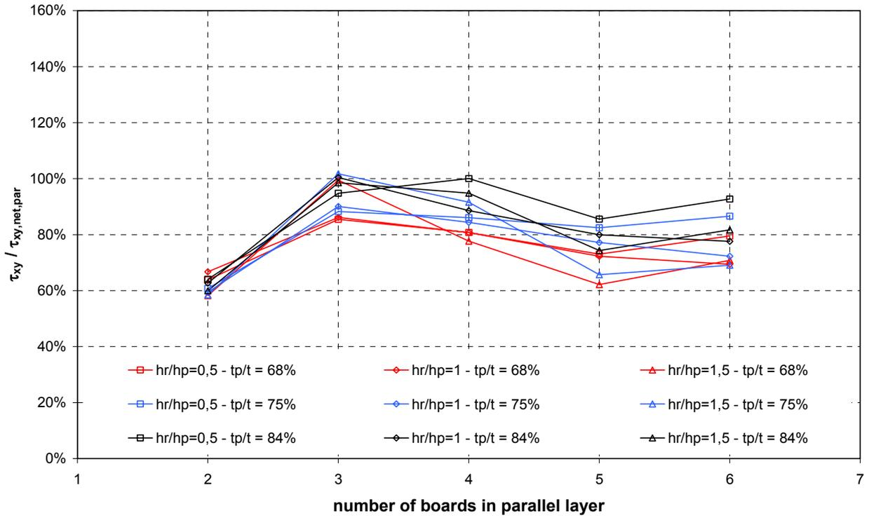
Fig. 136 Ratio between  $\tau_{xy}$  and  $\tau_{xy,net}$  for long 5-ply DLT beams (Series 2-3)
