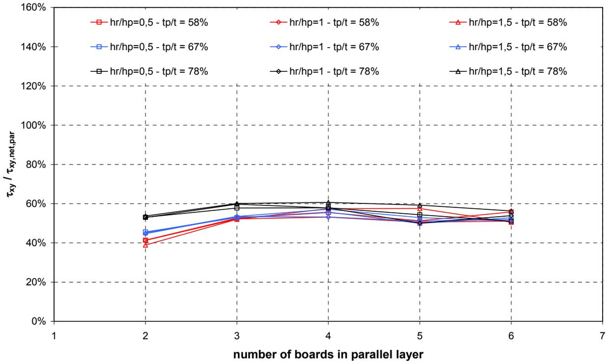
Fig. 134 Ratio between  $\tau_{xy}$  and  $\tau_{xy,net}$  for short 4-ply DLT beams (Series 2-2)
