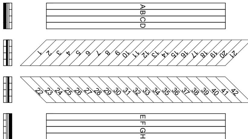
Fig. 50 Species 2.2 – Short beam with 45° reinforcing layers - 4 ply
