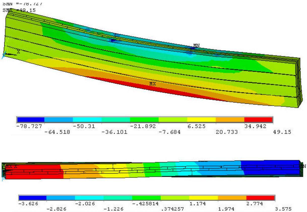
Fig. 104 Bending stresses (top) and deflection in z-direction (bottom) (five times distorted)
