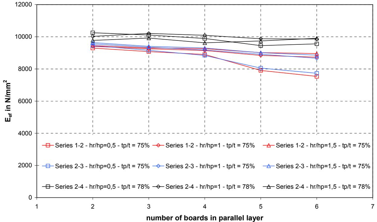
Fig. 40  $E_{ef}$  for long beams with  $t_p/t = 75\%$  (78%)
