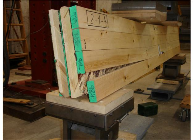
Fig. 71 Typical failure for DLT beams with five plies
