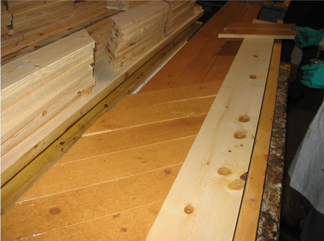
Fig. 59 Species 2.5 – Diagonal reinforcing layer with a PRF glue surface
