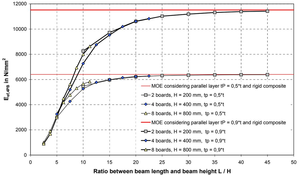
Fig. 25 Effective MOE for CLT beams (90°) with bonding stiffness  $K = 6 \text{ N/mm}^3$
