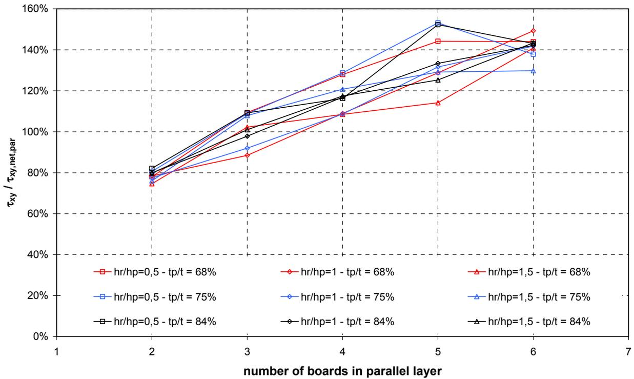
Fig. 132 Ratio between  $\tau_{xy}$  and  $\tau_{xy,net}$  for short 5-ply CLT beams (Series 1-1)
