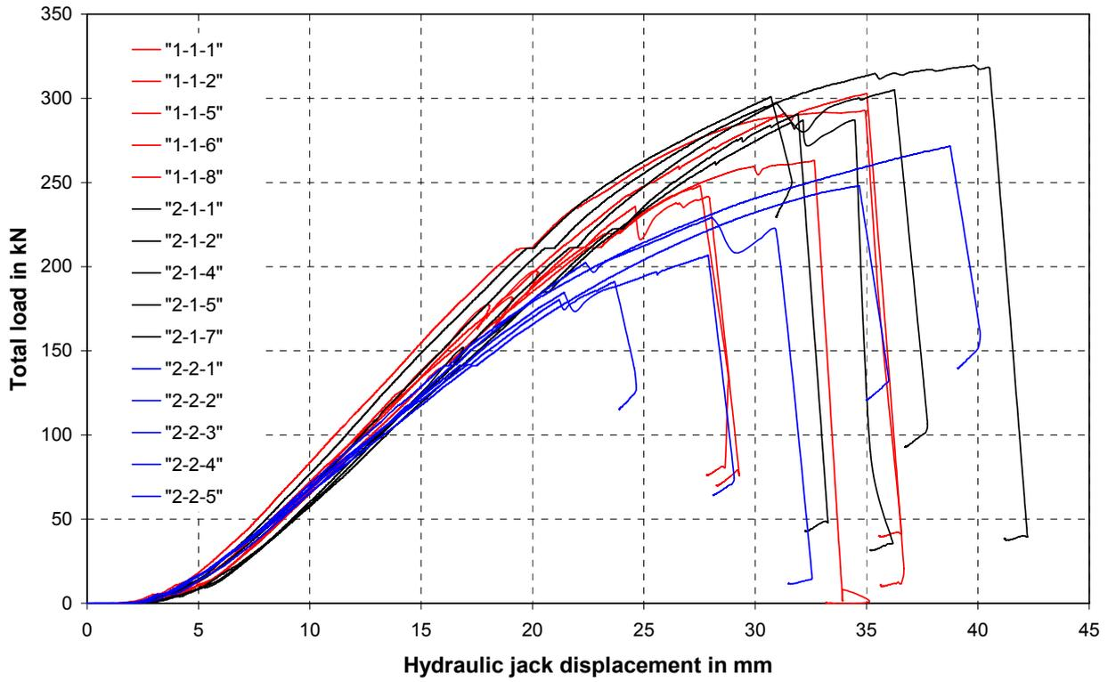
Fig. 67 Load-displacement behaviour for short beams
