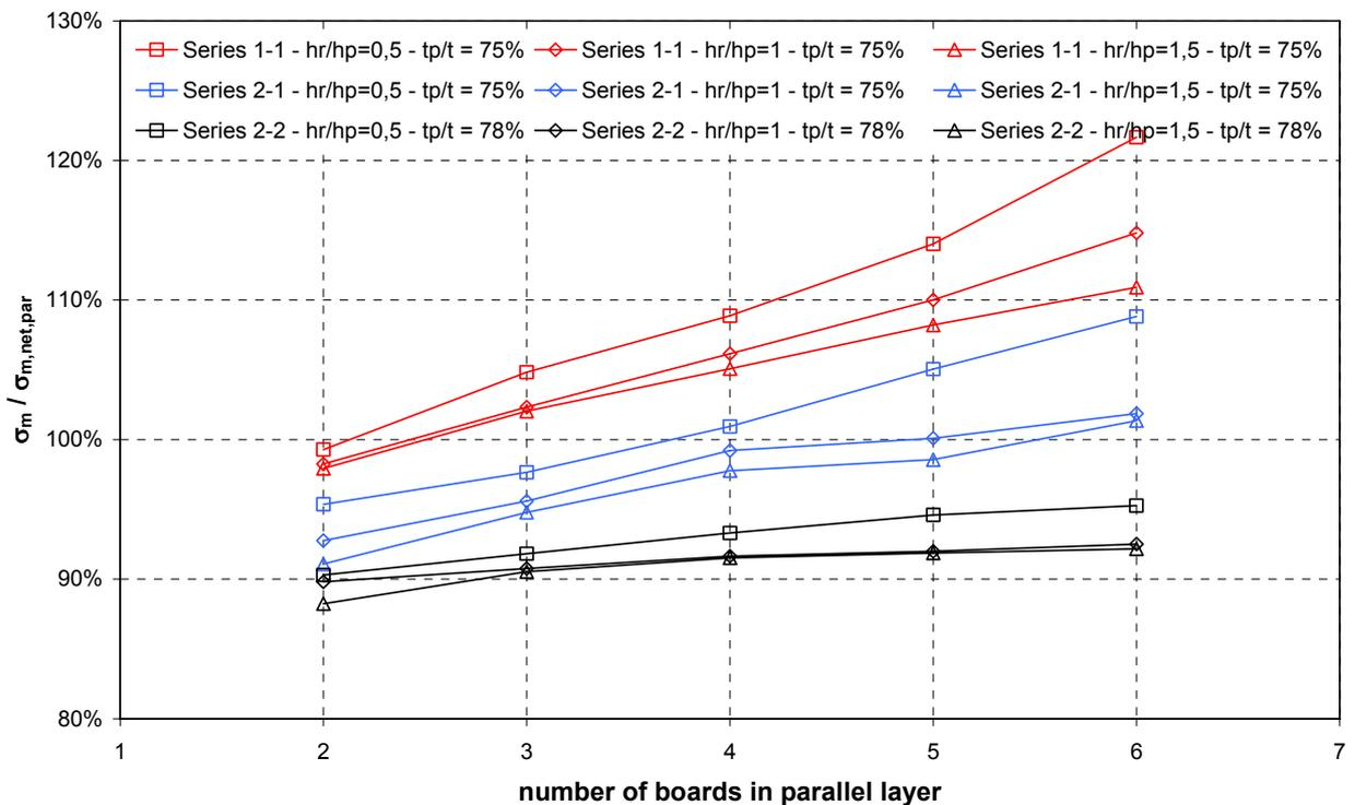
Fig. 43 Ratio between  $\sigma_m$  and  $\sigma_{m,net}$  for short beams with  $t_p/t = 75\%$  (78%)
