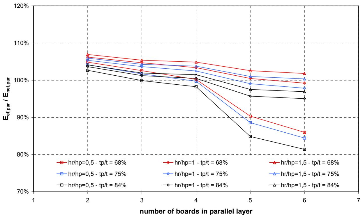
Fig. 123 Ratio between  $E_{ef}$  and  $E_{net}$  for long 5-ply CLT beams (Series 1-2)
