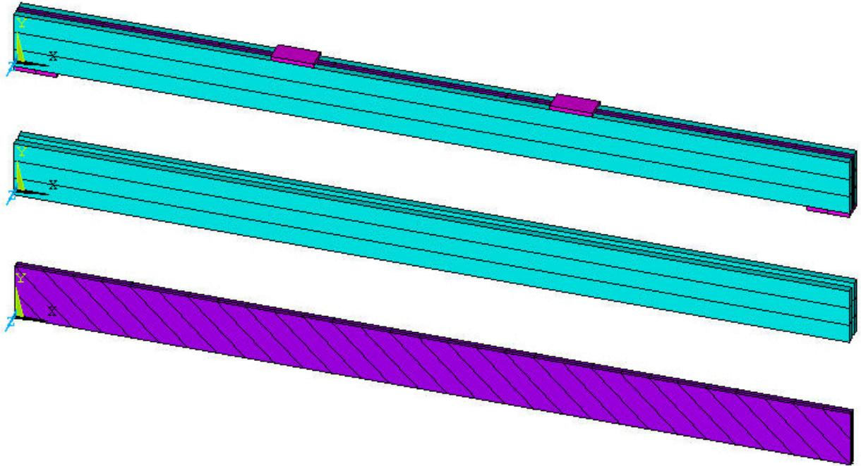
Fig. 111 FE system for specimen 2-4 (long DLT with four plies)
