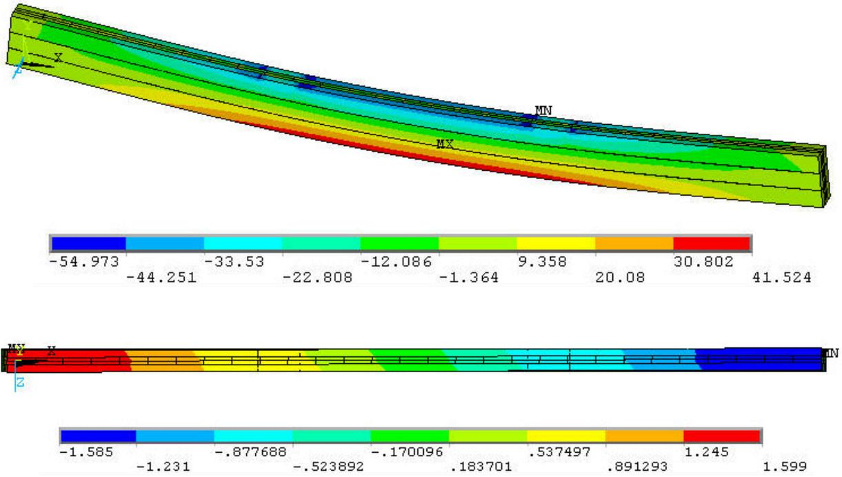
Fig. 113 Bending stresses (top) and deflection in z-direction (bottom) (three times distorted)
