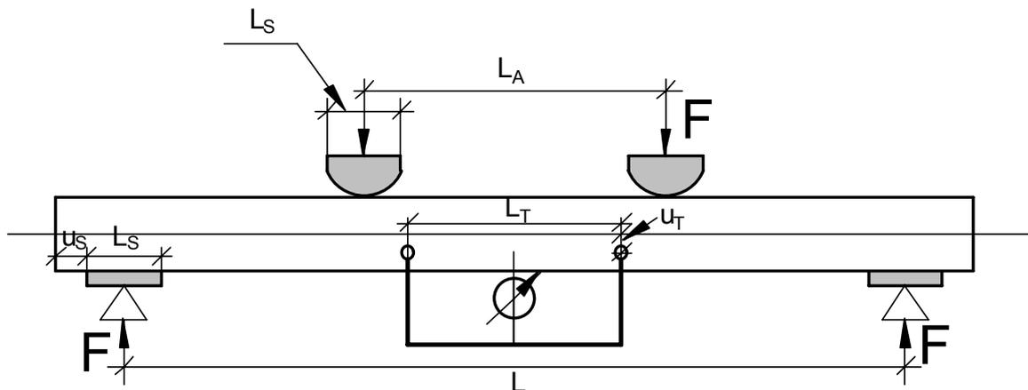
Fig. 17 Test set-up for long beams
