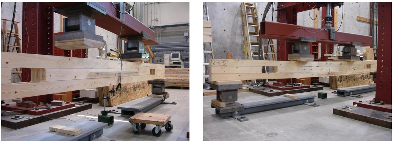
Fig. 88 Testing assembly for beams with holes before testing (left) and before failure (right)
