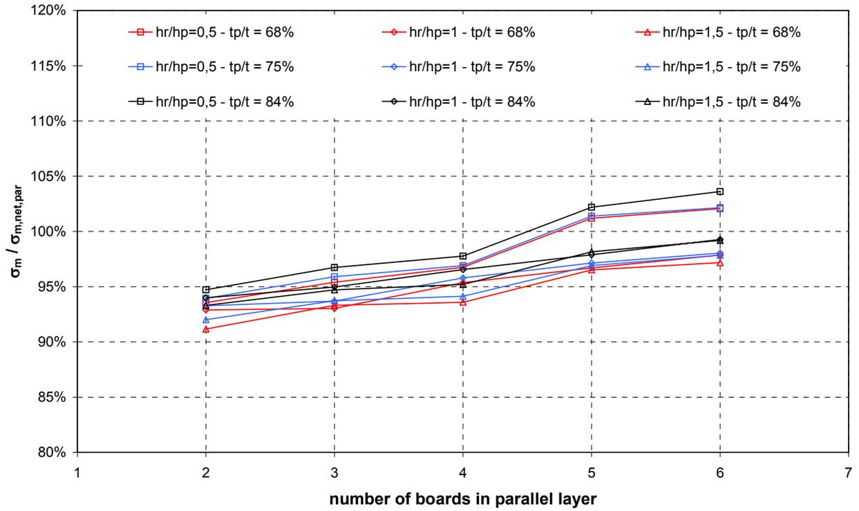
Fig. 130 Ratio between  $\sigma_m$  and  $\sigma_{m,net}$  for long 5-ply DLT beams (Series 2-3)
