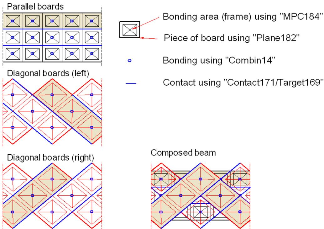
Fig. 29 Plane model considering contact between boards, orthotropic material properties and bonding
