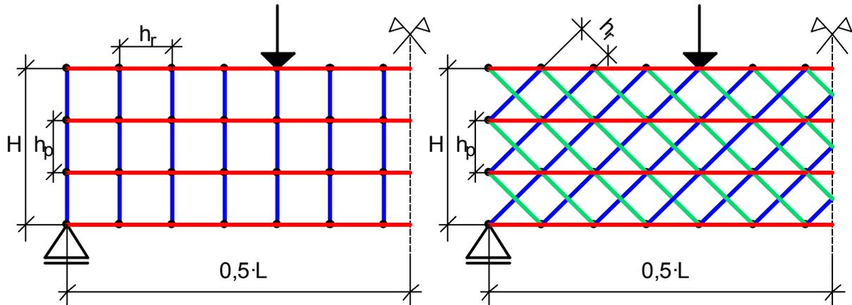
Fig. 22 Grid Model for CLT and DLT beams
