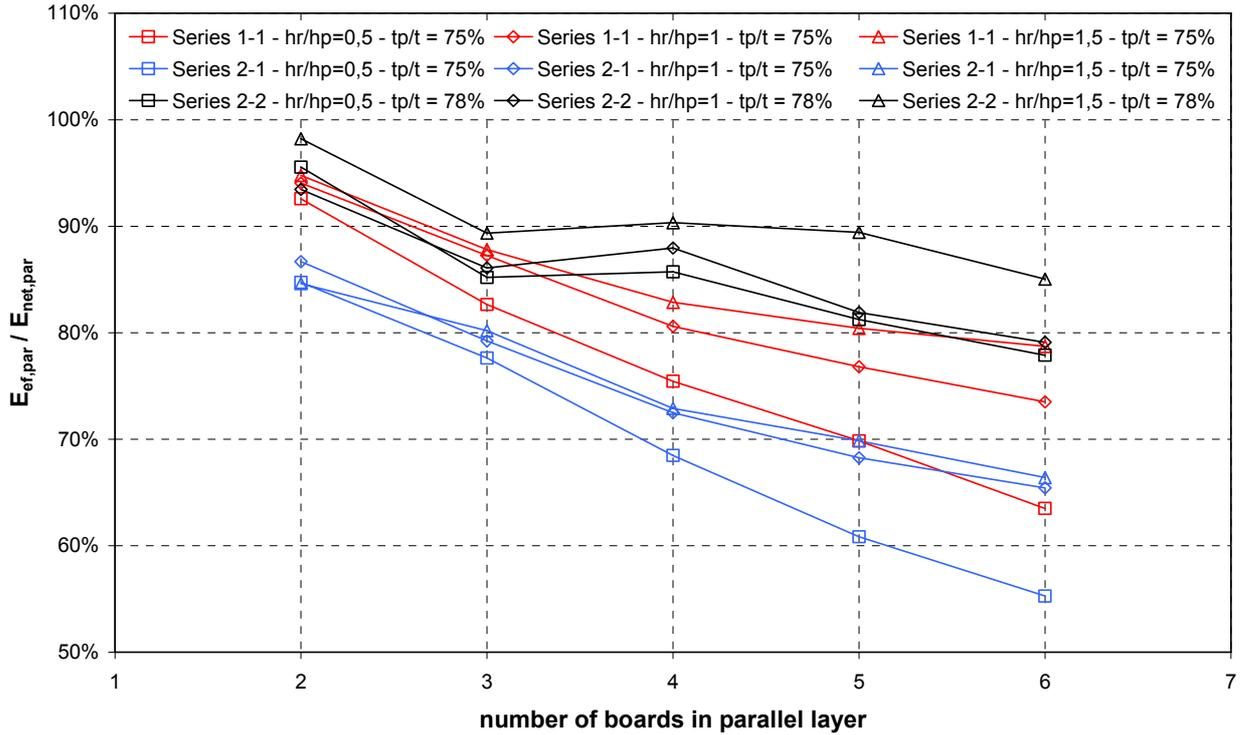
Fig. 41 Ratio between  $E_{ef}$  and  $E_{net}$  for short beams with  $t_p/t = 75\%$  (78%)
