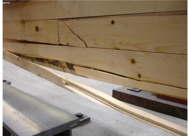
Fig. 77 Typical failure for long beams displayed as an example on a DLT beam with five plies
