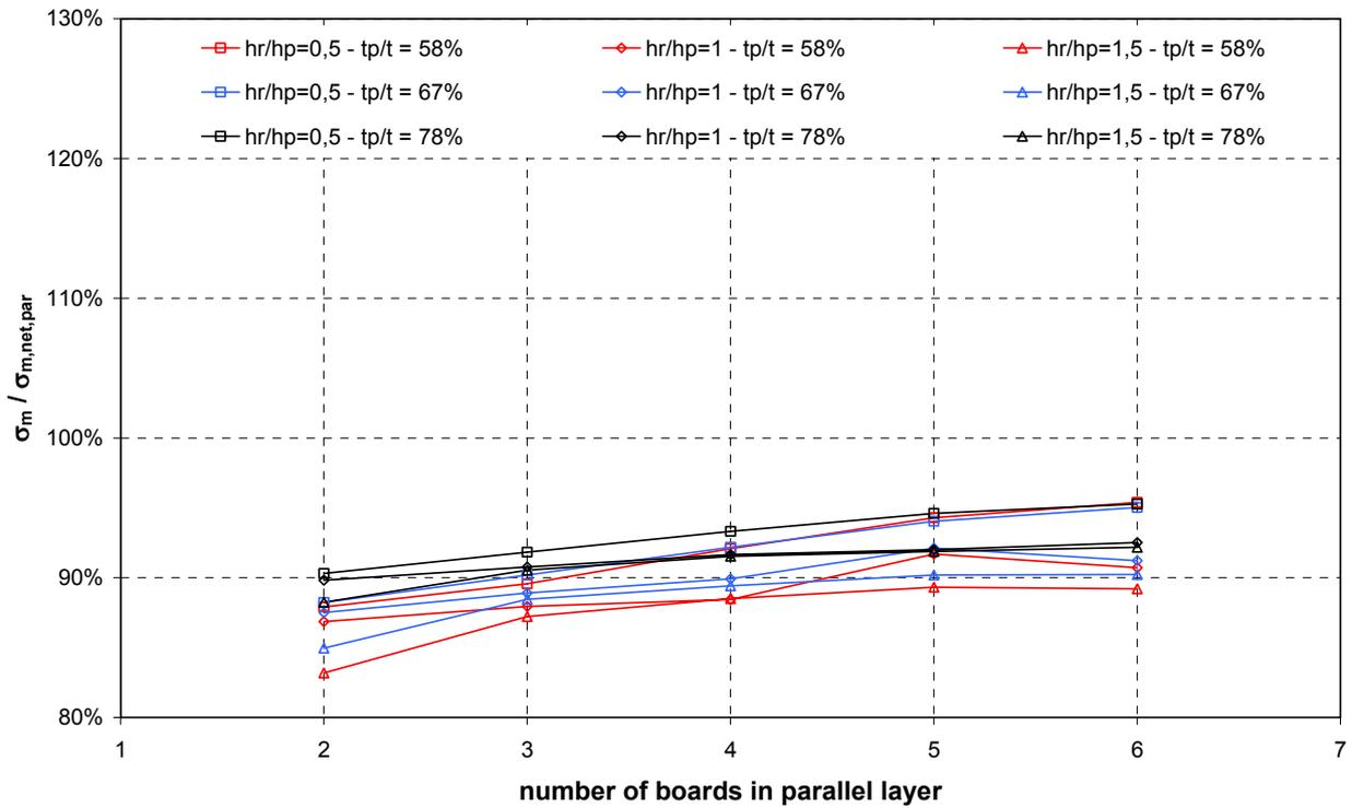
Fig. 128 Ratio between  $\sigma_m$  and  $\sigma_{m,net}$  for short 4-ply DLT beams (Series 2-2)
