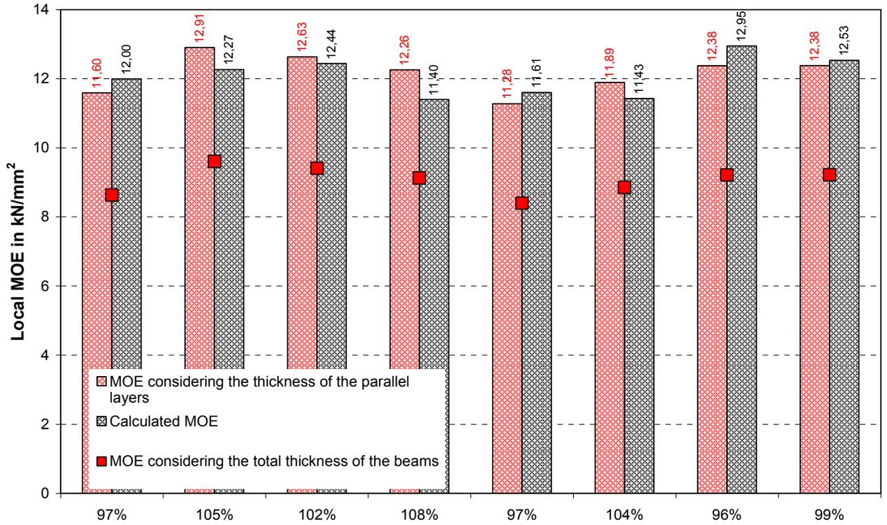
Fig. 94  $E_{0,net}$  ( $E_0$ ) versus  $E_{cal}$  for specimens 2-3 (long DLT with five plies)
