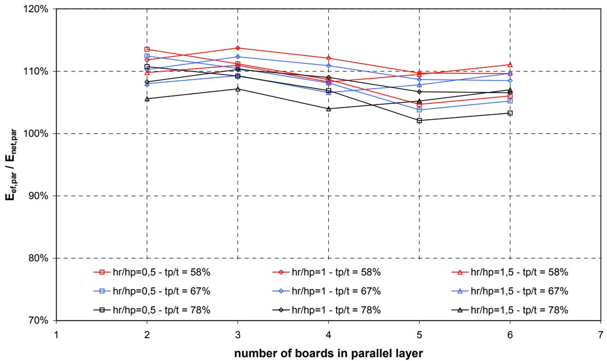
Fig. 125 Ratio between  $E_{ef}$  and  $E_{net}$  for long 4-ply DLT beams (Series 2-4)
