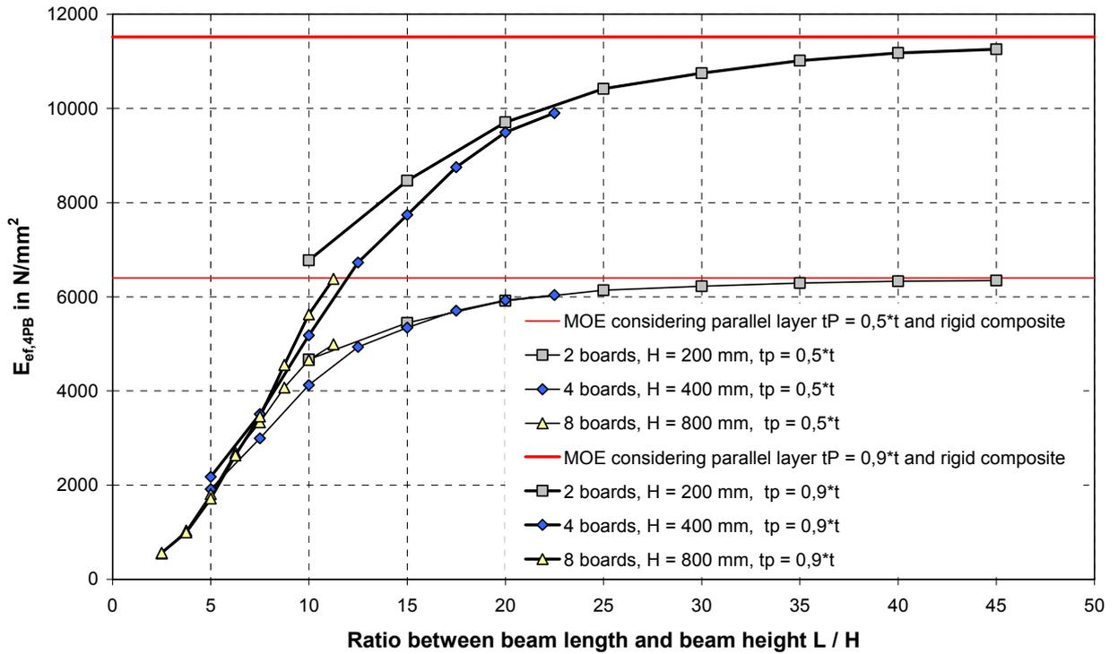
Fig. 24 Effective MOE for CLT beams ( $90^\circ$ ) with bonding stiffness  $K = 3 \text{ N/mm}^3$
