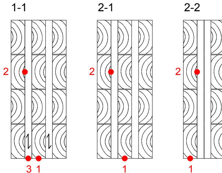
Fig. 31 Path definition for short beams (path 1 for  $\sigma_x$ , path 2 for  $\tau_{xy}$ , path 3 for  $\sigma_y$ )
