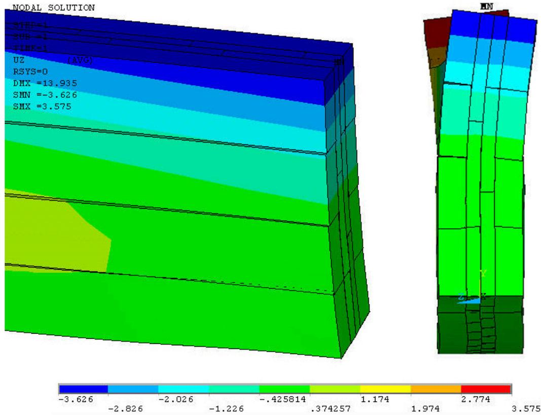
Fig. 103 Beam end with deflection in z-direction (Sp.2-2, five times distorted)
