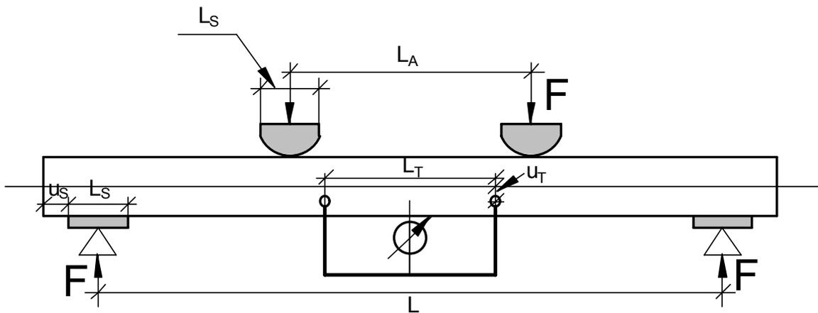
Fig. 16 Test set-up for short beams
