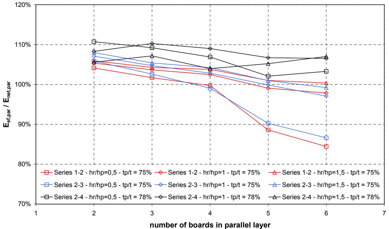
Fig. 42 Ratio between  $E_{ef}$  and  $E_{net}$  for long beams with  $t_p/t = 75\%$  (78%)
