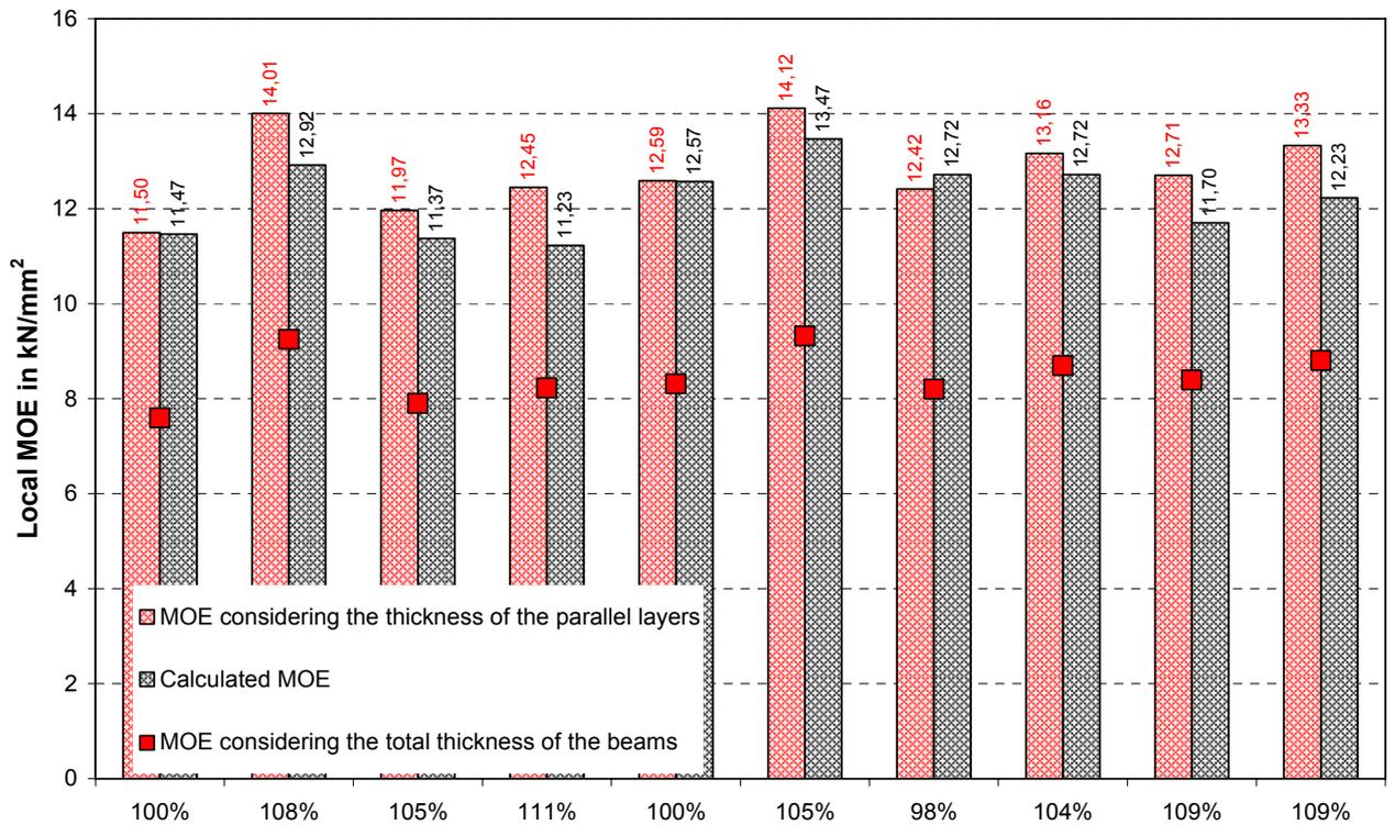
Fig. 95  $E_{0,net}$  ( $E_0$ ) versus  $E_{cal}$  for specimens 2-4 (long DLT with four plies)
