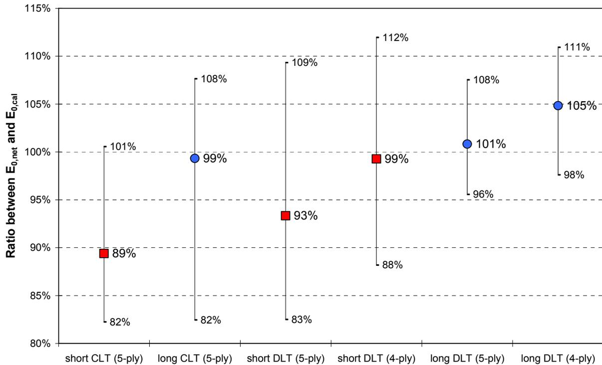
Fig. 20  $E_{0,net}$  versus  $E_{0,cal}$  for each beam type
