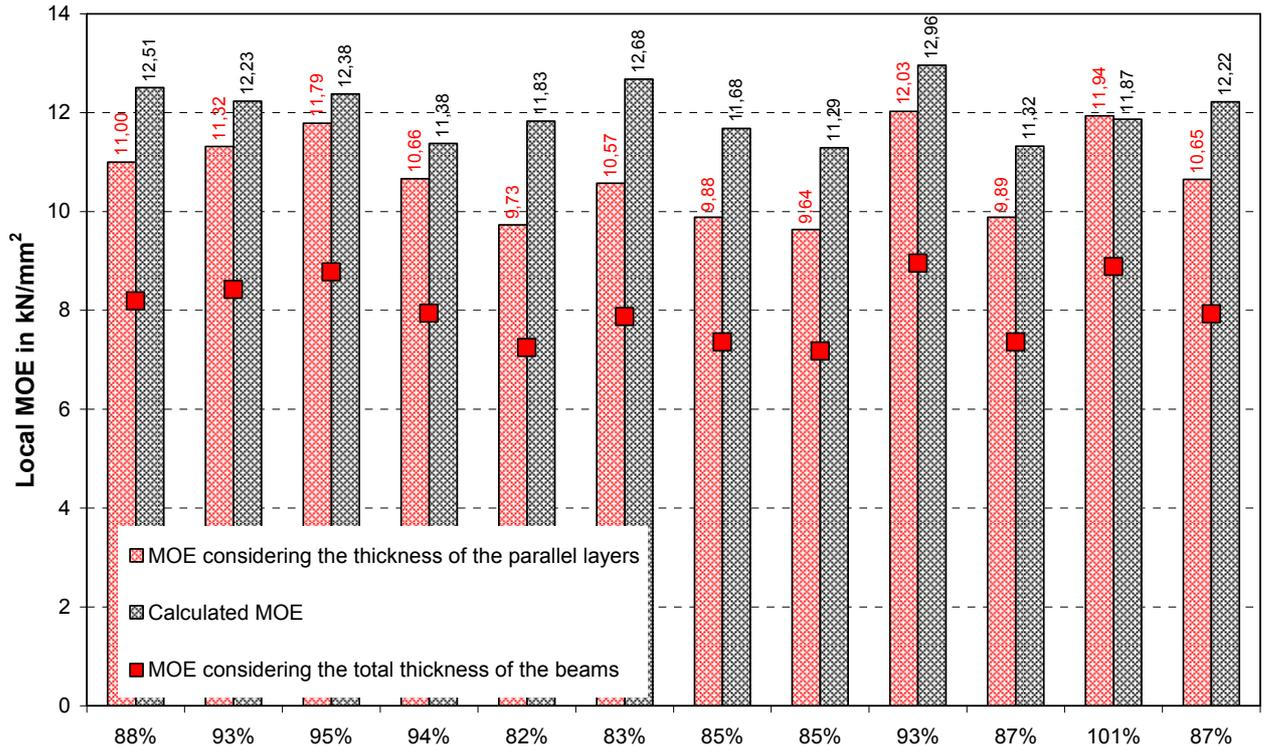
Fig. 90  $E_{0,net}$  ( $E_0$ ) versus  $E_{cal}$  for specimens 1-1 (short CLT with five plies)
