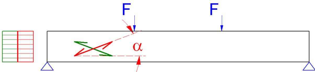
Fig. 7 Model to determine the relationship between the local MOE and inclination
