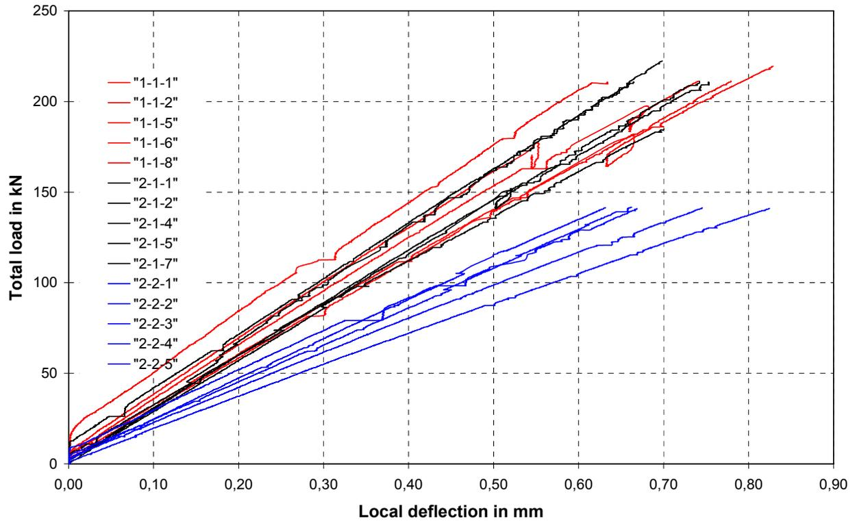
Fig. 69 Load-displacement behaviour for short beams
