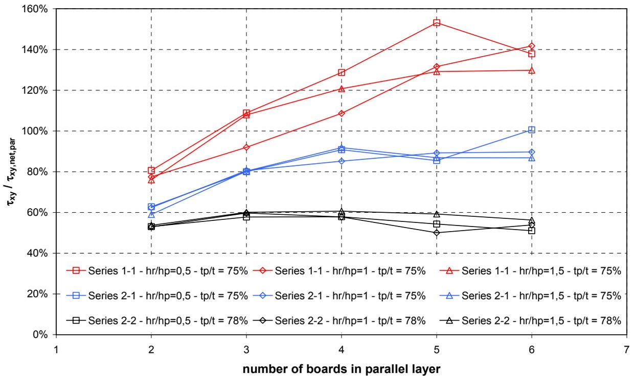
Fig. 45 Ratio between  $\tau_{xy}$  and  $\tau_{xy,net}$  for short beams with  $t_p/t = 75\%$  (78%)
