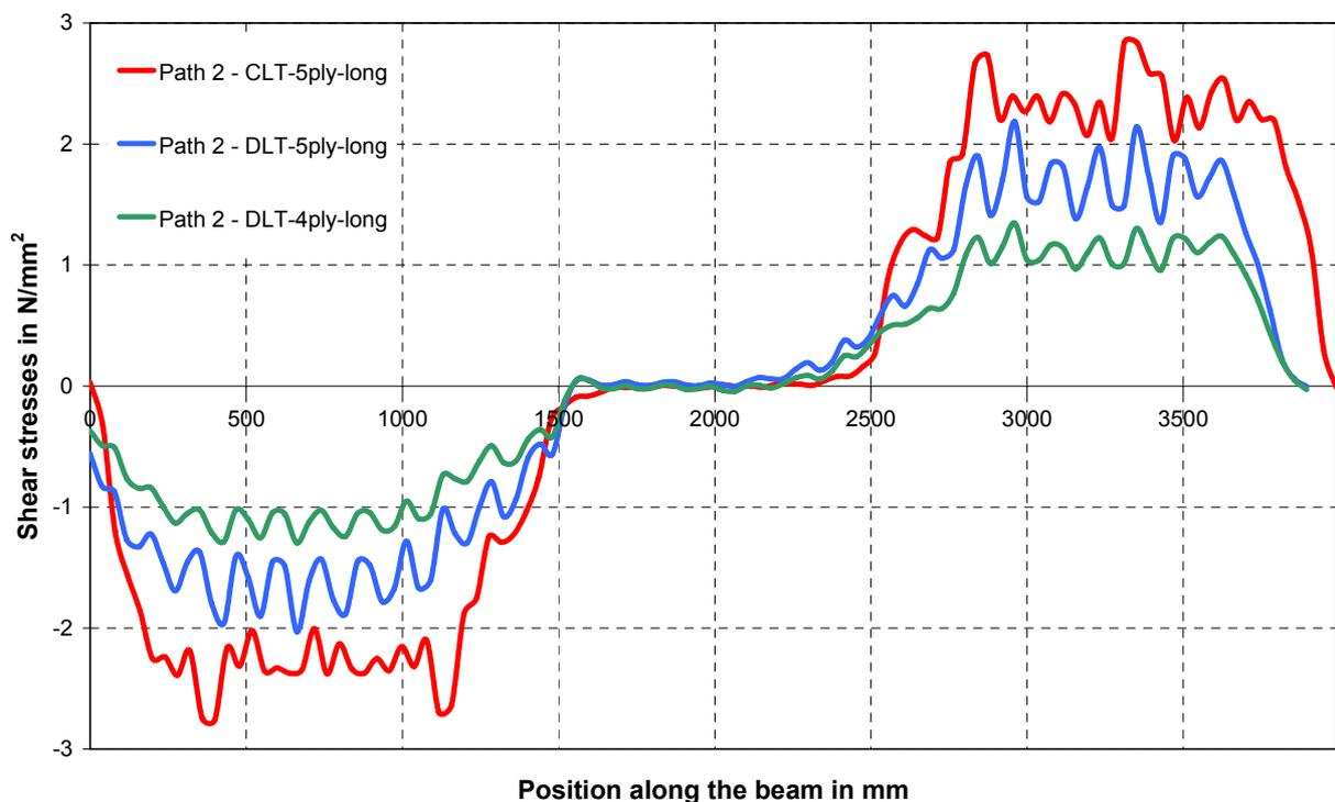
Fig. 36 Distribution of shear stresses  $\tau_{xy}$  along path 2 for long beams
