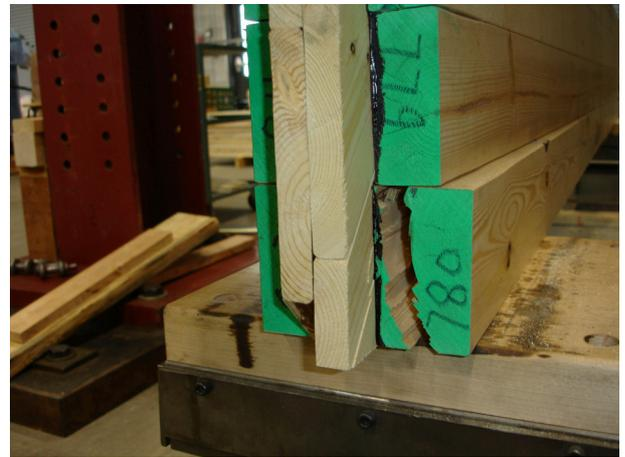
Fig. 72 Test set-up and typical failure for DLT beams with four plies
