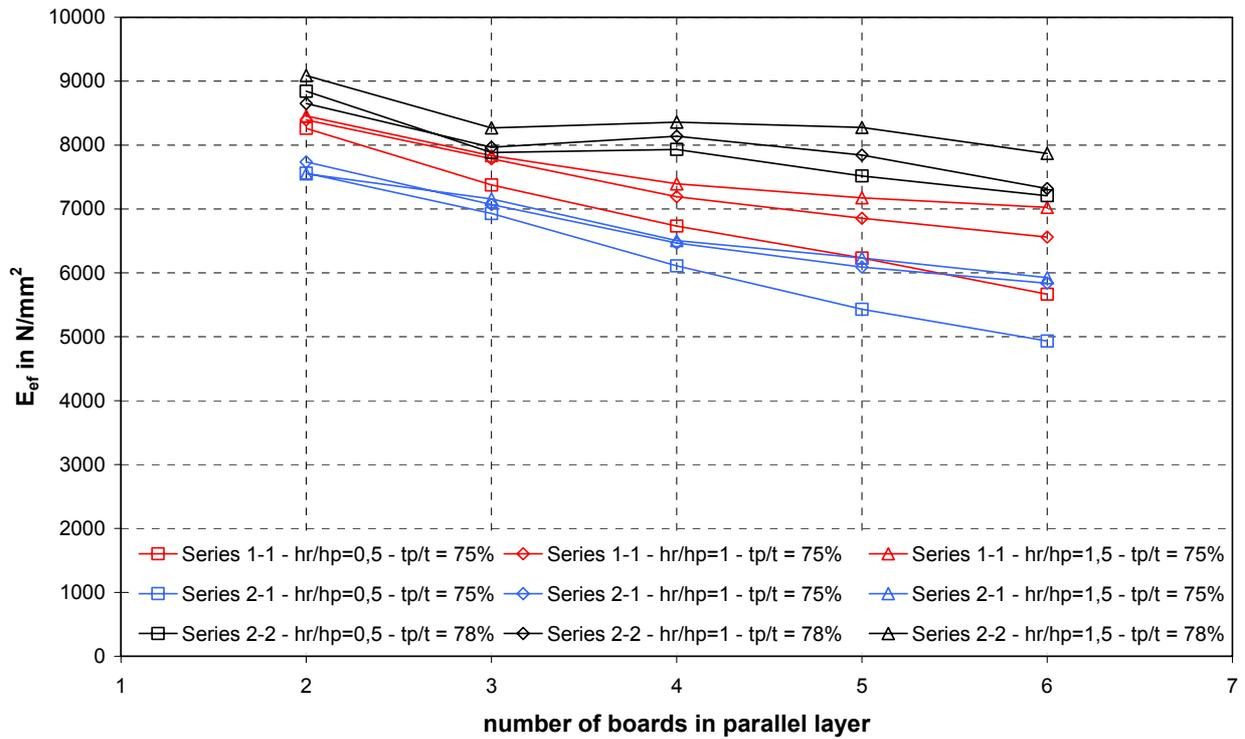
Fig. 39  $E_{ef}$  for short beams with  $t_p/t = 75\%$  (78%)
