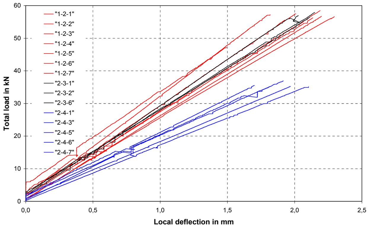
Fig. 87 Load-displacement behaviour for long beams with holes
