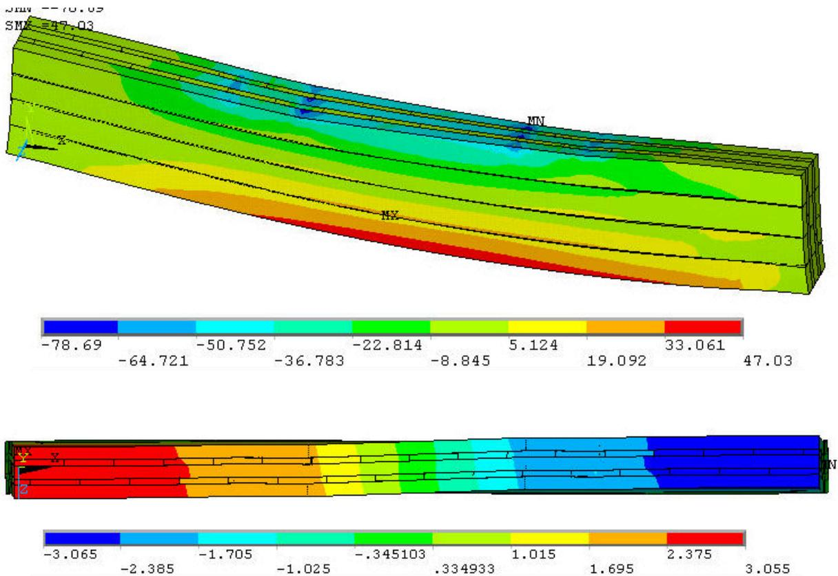
Fig. 101 Bending stresses (top) and deflection in z-direction (bottom) (five times distorted)
