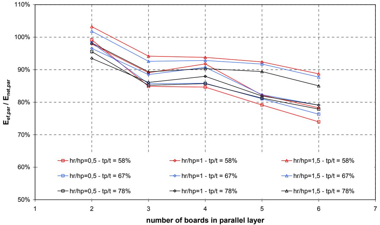
Fig. 122 Ratio between  $E_{ef}$  and  $E_{net}$  for short 4-ply DLT beams (Series 2-2)
