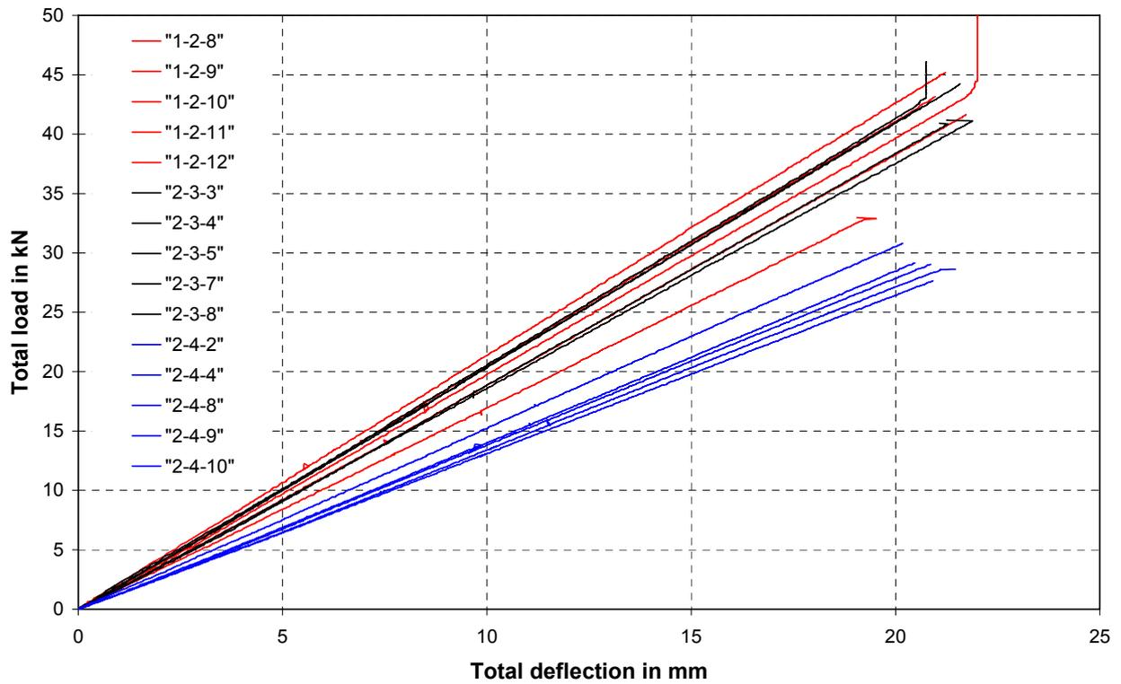
Fig. 74 Load-displacement behaviour for long beams
