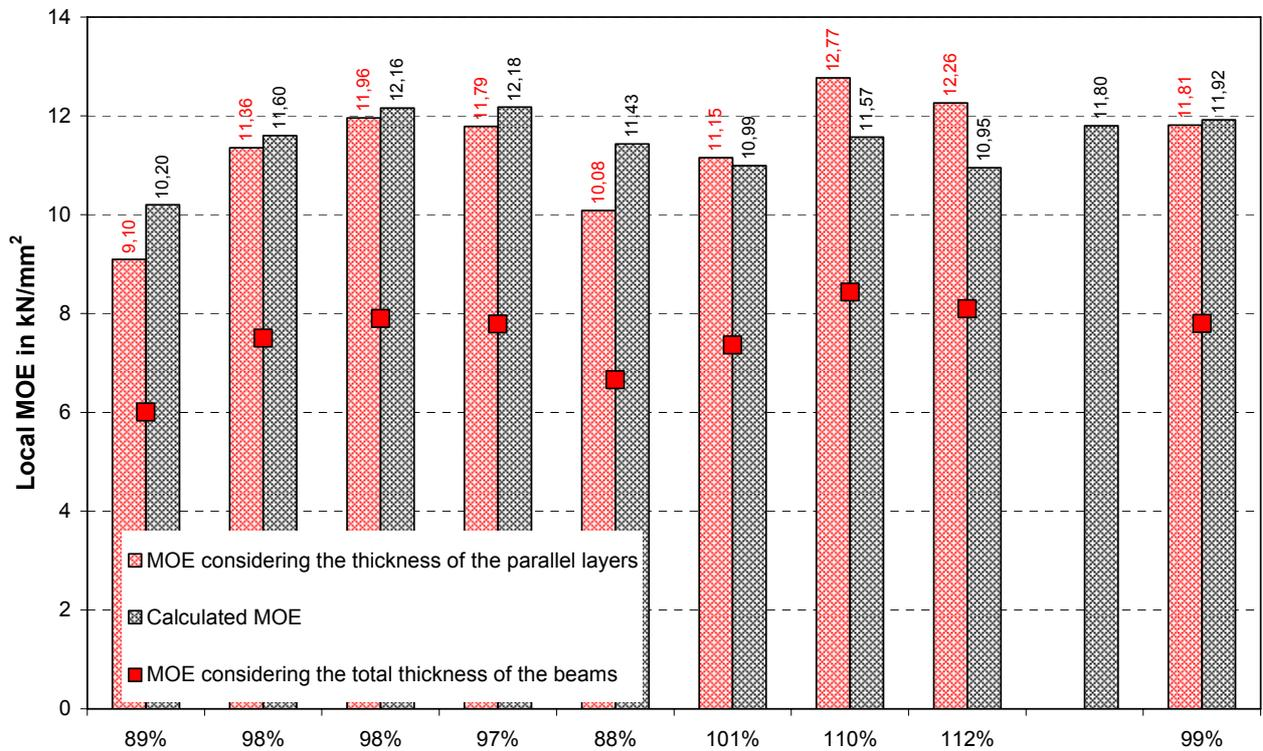
Fig. 93  $E_{0,net}$  ( $E_0$ ) versus  $E_{cal}$  for specimens 2-2 (short DLT with four plies)
