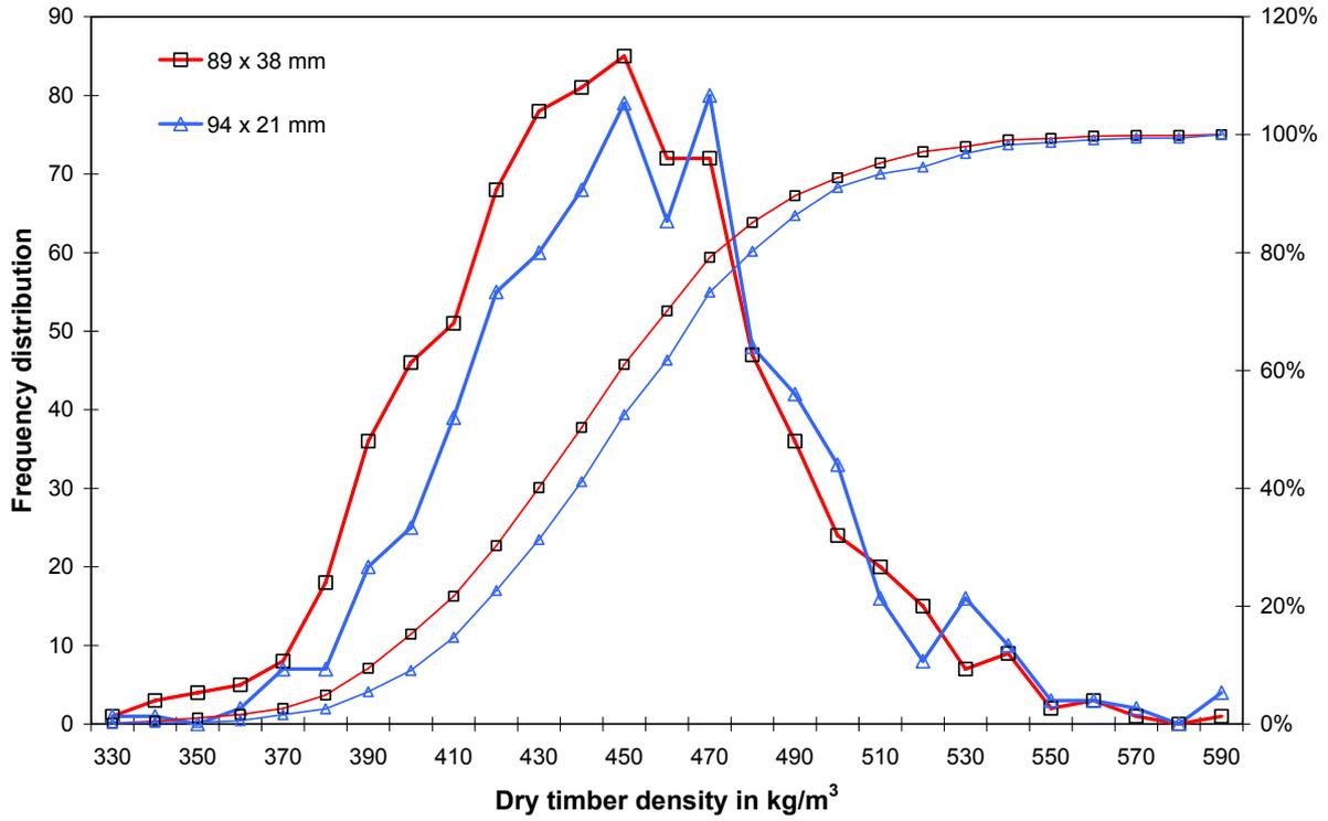
Fig. 13 Frequency distribution for the dry timber density
