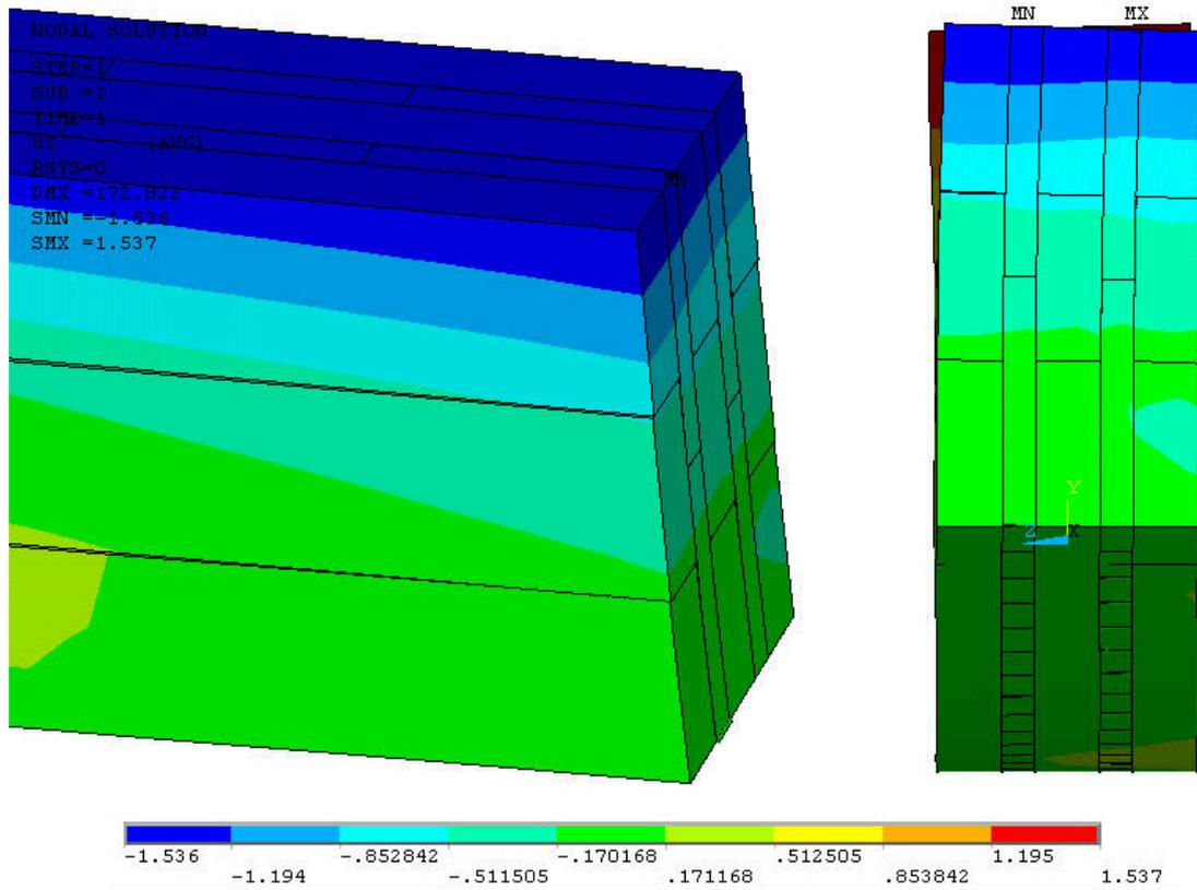
Fig. 109 Beam end with deflection in z-direction (Sp.2-3, three times distorted)
