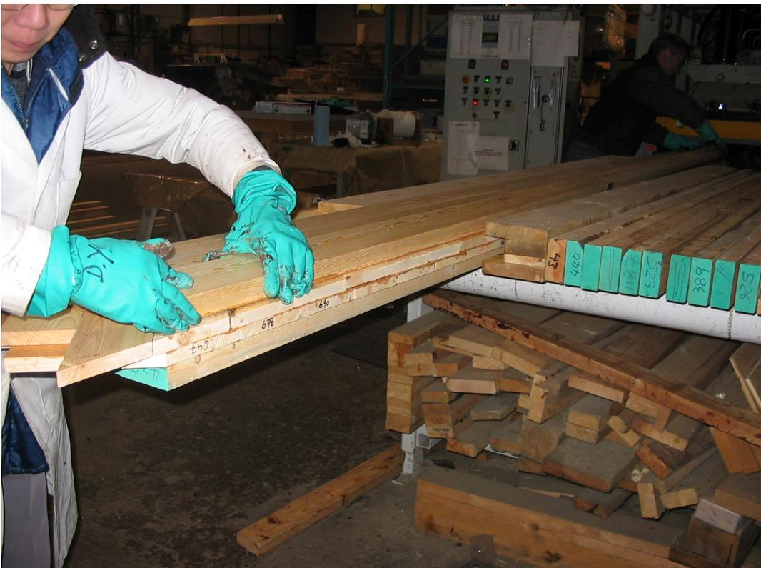
Fig. 64 Species 2.4 – Beam in a fixing frame short before on the way to the press
