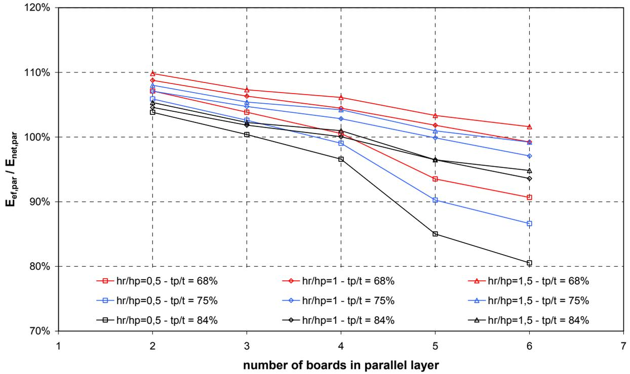
Fig. 124 Ratio between  $E_{ef}$  and  $E_{net}$  for long 5-ply DLT beams (Series 2-3)
