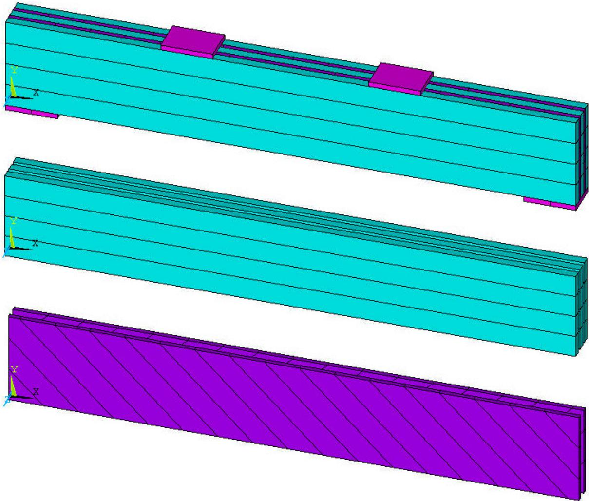
Fig. 99 FE system for specimen 2-1 (short DLT with five plies)
