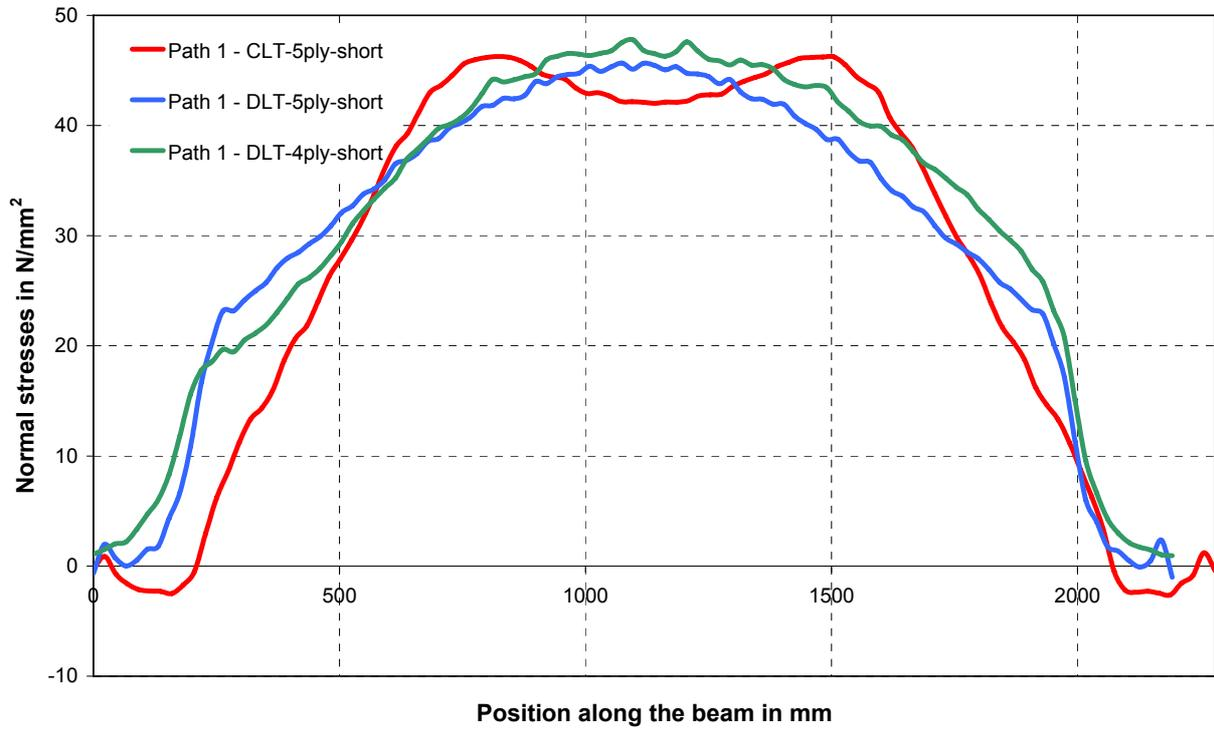
Fig. 33 Distribution of normal stresses  $\sigma_x$  along path 1 for short beams
