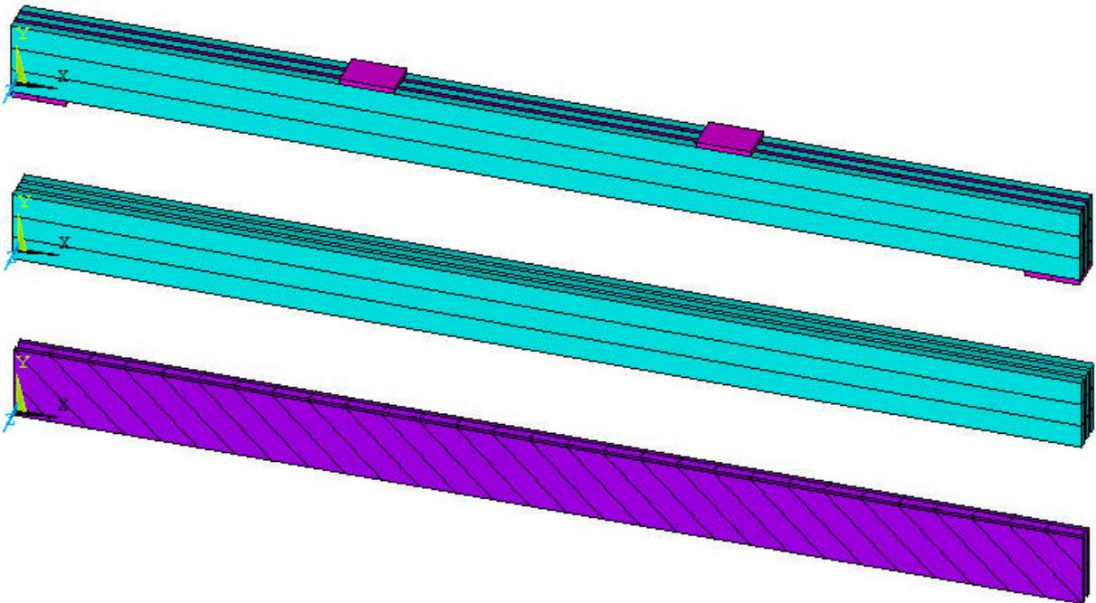
Fig. 108 FE system for specimen 2-3 (long DLT with five plies)
