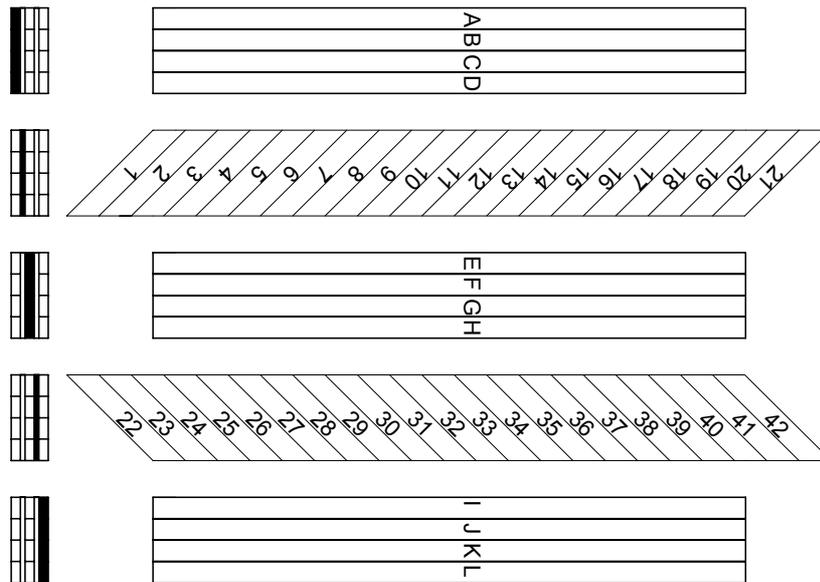
Fig. 49 Species 2.1 – Short beam with 45° reinforcing layers - 5 ply
