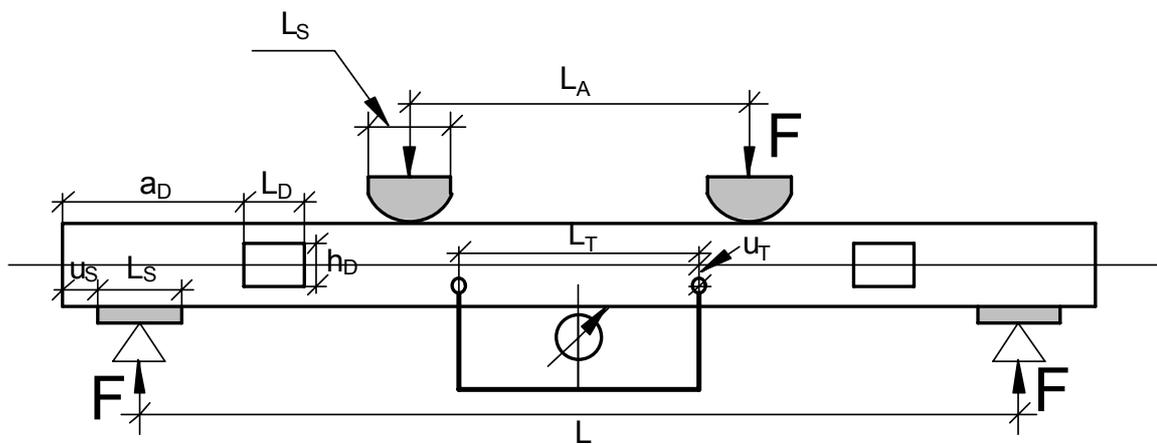
Fig. 19 Test set-up for long beams with holes
