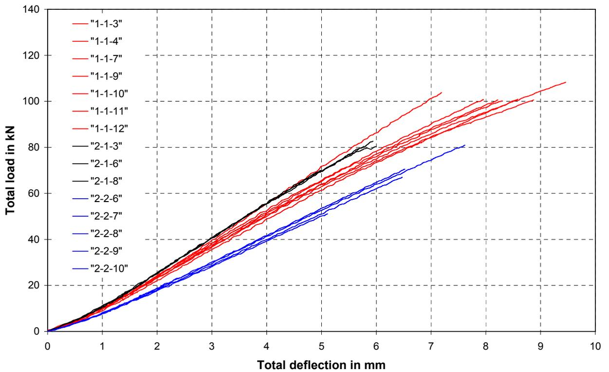
Fig. 80 Load-displacement behaviour for short beams with notches
