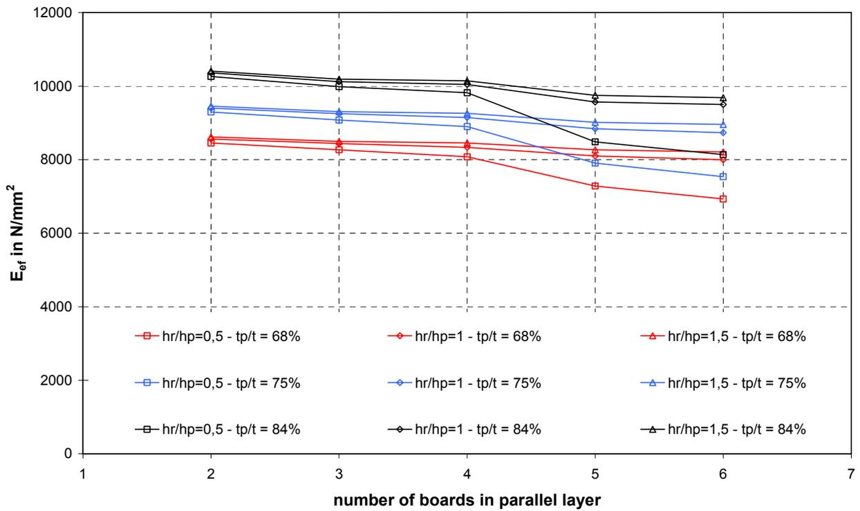
Fig. 117  $E_{ef}$  for long 5-ply CLT beams (Series 1-2)
