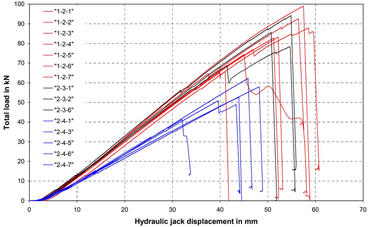
Fig. 85 Load-displacement behaviour for long beams with holes
