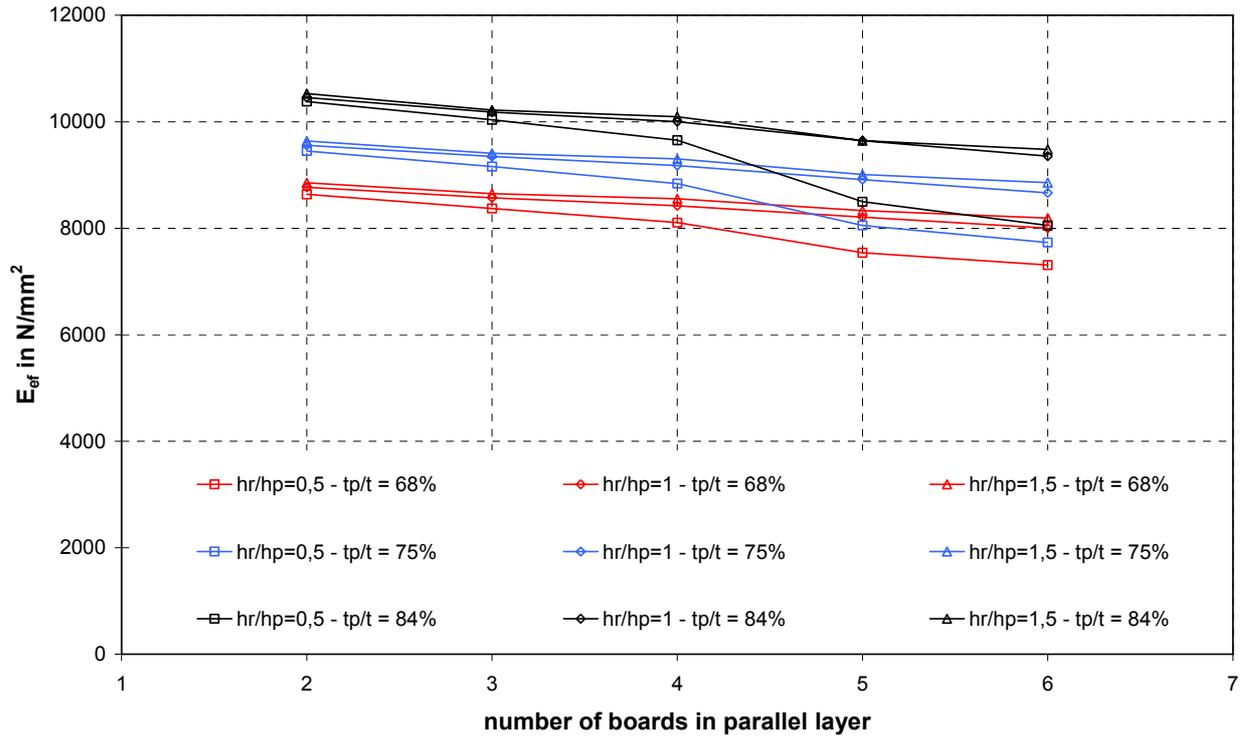
Fig. 118  $E_{ef}$  for long 5-ply DLT beams (Series 2-3)
