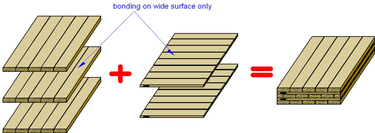
Fig. 1 From raw material to cross laminated timber (CLT) panel
