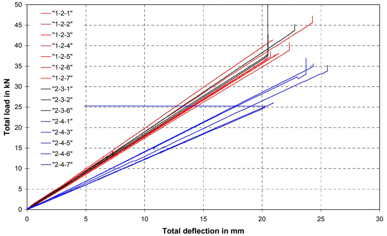
Fig. 86 Load-displacement behaviour for long beams with holes
