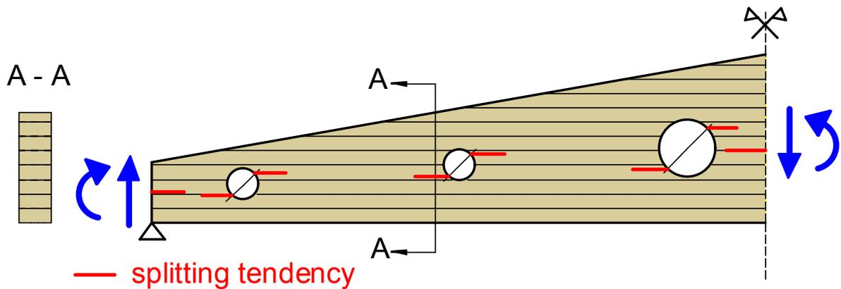
Fig. 4 Glulam beam loaded by tensile stresses perpendicular to the grain and by shear stresses
