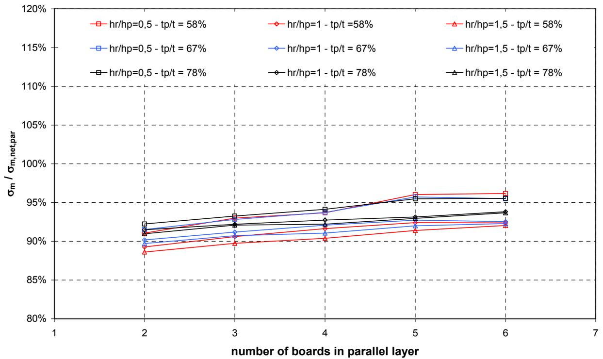
Fig. 131 Ratio between  $\sigma_m$  and  $\sigma_{m,net}$  for long 4-ply DLT beams (Series 2-4)
