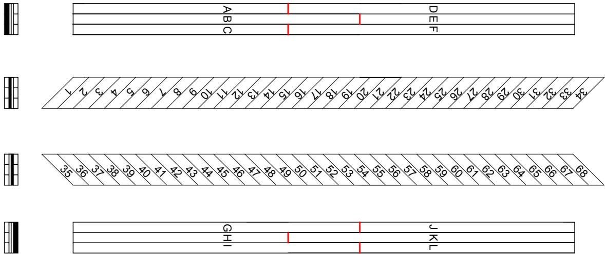
Fig. 52 Species 2.4 – Long beam with 45° reinforcing layers - 4 ply
