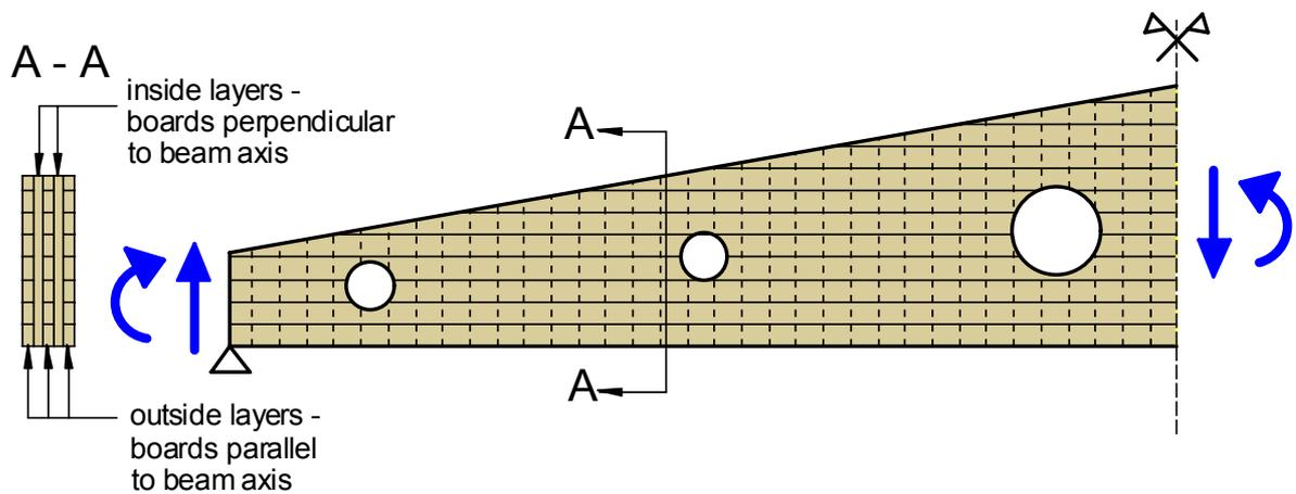
Fig. 5 Beam loaded by tensile stresses perpendicular to the grain made using CLT elements
