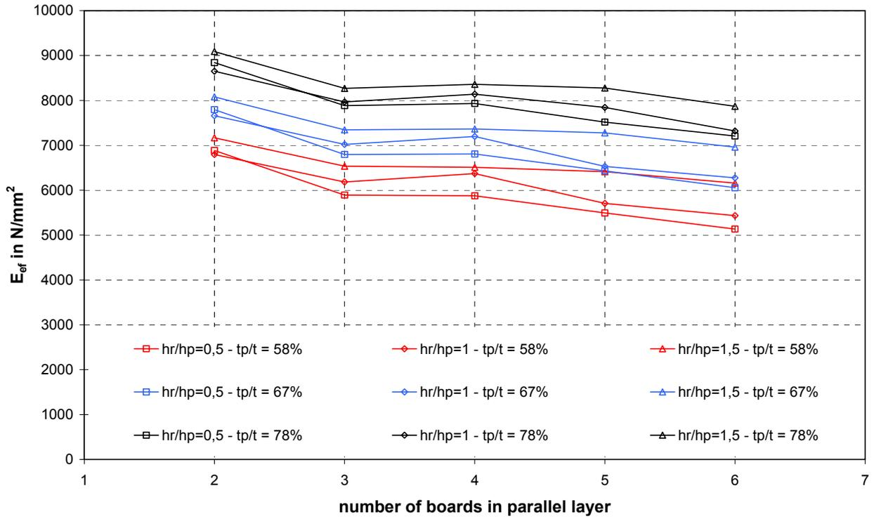
Fig. 116  $E_{ef}$  for short 4-ply DLT beams (Series 2-2)
