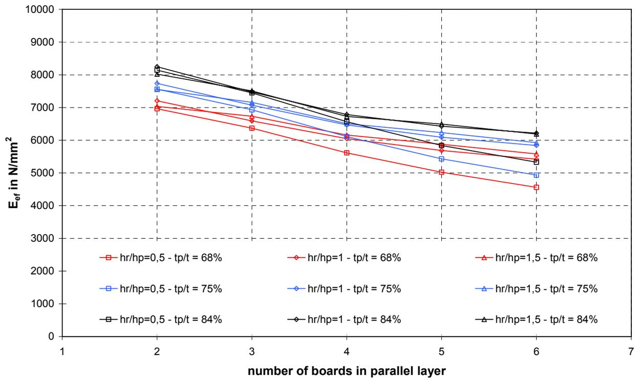
Fig. 115  $E_{ef}$  for short 5-ply DLT beams (Series 2-1)
