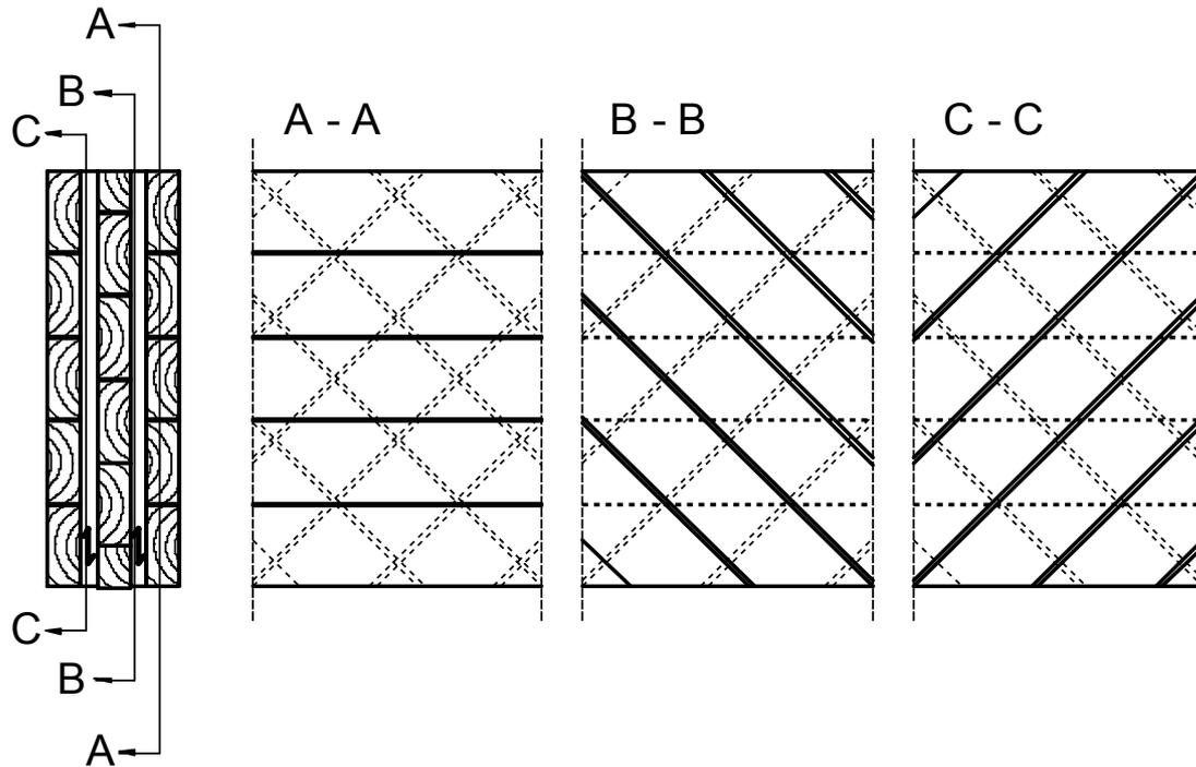
Fig. 6 Modified CLT element with diagonal orientated inner layers
