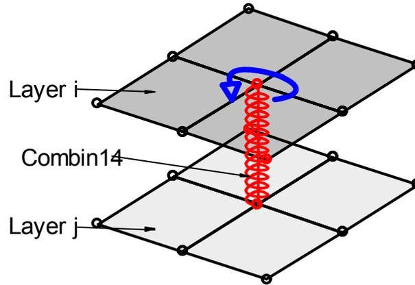
Fig. 23 ANSYS 10 – Combin14 - spring element used for the bonding between the boards
