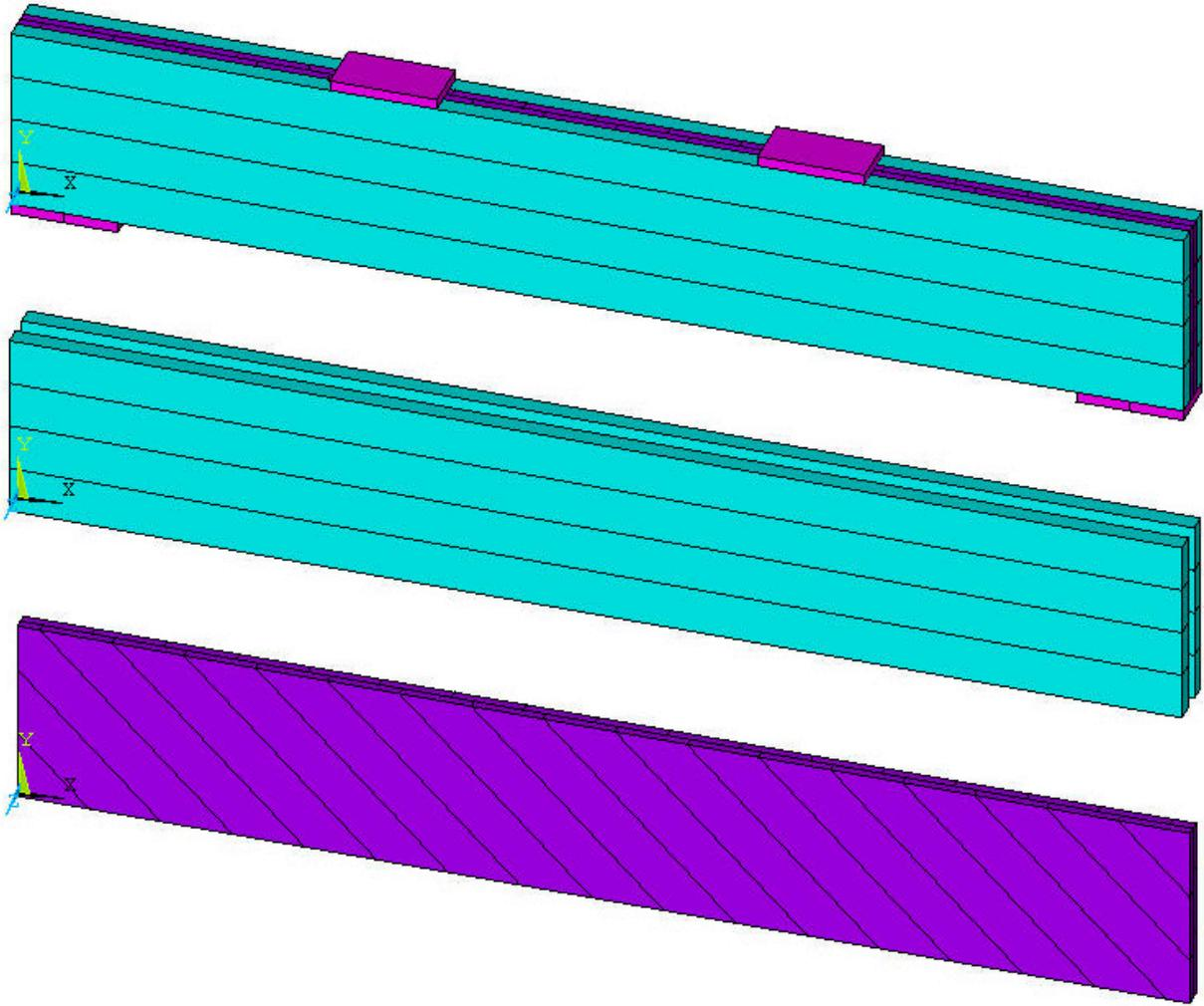
Fig. 102 FE system for specimen 2-2 (short DLT with four plies)
