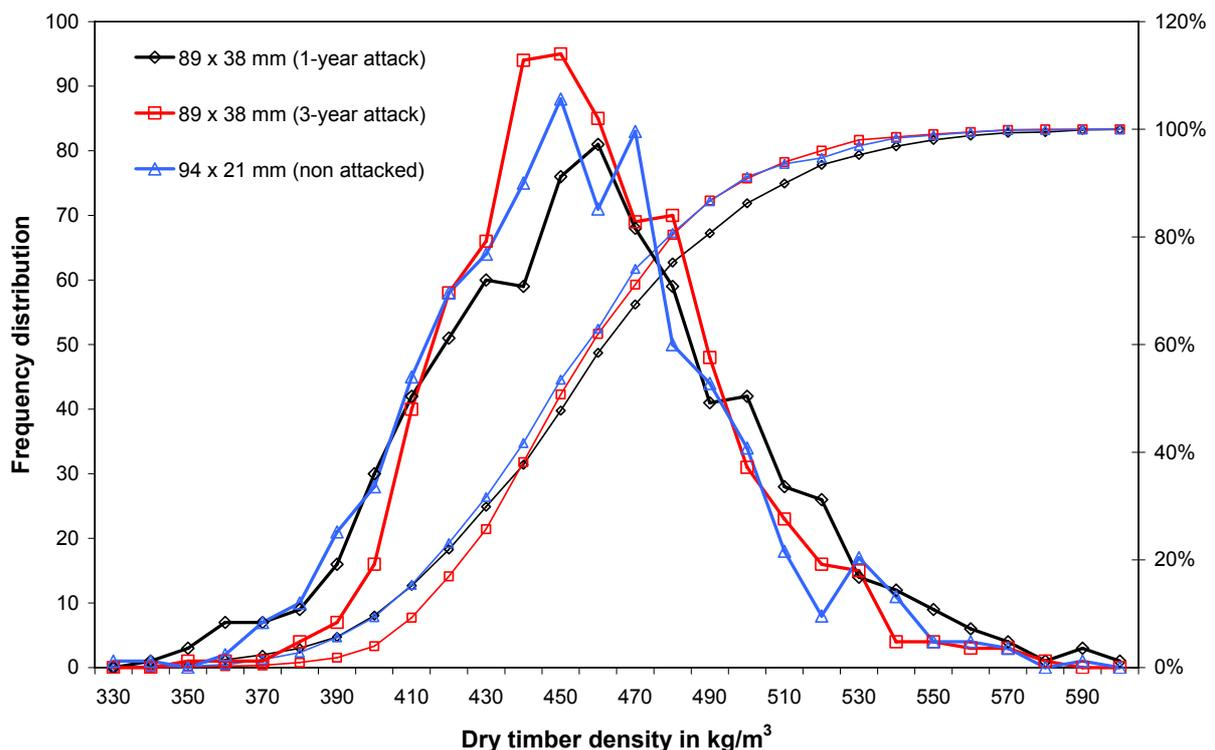
Fig. 9 Frequency distribution for the dry timber density
