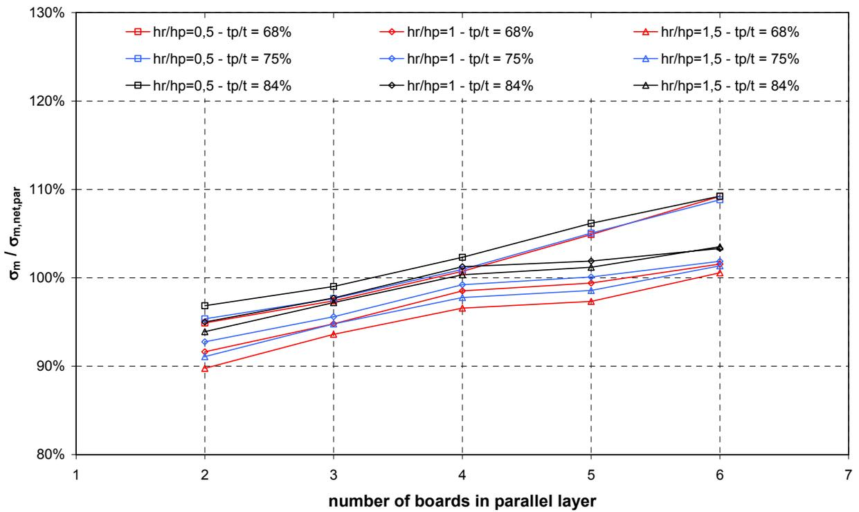
Fig. 127 Ratio between  $\sigma_m$  and  $\sigma_{m,net}$  for short 5-ply DLT beams (Series 2-1)
