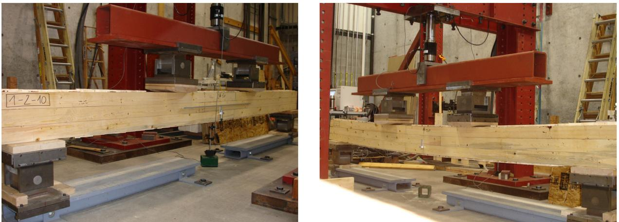
Fig. 76 Testing assembly for long beams (left). Loaded long beam before bending failure (right)
