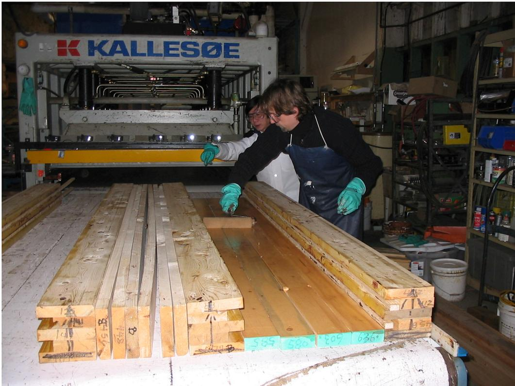
Fig. 53 Species 1.1 – Application of the PRF glue on the first parallel layer
