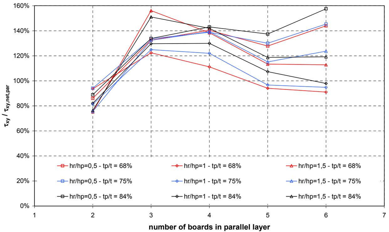
Fig. 135 Ratio between  $\tau_{xy}$  and  $\tau_{xy,net}$  for long 5-ply CLT beams (Series 2-1)
