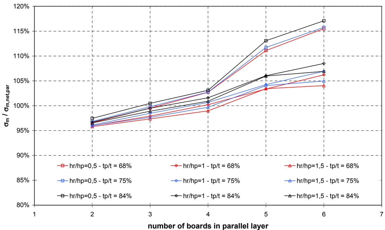
Fig. 129 Ratio between  $\sigma_m$  and  $\sigma_{m,net}$  for long 5-ply CLT beams (Series 1-2)
