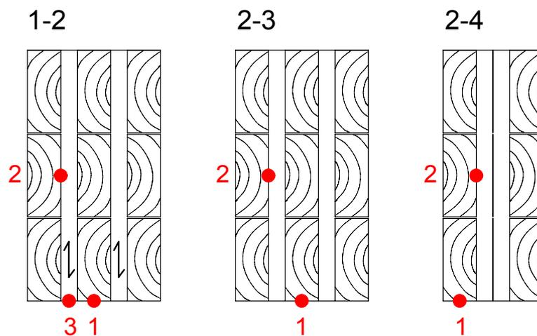
Fig. 32 Path definition for long beams (path 1 for  $\sigma_x$ , path 2 for  $\tau_{xy}$ , path 3 for  $\sigma_y$ )
