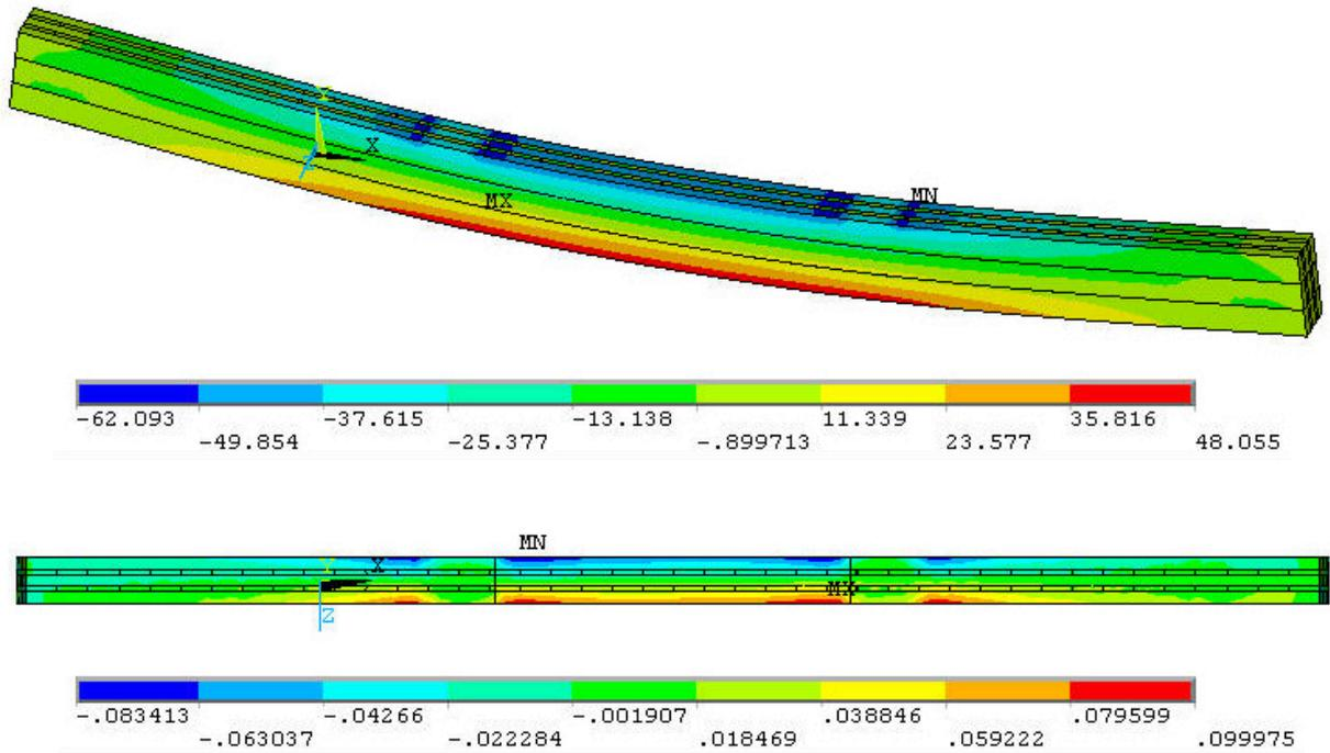
Fig. 107 Bending stresses (top) and deflection in z-direction (bottom) (three times distorted)
