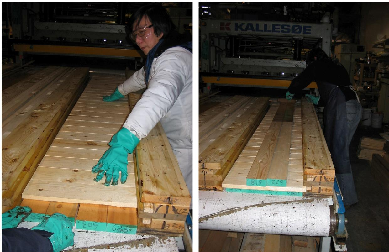
Fig. 54 Species 1.1 – Left: Assembling of the first reinforcing layer (90°). Right: Assembling of the second parallel layer
