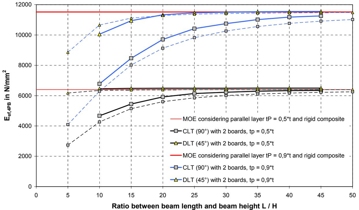
Fig. 28 Effective MOE for DLT beams (45°) and CLT beams (90°) – Comparison between numerical and analytical results
