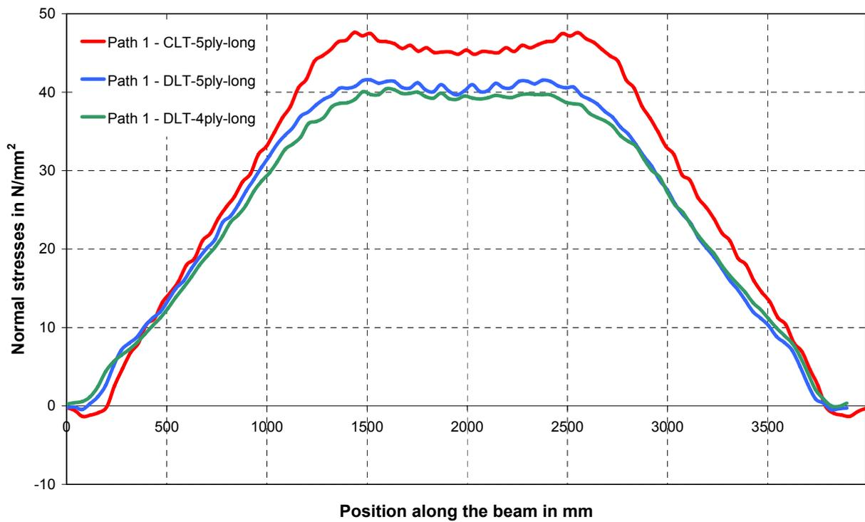
Fig. 34 Distribution of normal stresses  $\sigma_x$  along path 1 for long beams
