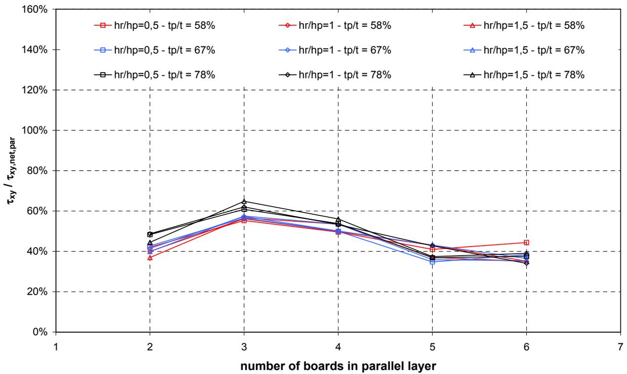
Fig. 137 Ratio between  $\tau_{xy}$  and  $\tau_{xy,net}$  for long 4-ply DLT beams (Series 2-4)
