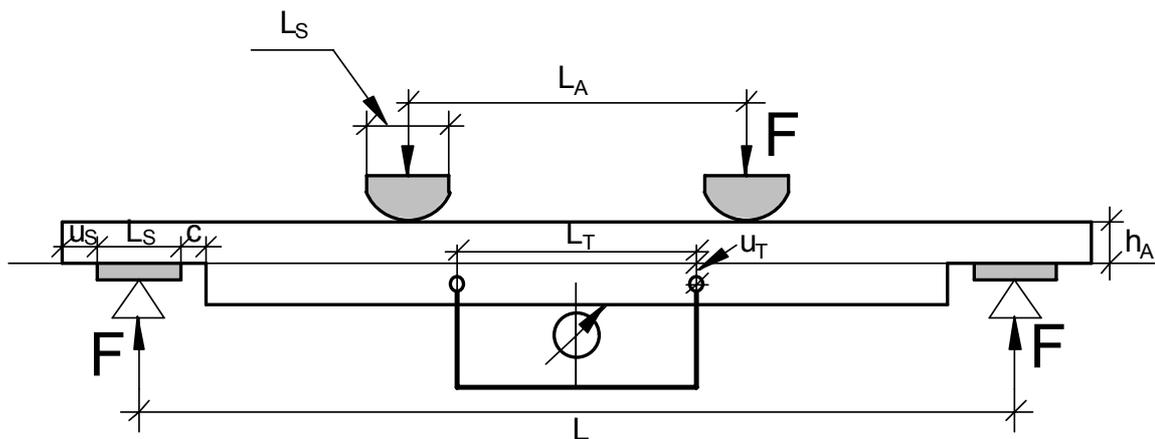
Fig. 18 Test set-up for short beams with notches
