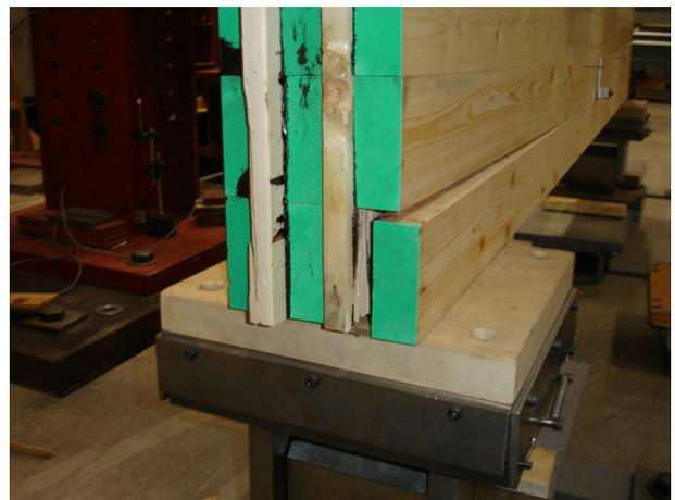
Fig. 70 Typical failure in bending for CLT beam (left). Failure at the CLT beam end (right)
