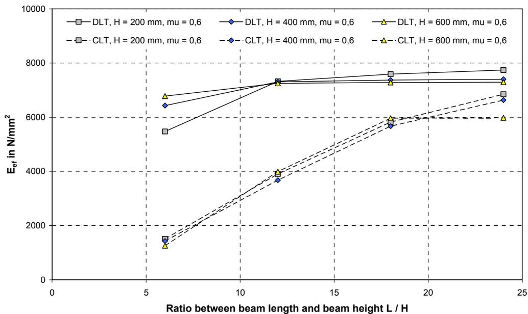
Fig. 30 Effective MOE  $E_{ef}$  for CLT and DLT elements (plane model with  $\mu = 0.6$ )
