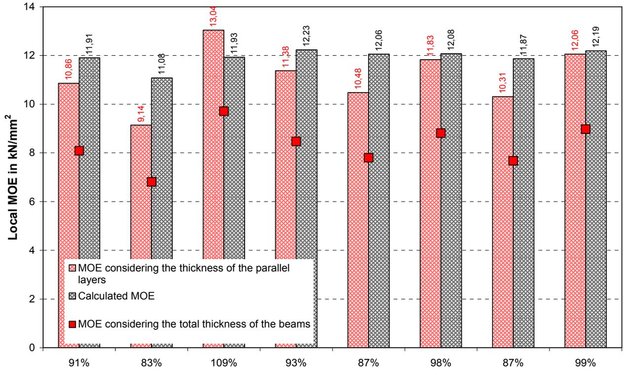
Fig. 92  $E_{0,net}$  ( $E_0$ ) versus  $E_{cal}$  for specimens 2-1 (short DLT with five plies)
