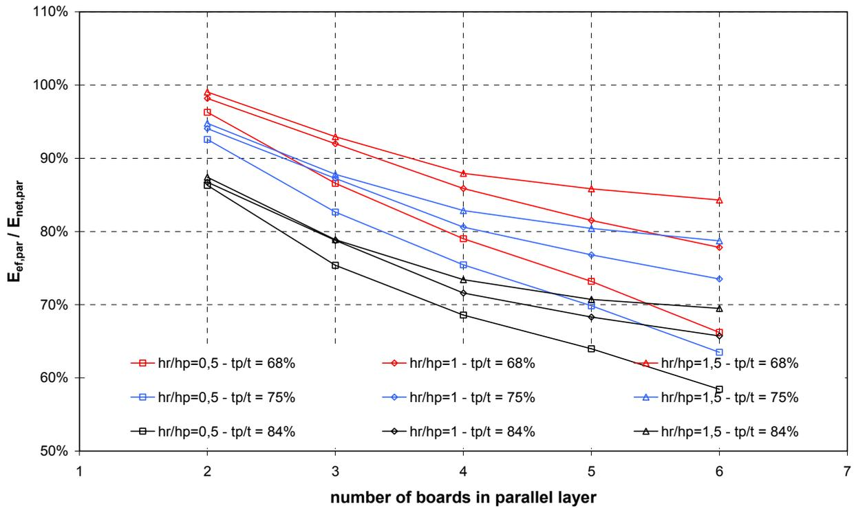
Fig. 120 Ratio between  $E_{ef}$  and  $E_{net}$  for short 5-ply CLT beams (Series 1-1)
