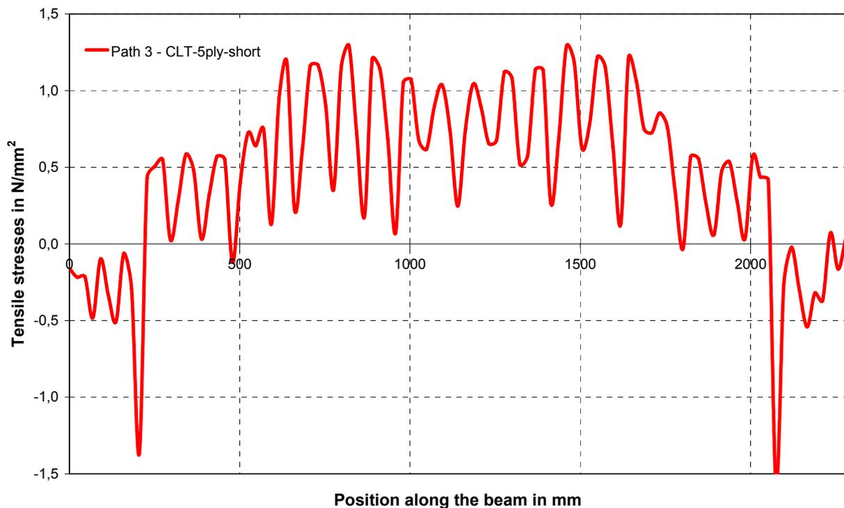
Fig. 37 Distribution of stresses perpendicular to beam axis  $\sigma_y$  along path 3 for short beams
