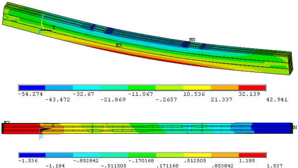
Fig. 110 Bending stresses (top) and deflection in z-direction (bottom) (three times distorted)
