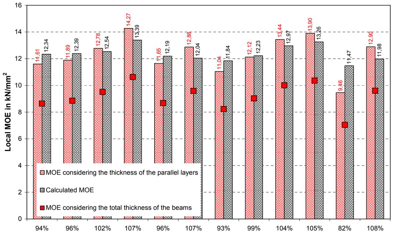
Fig. 91  $E_{0,net}$  ( $E_0$ ) versus  $E_{cal}$  for specimens 1-2 (long CLT with five plies)
