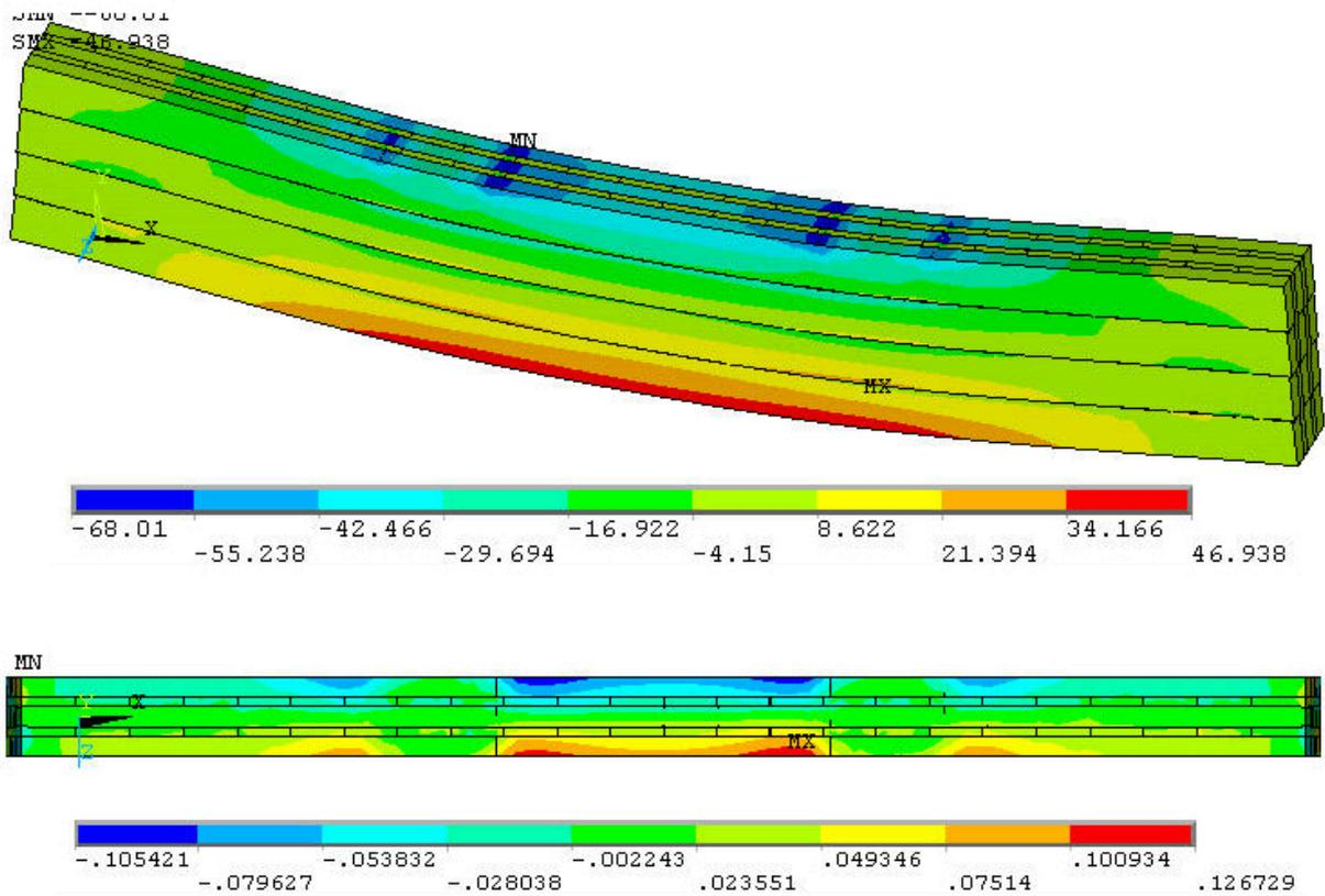
Fig. 98 Bending stresses (top) and deflection in z-direction (bottom) (five times distorted)
