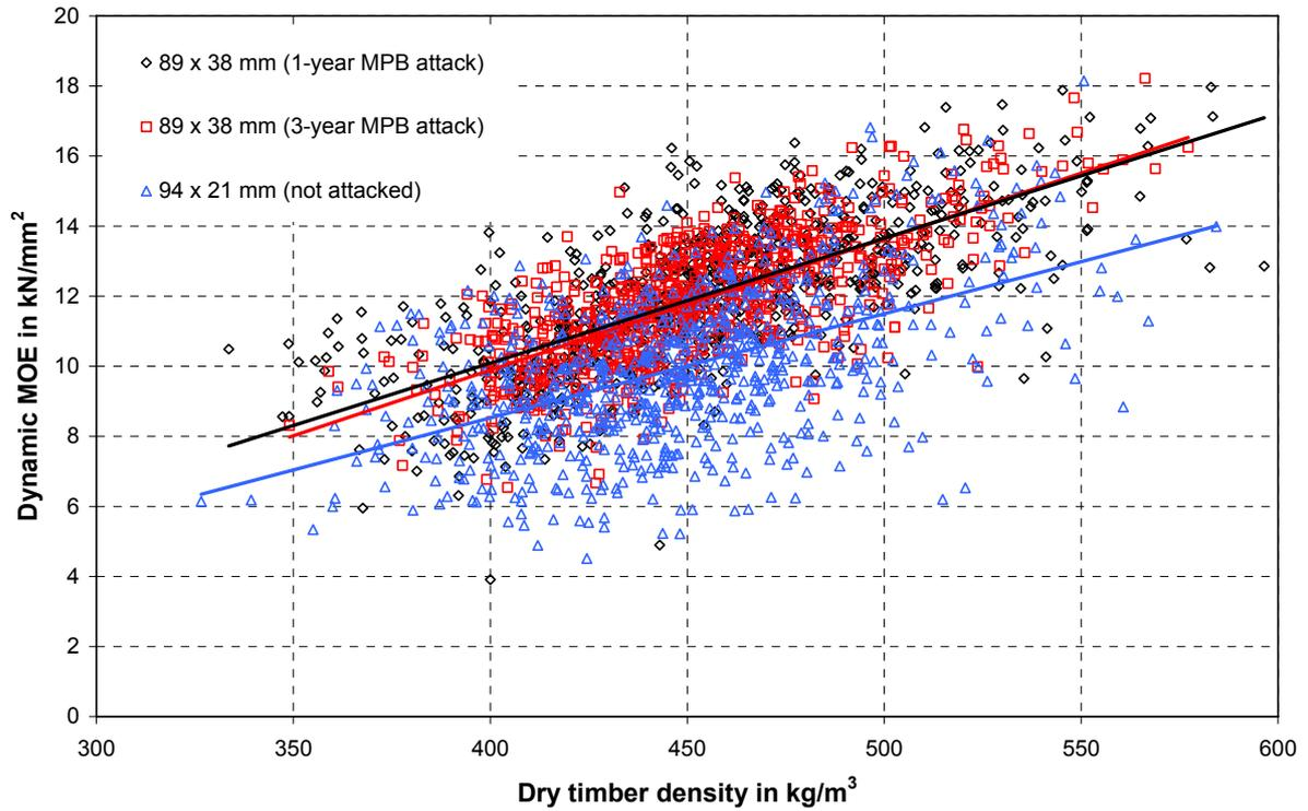
Fig. 11 Relation between the dynamic MOE and the dry timber density
