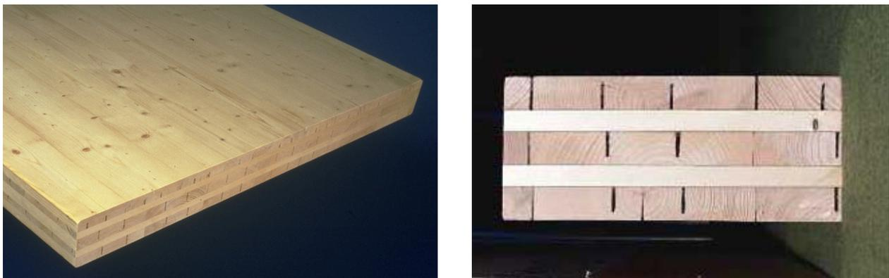
Fig. 2 CLT panel with gaps and grooves
