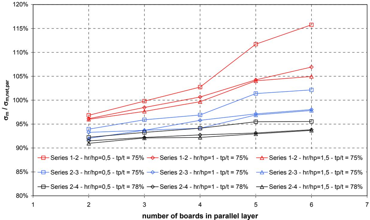
Fig. 44 Ratio between  $\sigma_m$  and  $\sigma_{m,net}$  for long beams with  $t_p/t = 75\%$  (78%)
