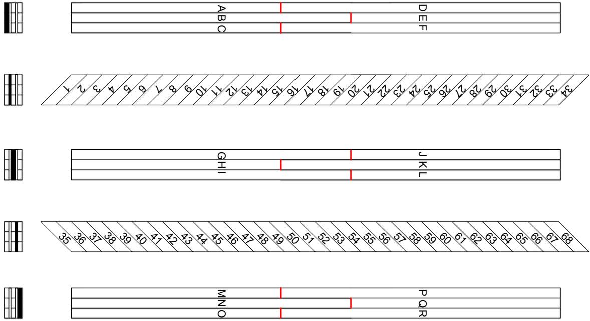
Fig. 51 Species 2.3 – Long beam with 45° reinforcing layers - 5 ply
