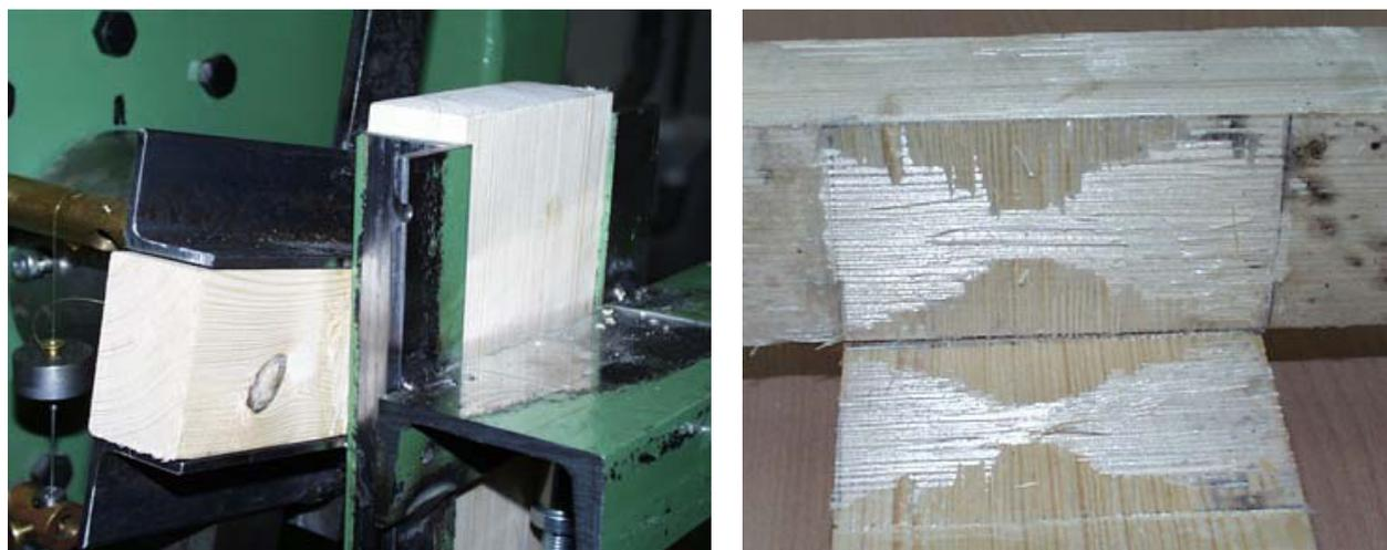
Fig. 21 Left: Test configuration. Right: Test specimen after failure (Figures taken from [2])
