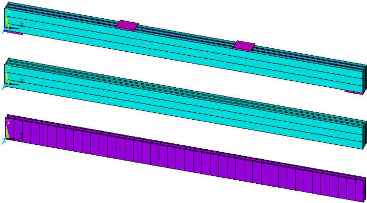
Fig. 105 FE system for specimen 1-2 (long CLT with five plies)
