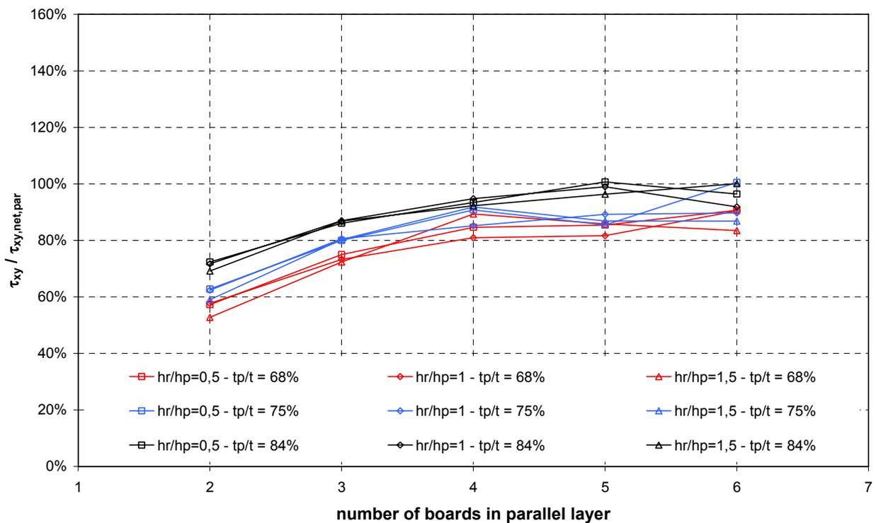
Fig. 133 Ratio between  $\tau_{xy}$  and  $\tau_{xy,net}$  for short 5-ply DLT beams (Series 2-1)
