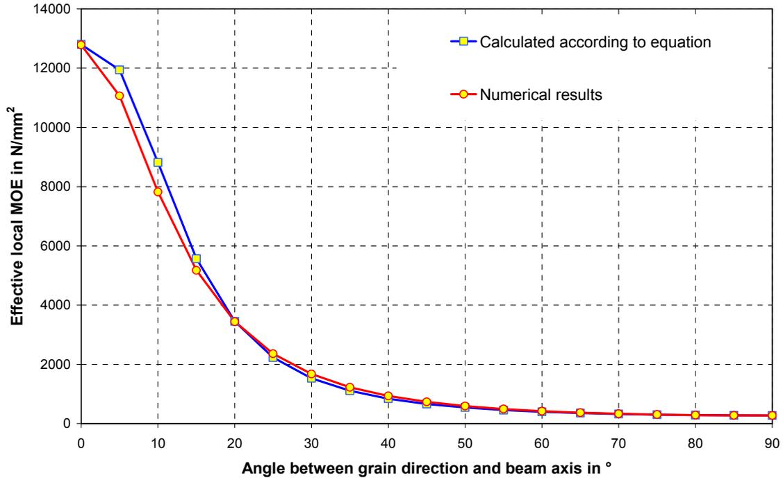
Fig. 8 Relationship between inclination and local MOE in the beam axis direction
