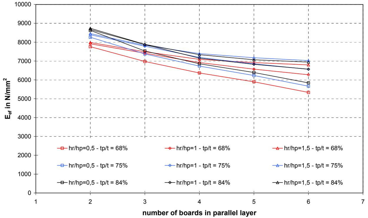
Fig. 114  $E_{ef}$  for short 5-ply CLT beams (Series 1-1)
