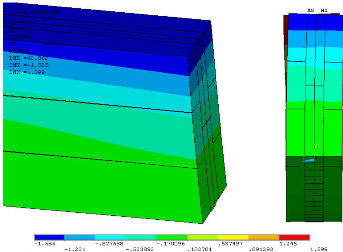
Fig. 112 Beam end with deflection in z-direction (Sp.2-4, three times distorted)
