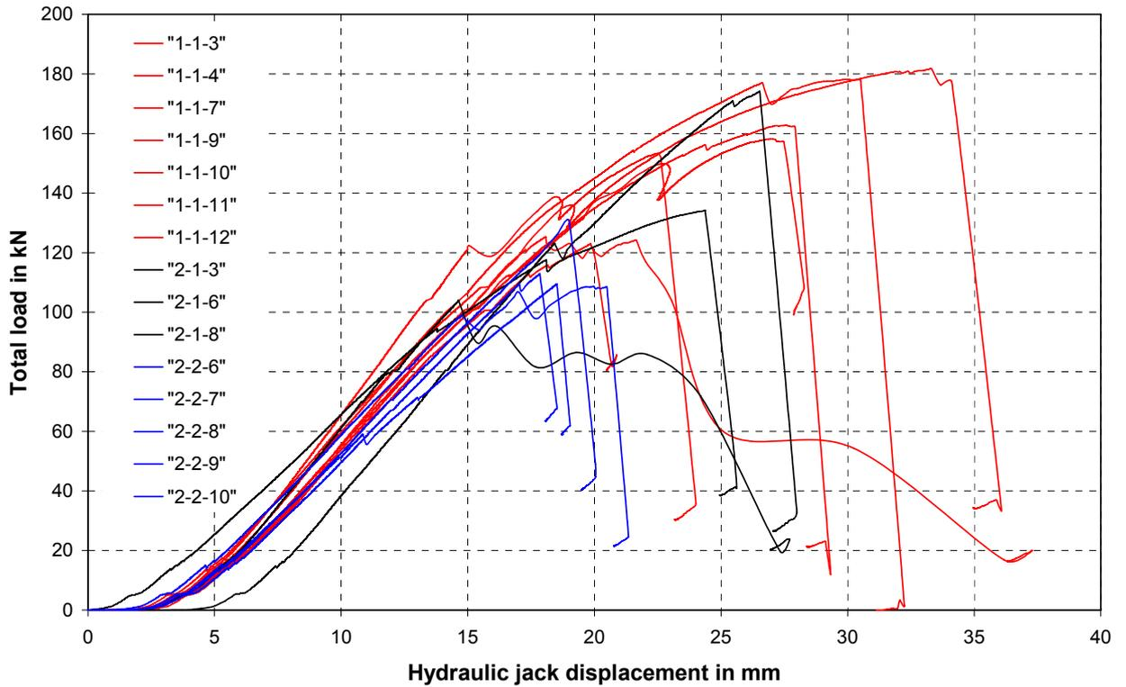
Fig. 79 Load-displacement behaviour for short beams with notches
