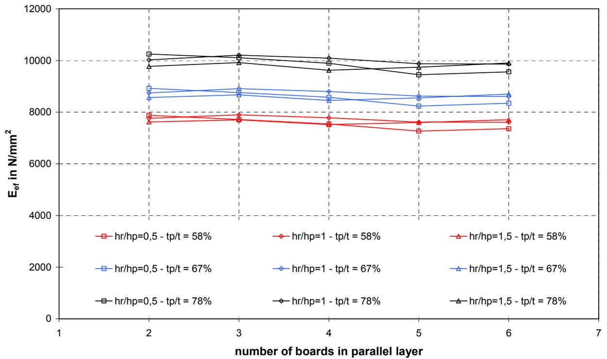
Fig. 119  $E_{ef}$  for long 4-ply DLT beams (Series 2-4)
