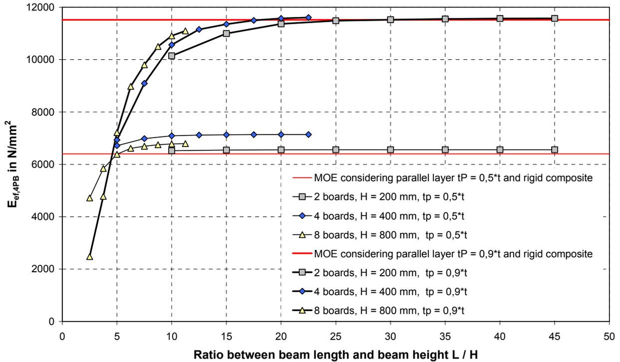
Fig. 27 Effective MOE for DLT beams (45°) with bonding stiffness  $K = 6 \text{ N/mm}^3$
