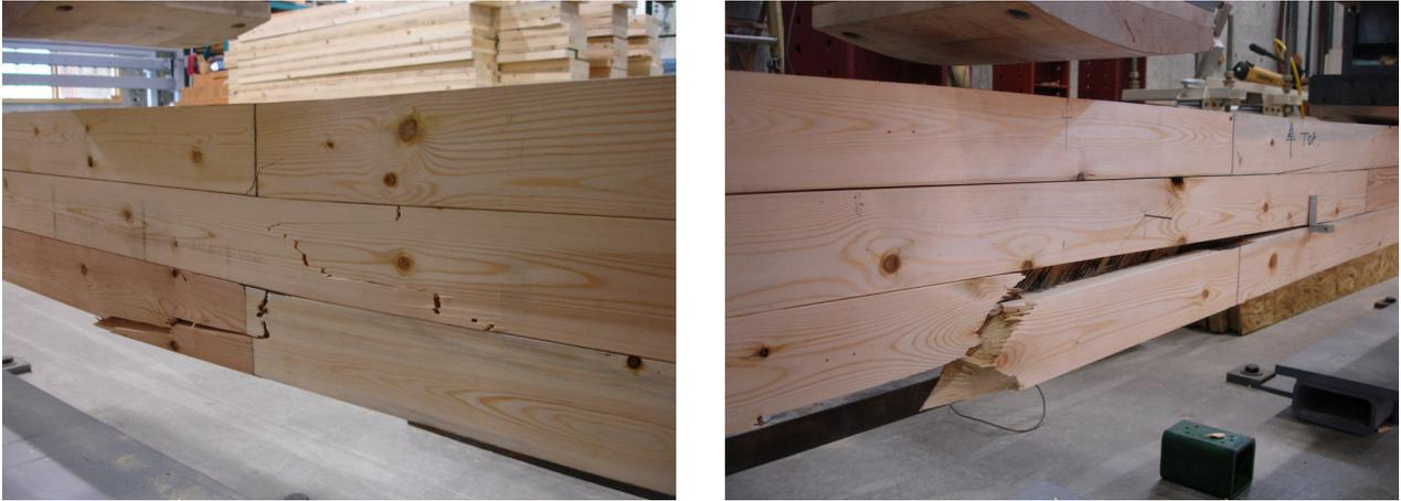
Fig. 89 Bending failure for CLT beams (left) and for DLT beams (right)
