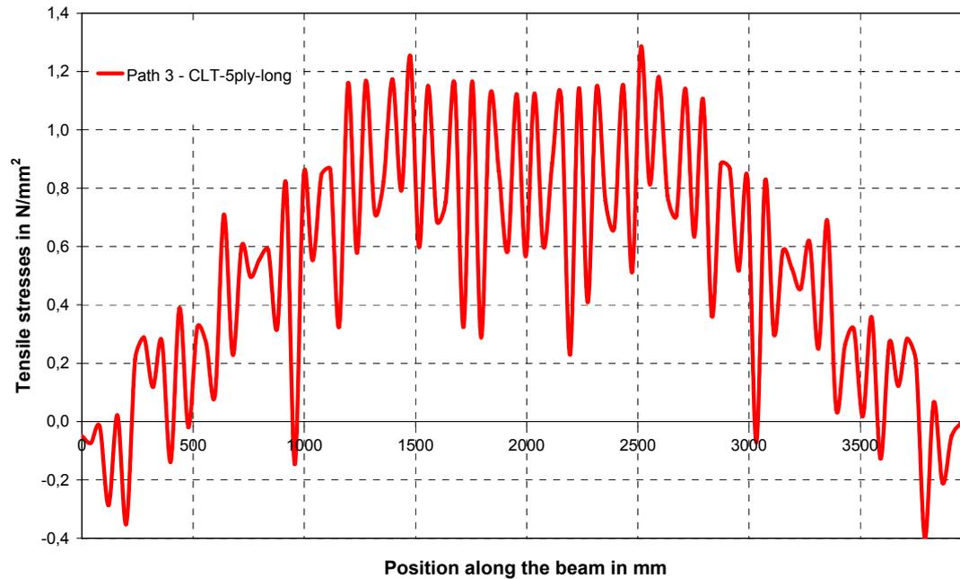
Fig. 38 Distribution of stresses perpendicular to beam axis  $\sigma_y$  along path 3 for long beams
