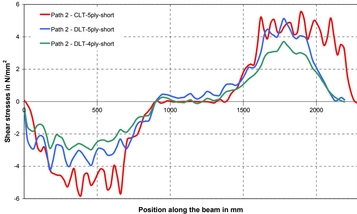
Fig. 35 Distribution of shear stresses  $\tau_{xy}$  along path 2 for short beams
