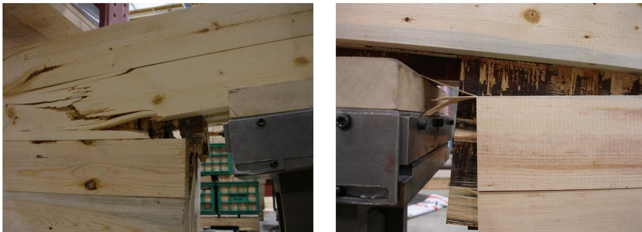
Fig. 82 Typical failure of the reinforcing layer in short CLT beams with notches
