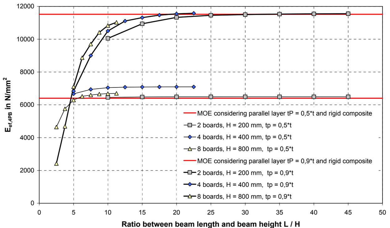
Fig. 26 Effective MOE for DLT beams ( $45^\circ$ ) with bonding stiffness  $K = 3 \text{ N/mm}^3$
