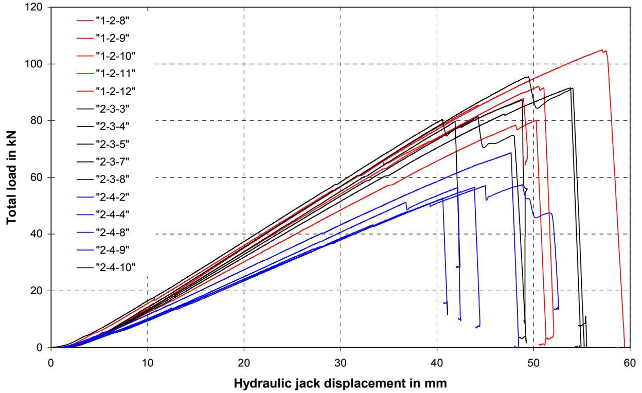
Fig. 73 Load-displacement behaviour for long beams
