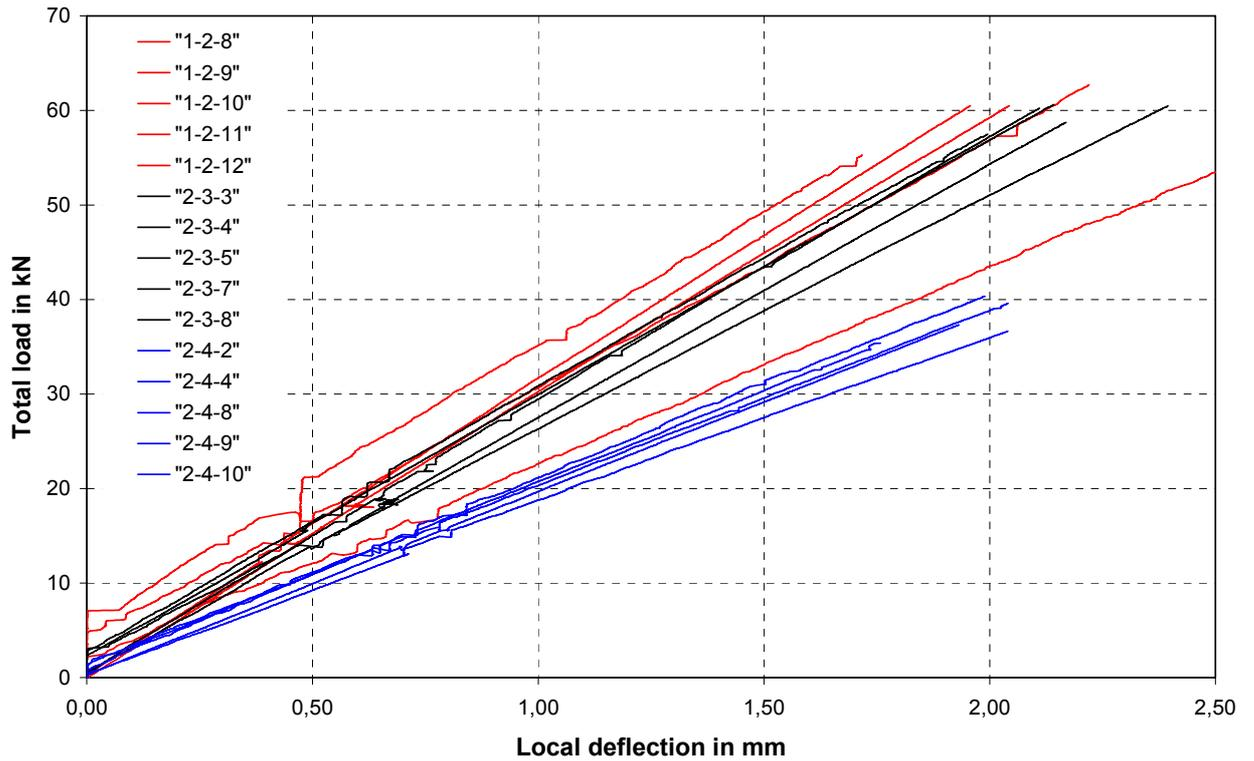
Fig. 75 Load-displacement behaviour for long beams
