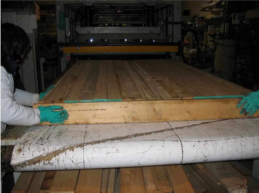
Fig. 57 Species 1.1 – Two beams in a fixing frame on the way to the press
