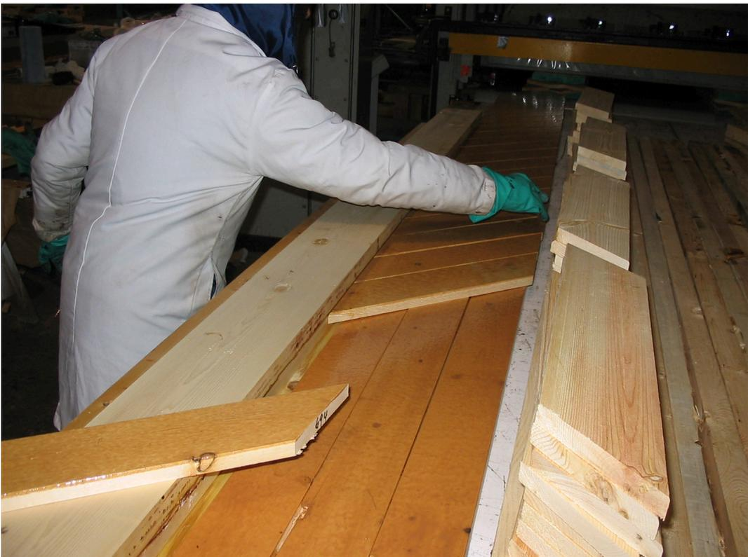
Fig. 60 Species 2.4 – Assembling of the diagonal layer on the first parallel layer
