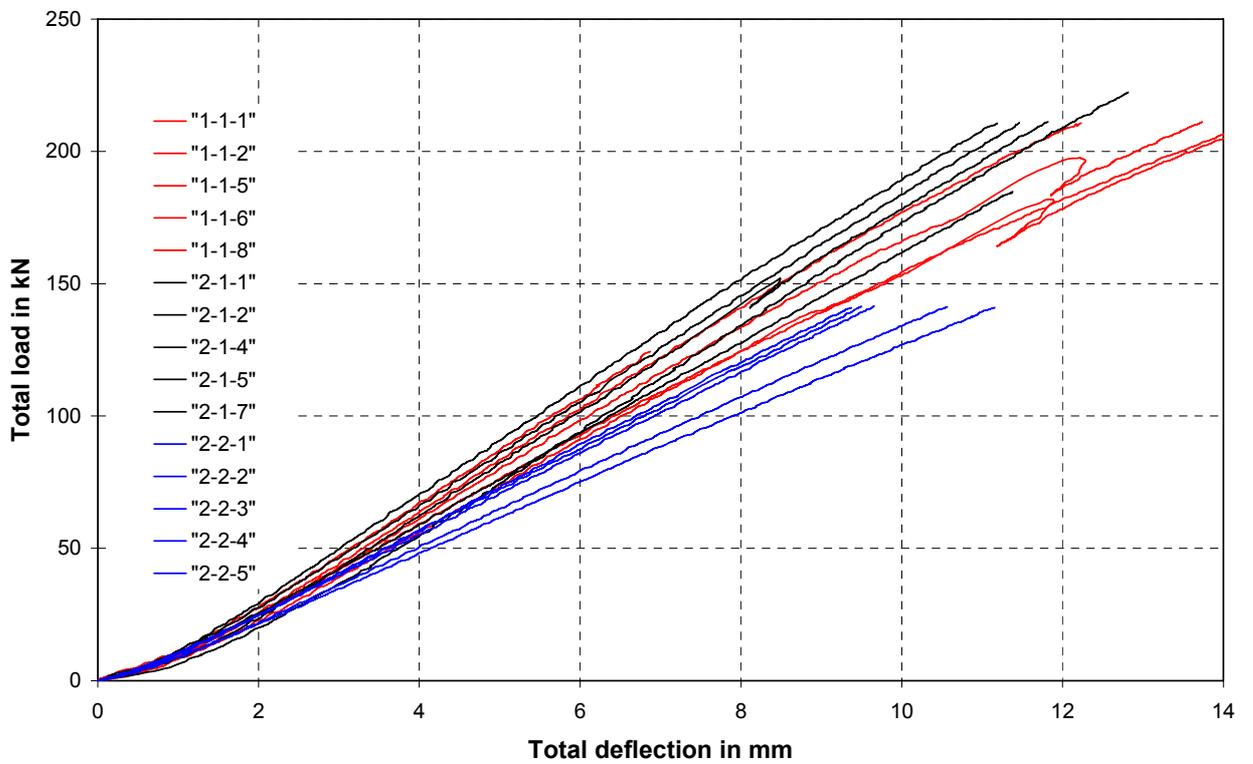
Fig. 68 Load-displacement behaviour for short beams
