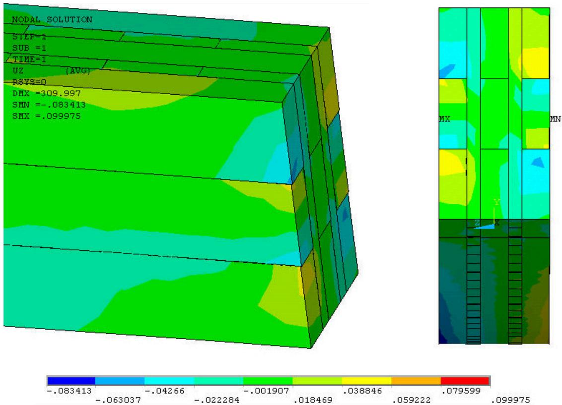
Fig. 106 Beam end with deflection in z-direction (Sp.1-2, three times distorted)
