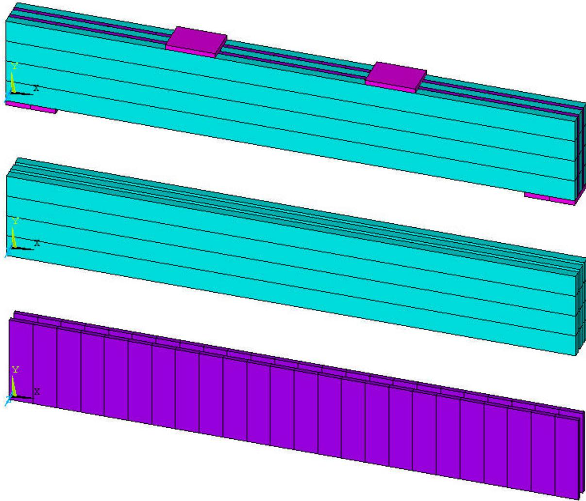
Fig. 96 FE system for specimen 1-1 (short CLT with five plies)
