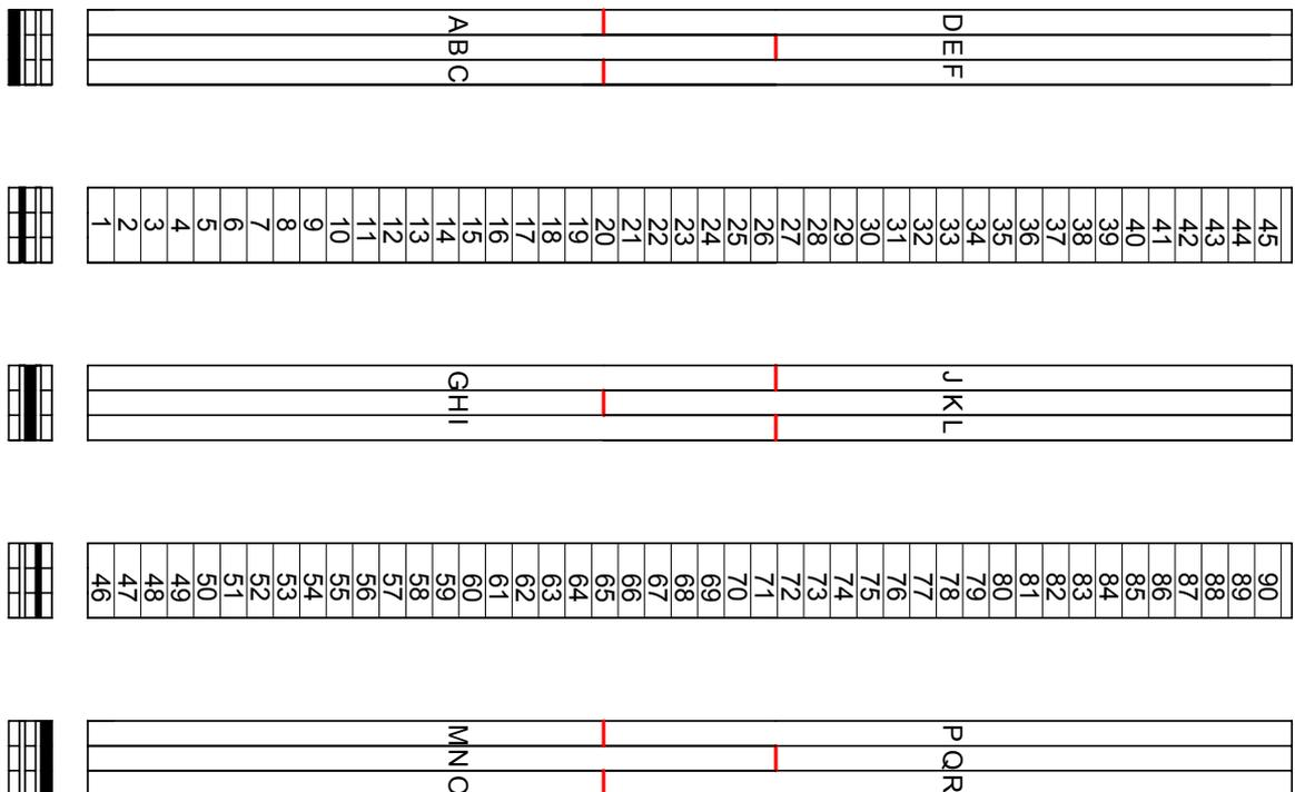
Fig. 48 Species 1.2 – Long beam with 90° reinforcing layers - 5 ply
