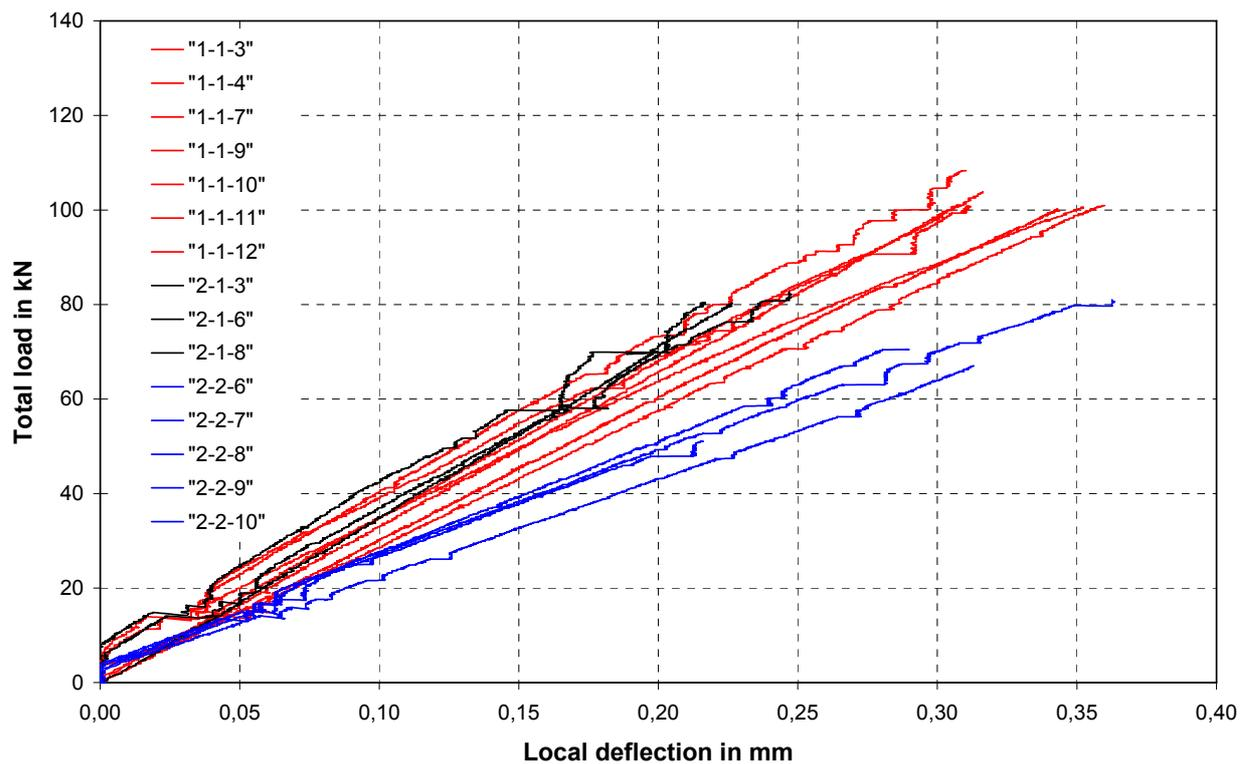
Fig. 81 Load-displacement behaviour for short beams with notches
