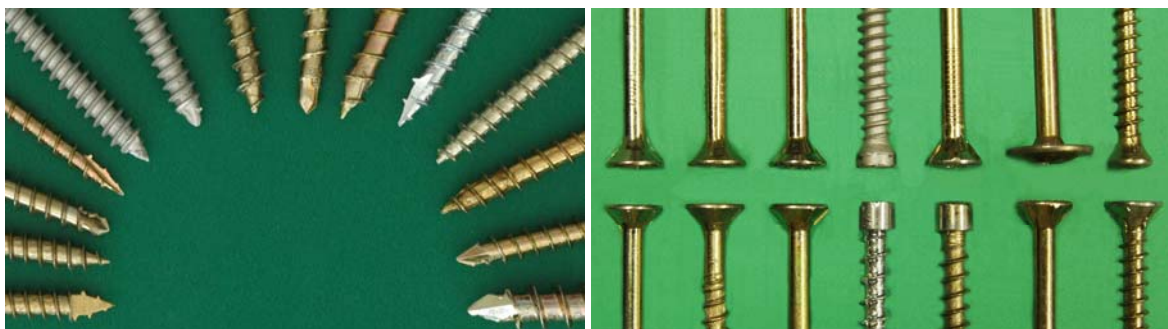
Fig. 3: Different tips and heads of self-tapping screws
