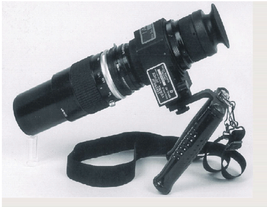
Figure 8.3.2. Cerenkov viewing detector [4,5].
