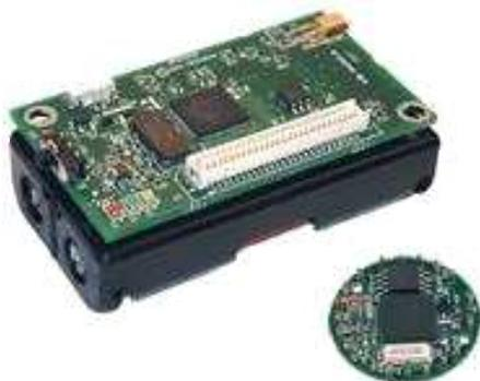
Figure 2.2: Mica motes: Mica2 (left) and Mica2Dot (right)
