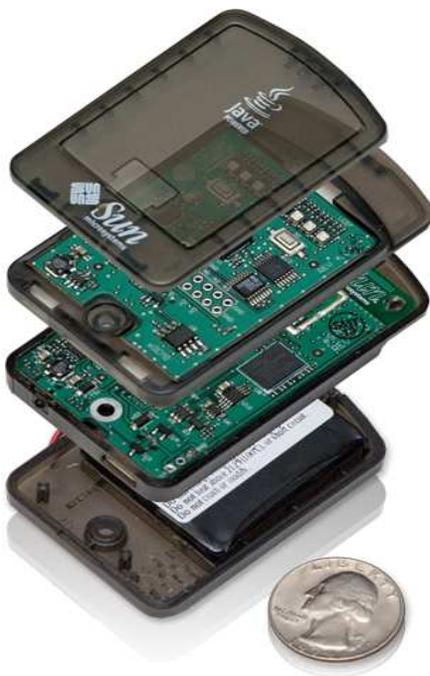
Figure 2.1: A Sun SPOT sensor node and its components
