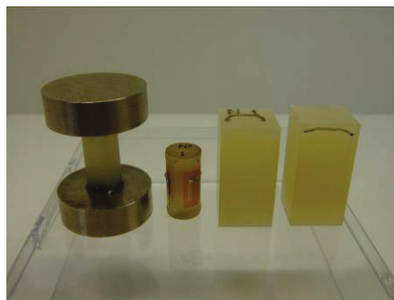
Fig. 7: Showing geometry of compression sample PCR1 (steel caps), PCR2 with 8 mm diameter and PCR3 (radial), PCR4 (transversal).
