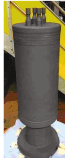
Fig. 2: HV-insulation mock-up - left: glas/G10 insulation, right: mock-up covered with conductive paint.
