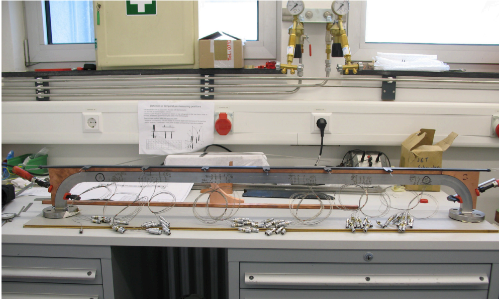
Fig. 4: HETRA channel with assembled cooper parts, graphite layers and electrical heaters.
