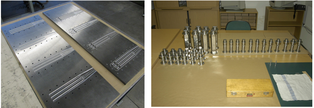
Fig. 4: Examples of already manufactured parts for Gricaman manifolds: left – plates with milled outlet legs of cap channels (parts Mf3-30 and Mf3-31 in Figure 3); manifold flanges (parts Mf2-12 and Mf2-13 in Figure 2 and Mf3-25, Mf3-26 and Mf3-27 in Figure 3).
