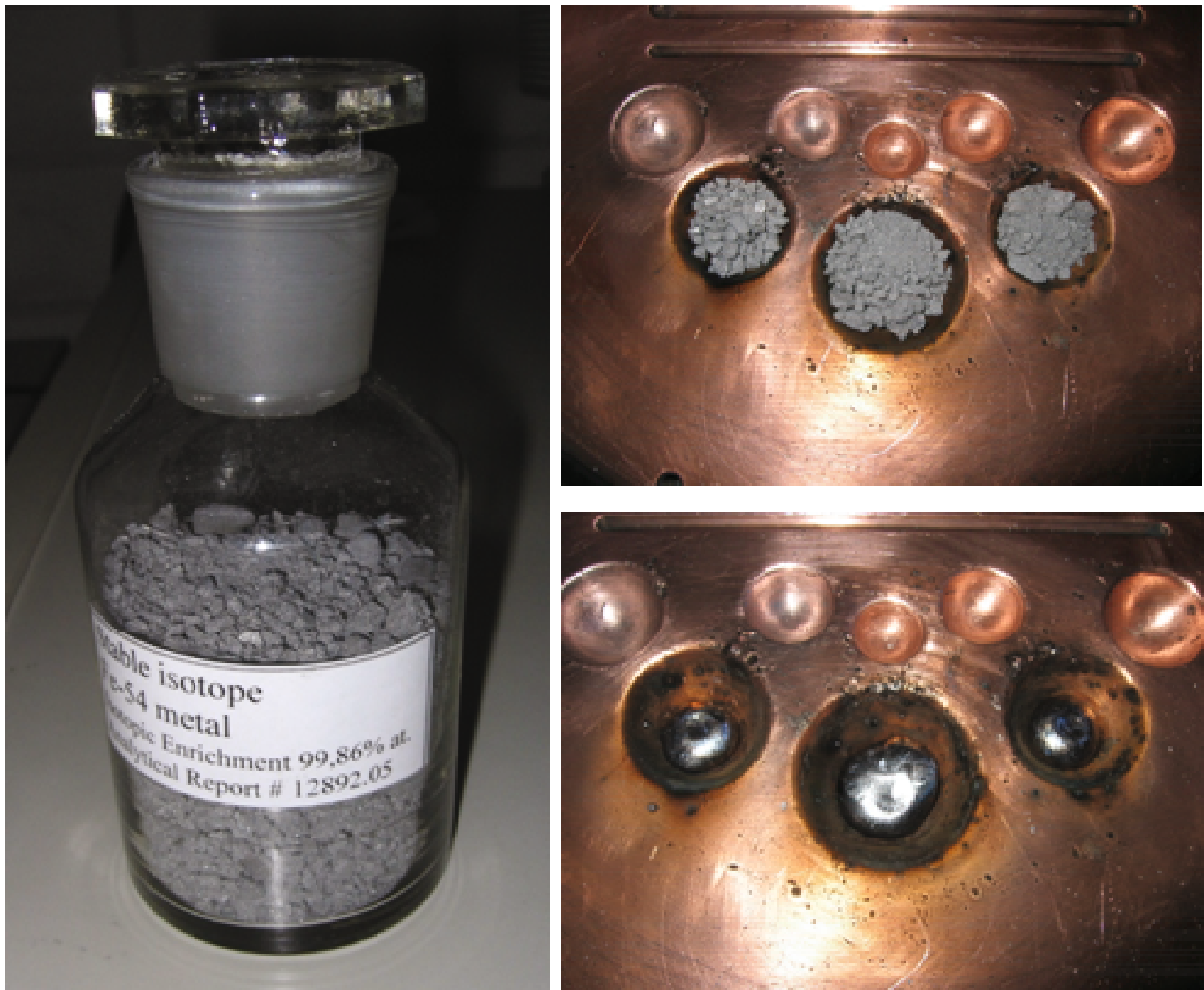
Fig. 1: Left: Bottle with 391 grams of Fe54 Isotope, as delivered. Right upper and lower image: Before and after arc melting the isotope powder to pellets.
