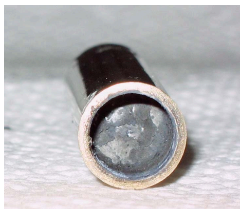
Fig. 2: Be-Ti rod after overpressure sintering inside of Nb tube.
