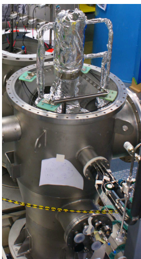
ISS: The opened Cold-Box with a view on the condenser
