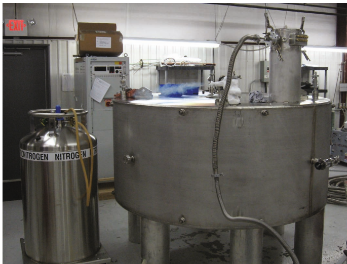
Fig. 8: Completely mounted fast step-tuneable magnet during tests at the manufacturer's site.
