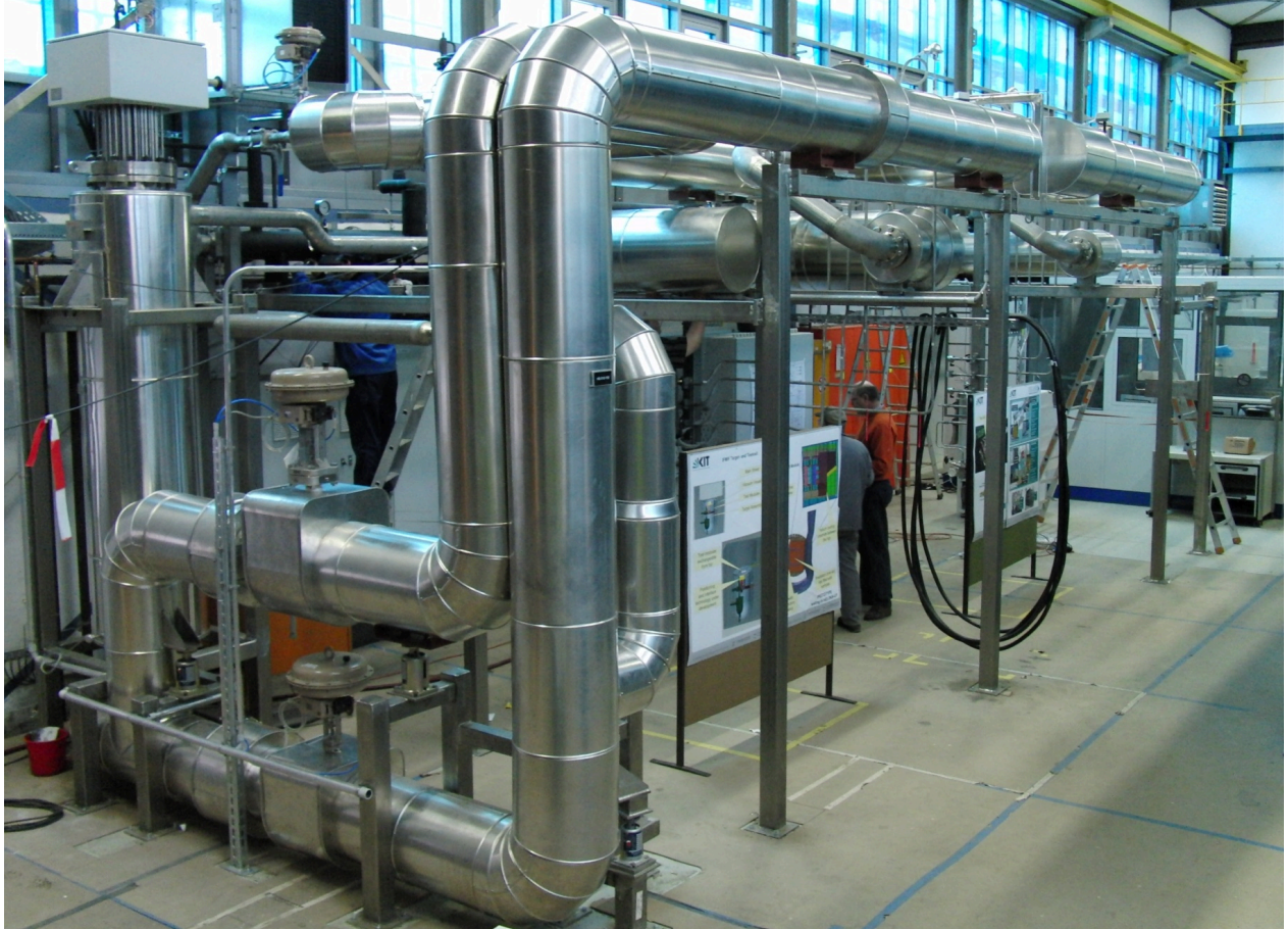
Helium Loop Karlsruhe – Low pressure (HELOKA-LP) for testing the High Flux Test Module for IFMIF
