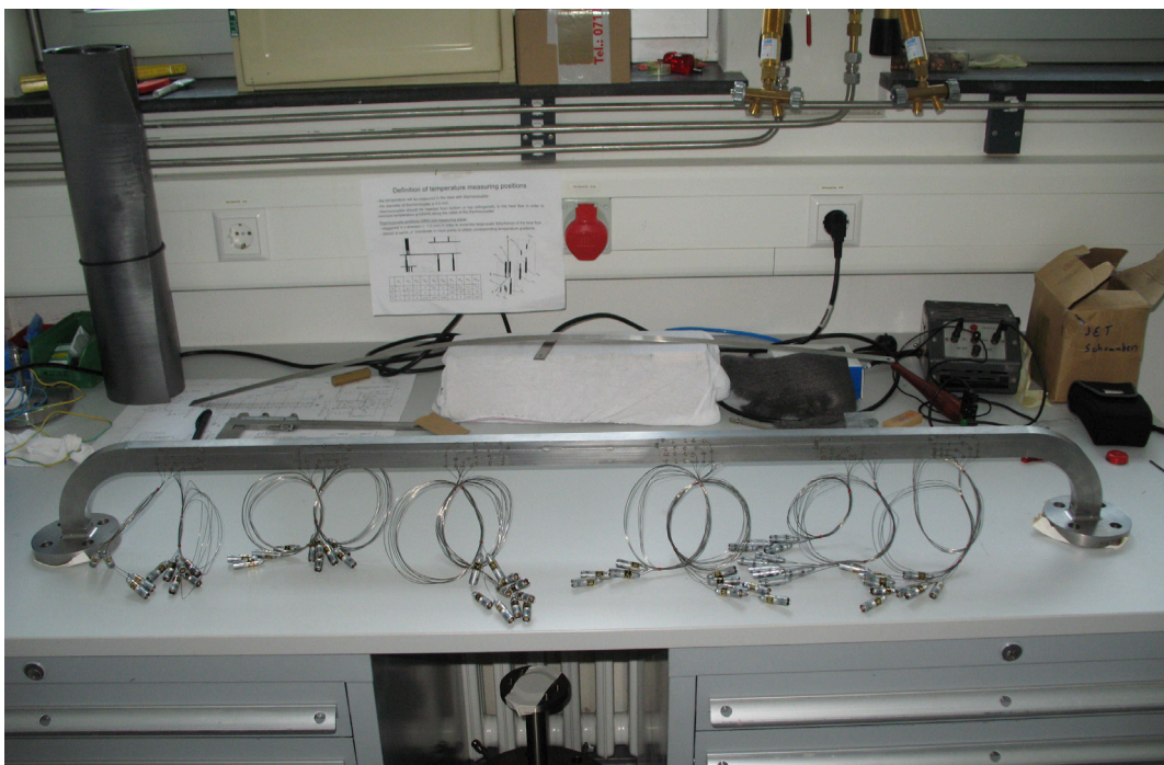
Fig. 2: HETRA channel (heated section) with installed thermocouples.
