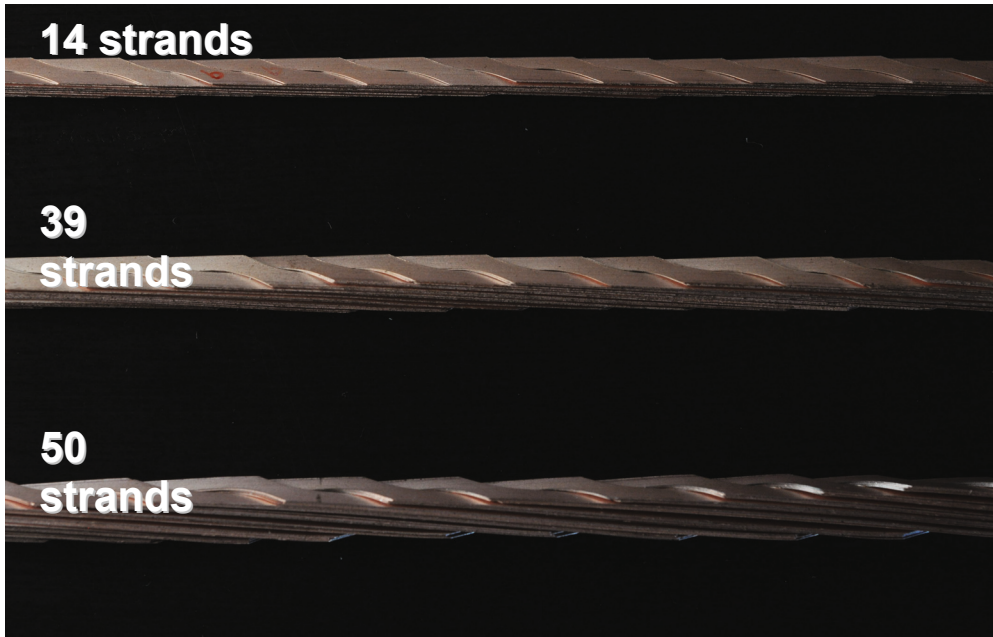
Fig. 2: Different stages of multistacking (1x, 3x, and 5x ) in 4 mm wide RACC-cables with 0.46 kA, 1.1 kA and 1.3 kA transport current (77 K, s.f.)
