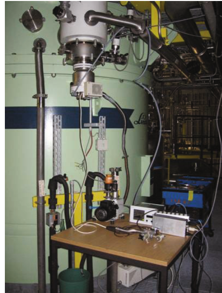
Fig. 5: Test of new vacuum pumps for the thermal insulation of the 2 kW-refrigerator.
