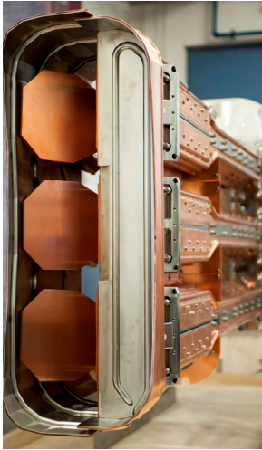
Front-end of the W7-X plug-in antenna with the launching mirrors
