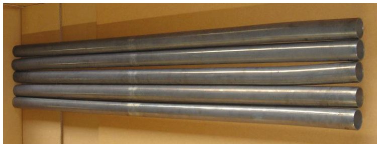
Fig. 1: Picture of the butt welded TF tubes.
