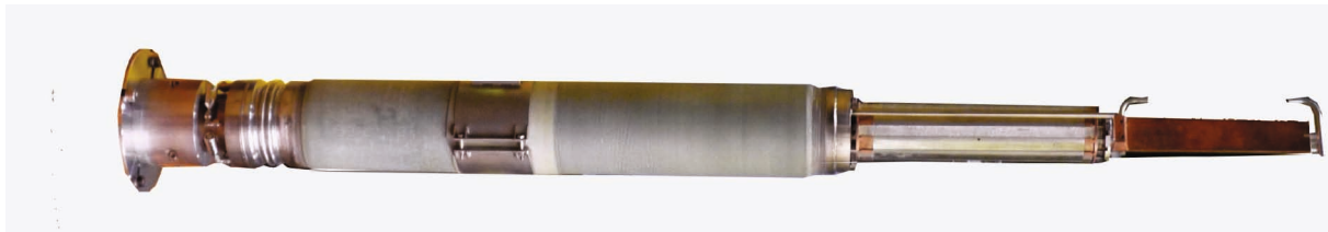
Fig. 3: Mock-up of the W7-X current lead.
