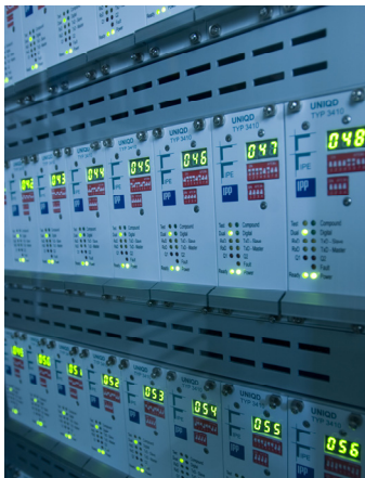
KIT quench detectors UNIQRD (type: 3410) during burn-in
