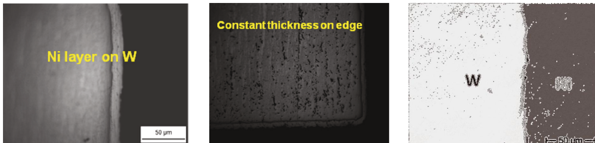
Fig. 4: Nickel layers on tungsten deposited from aqueous electrolyte.
